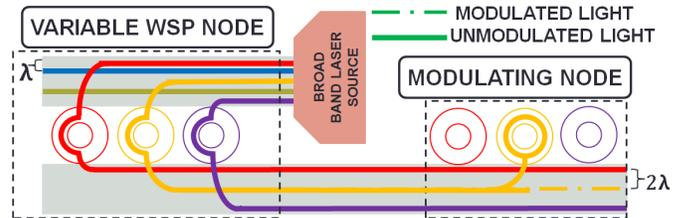
**Fig. 3: WSP technique: variable WSP-node increases wavelength spacing by 100% from λ to 2λ in the bottom data waveguide of the PNoC and the modulating node on the waveguide modulates on available wavelengths.**
