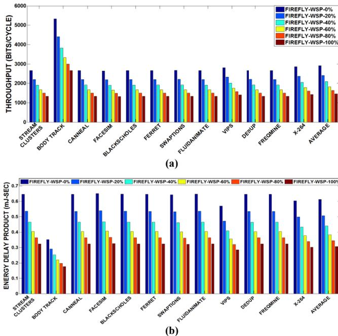
**Fig. 6: (a) Throughput, and (b) energy-delay product (EDP) comparison between Firefly baseline and Firefly configurations with WSP\_20%, WSP\_40%, WSP\_60%, WSP\_80% and WSP\_100%, for PARSEC suite.**
