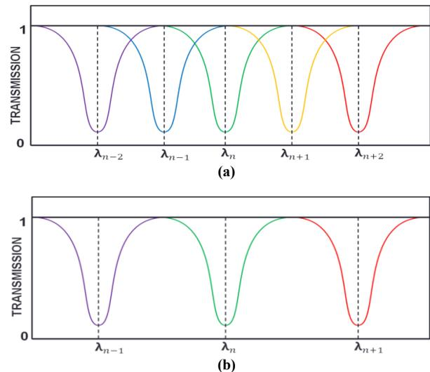
Fig. 1: Transmission spectrum of the cascaded microring modulators when using (a) smaller wavelength spacing (b) larger wavelength spacing.
