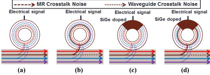
**Fig. 2: MR operation modes: (a) modulator in passing (through) mode (b) modulator in modulating mode (c) detector in passing mode (d) detector in detecting mode**
