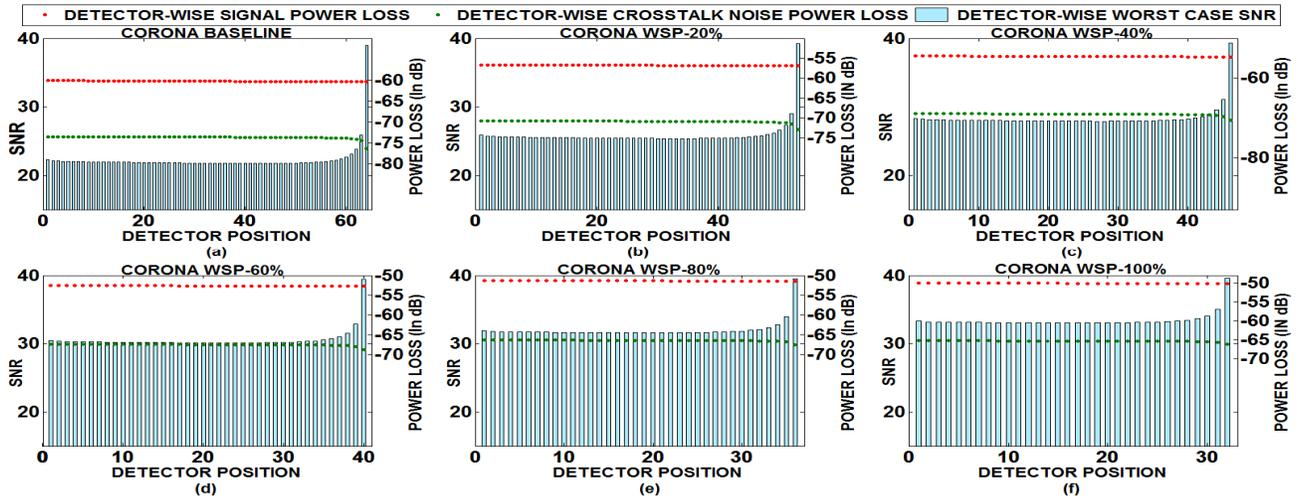
Fig. 4: Detector-wise signal power loss, crosstalk noise power loss and minimum SNR in MPLN for Corona (a) baseline with 64-detectors (b) WSP increased by 20% with 53-detectors (c) WSP increased by 40% with 46-detectors (d) WSP increased by 60% with 40-detectors (e) WSP increased by 80% with 36-detectors (f) WSP increased by 100% (doubled) with 32-detectors.
