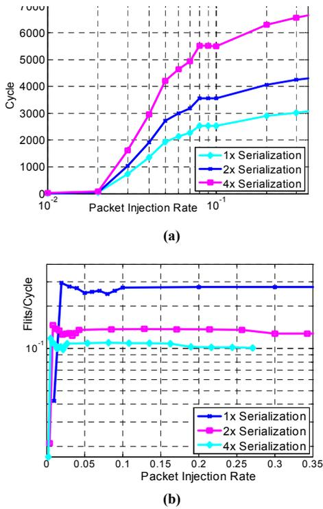
Figure 10. Impact of serialization on (a) average latency, (b) throughput
