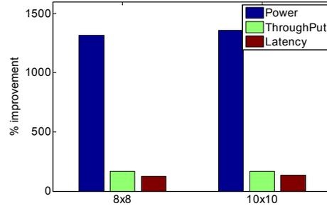
Figure 11. Overall improvement with hybrid photonic NoC
