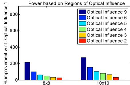
Figure 7. Reduction in power consumption with varying regions of optical influence
