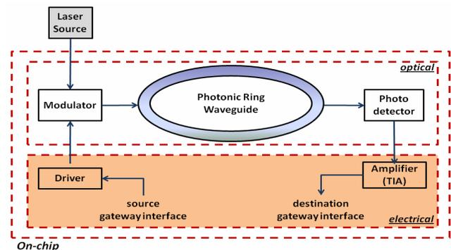
Figure 2. High level overview of photonic transmission architecture
