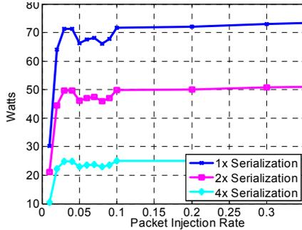
Figure 9. Impact of serialization on power consumption
