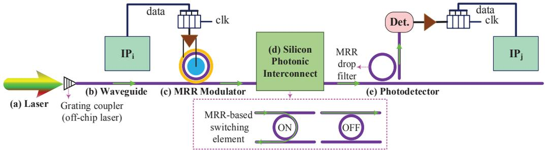
Fig. 2. An abstract overview of a silicon photonic interconnect between two intellectual property (IP) cores ( $IP_i$  and  $IP_j$ ) in a HPC system. As an example, we consider using microring resonators (MRRs) for modulation, switching, and filtering.
