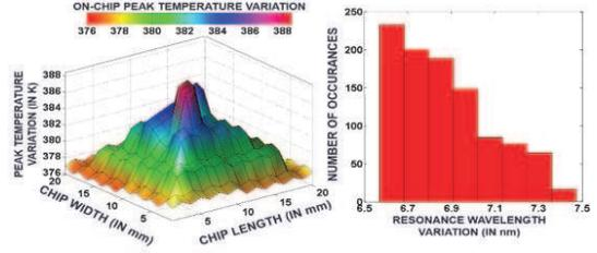
Fig. 4. (a) Spatial variation in peak temperatures; and, (b) Histogram of peak thermal variation-induced resonant wavelength variation across a chip of size  $400 \text{ nm}^2$  using 3D ICE tool while executing 64 threaded PARSEC and SPLASH2 benchmark applications on a 64-core system [15].
