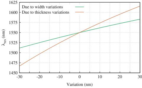
Fig. 3. Resonant wavelength ( $\lambda_{res}$ ) shift in a microring resonator as a result of variations in the waveguide width and thickness (x-axis). As can be seen, the resonant wavelength shifts with any variations in the critical dimensions (width and thickness) of the microring resonator.
