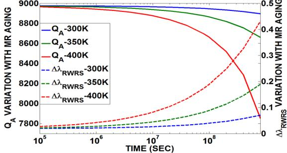
Fig. 3: Variation of resonance wavelength red shift ( $\Delta\lambda_{RWRS}$ ) and  $Q_A$  with time at three operating temperatures 300K, 350K, and 400K.
