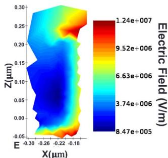
Fig. 2: Distribution of electric field (E) across Si-SiO<sub>2</sub> boundary B<sub>2</sub> when -4V bias voltage is applied across PN junction.
