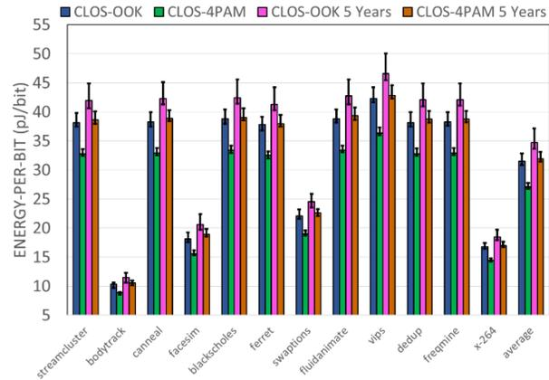
Fig. 11: Energy-per-bit (EPB) comparison of the baseline CLOS-OOK and CLOS-4PAM PNoCs with their variants with 5 Years of VBTI aging considering 100 PV maps across PARSEC benchmarks.
