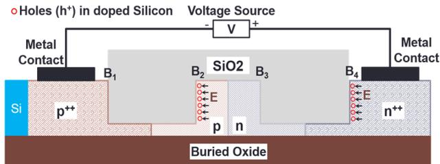
Fig. 1: Cross-section of a tunable MR with PN junction in its core to facilitate carrier injection and depletion with voltage biasing.
