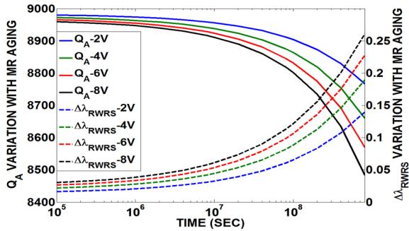
Fig. 4: Variation of  $Q_A$  and resonance wavelength red shift ( $\Delta\lambda_{RWRS}$ ) with operation time at four bias voltages -2V, -4V, -6V, and -8V.
