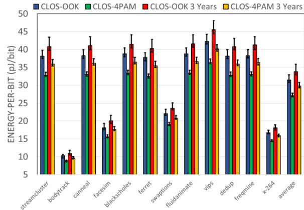
Fig. 10: Energy-per-bit (EPB) comparison of the baseline CLOS-OOK and CLOS-4PAM PNoCs with their variants with 3 Years of VBTI aging considering 100 PV maps across PARSEC benchmarks.
