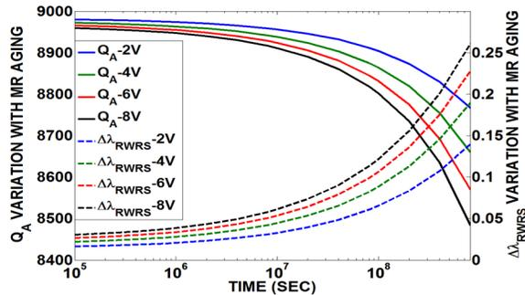
Fig. 4: Variation of  $Q_A$  and resonance wavelength red shift ( $\Delta\lambda_{\text{RWRS}}$ ) with operation time at four bias voltages -2V, -4V, -6V, and -8V.
