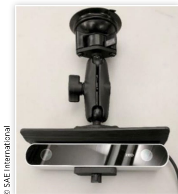
FIGURE 4 ZED stereo vision camera used for video capture
