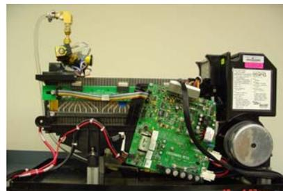
Fig. 2: Ballard NEXA 1.2kW PEM fuel cell system, including hydrogen pressure regulator, air compressor, and control system with sensors. This system was used for the development work in this paper.
