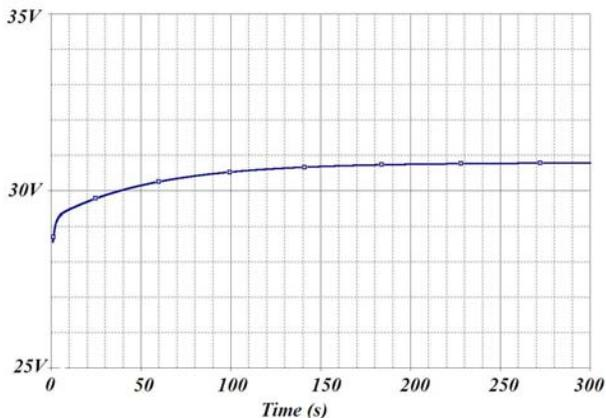
Fig. 11. Full-load step simulation using PSPICE model developed.
