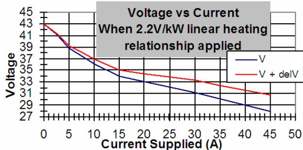
Fig. 8. I-V curve of Ballard Nexa fuel cell. Lower curve is original output voltage curve, taken from [11]. Upper curve is output voltage with the static subsystem in effect.
