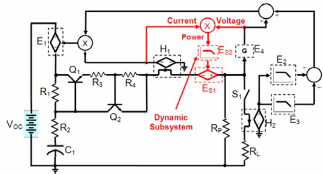
Fig. 9. Fuel cell model with dynamic subsystem modification added.
