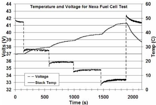
Fig. 12. Experimental test results for 4 load steps performed on Ballard fuel cell system.
