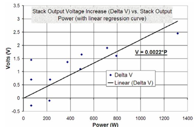
Fig. 6. Stack output voltage change for a given load condition. This general relationship is the basis for the power based model.
