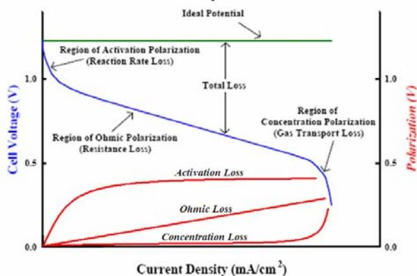
Fig. 3. Typical fuel cell polarization, or I-V, curve. Ideal potential (top) is reduced by three polarization regions (bottom three curves), to the commonly seen result (second from top).
