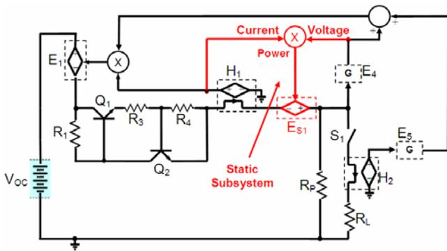
Fig. 7. Fuel cell model with static modification subsystem added.
