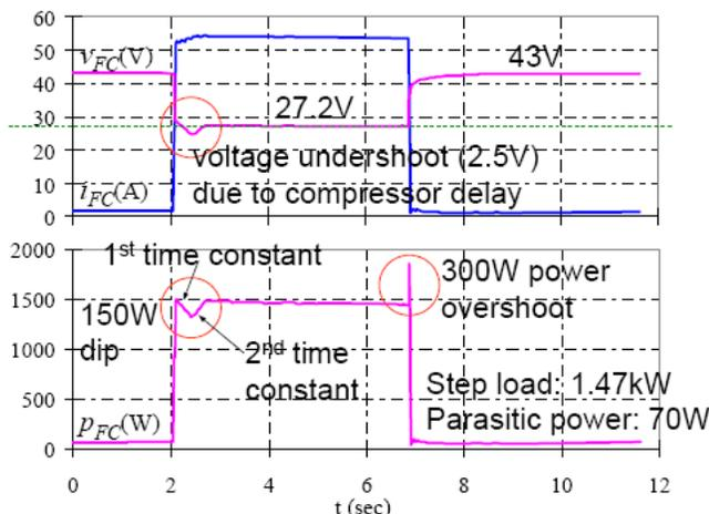
Fig. 4. Short time-period fuel cell dynamic showing no- to full-load step. Transient points of interest are circled on voltage and power curves.
