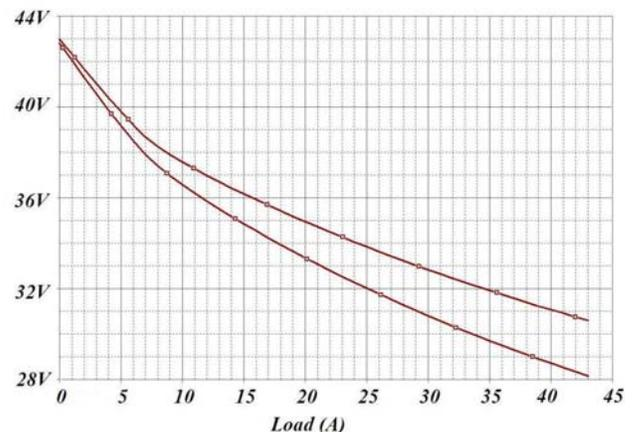
Fig. 10. I-V curve from simulation of PSPICE model set up for Ballard fuel cell system. Upper curve represents electrical model with proposed modification in effect, and lower curve without. The lower curve closely matches that found in [11] for the Ballard system.
