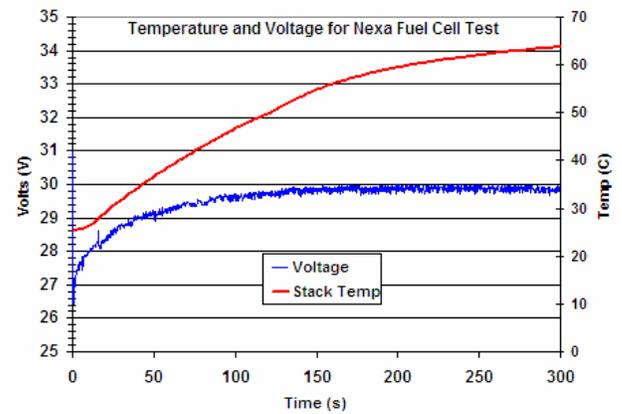
Fig. 5. Temperature (upper curve) and voltage (lower curve) data for a full-load step transient, showing long time-constant rises in both. This gave motivation to improve fuel cell models that do not incorporate these long time transients.
