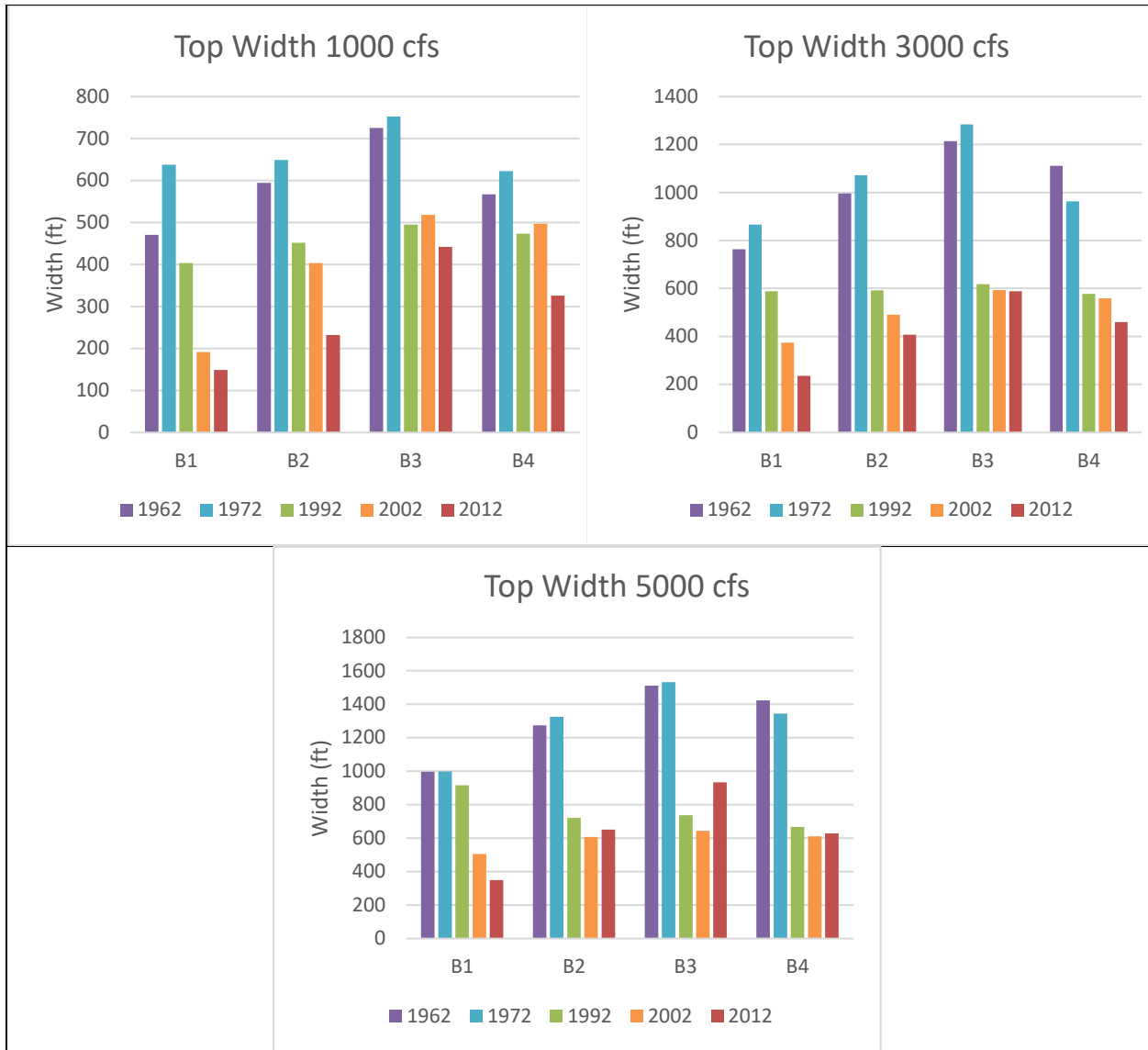
Figure 3-16 HEC-RAS Wetted top width of channel at 1,000 cfs (top left), 3,000 cfs (top right), and 5,000 cfs (bottom middle)
