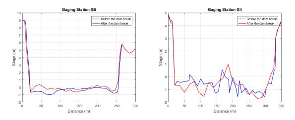
Figure 3.10 – Cross section survey in the Doce River at stations G5 and G4
