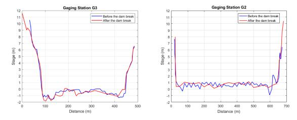
Figure 3.11 – Cross section survey in the Doce River at stations G3 and G2
