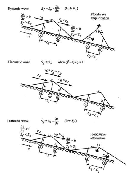
Figure 2.4 – Propagation of dynamic, kinematic and diffusive waves (Julien, 2018)
