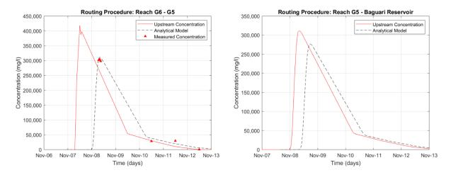
Figure 4.5 - Routing procedure result in the reaches: G6-G5 and G5-Baguari Reservoir
