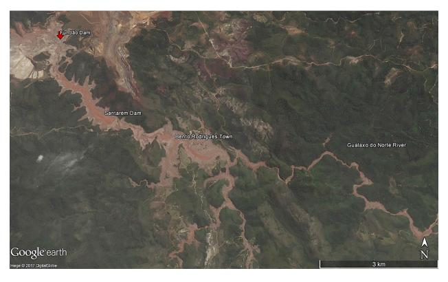
Figure 4.3 – Fundão Dam site after the collapse (Google, 2015)
