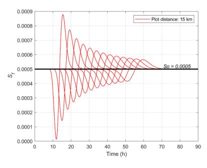
Figure 5.11 – Variation of energy slope during the numerical simulation (Reach A)
