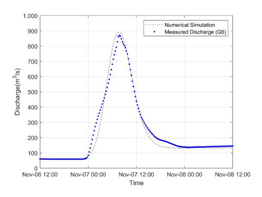
Figure 5.6 – Application of the new hydraulic diffusivity coefficient on the Doce River reach using the Crank Nicolson scheme (Candonga Dam – G6)
