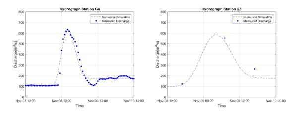
Figure 5.12 - Hydrograph at station G4 and G3
