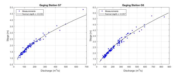
Figure 3.12 - Stage-discharge curves at stations G7 and G6
