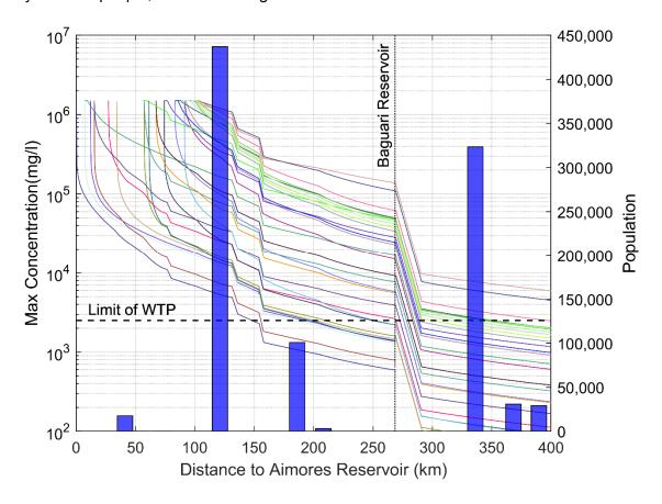
Figure 7.5 – Propagation of the high sediment concentration due the collapse of tailings dams in the Doce River basin
