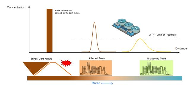
Figure 7.3 – Sketch of the sediment propagation after a hypothetical tailings dam failure
