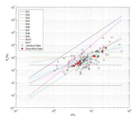
Figure 4.11 – Comparison between the longitudinal dispersion coefficients presented in the literature and the Doce Rive data with *W/h* =66.
