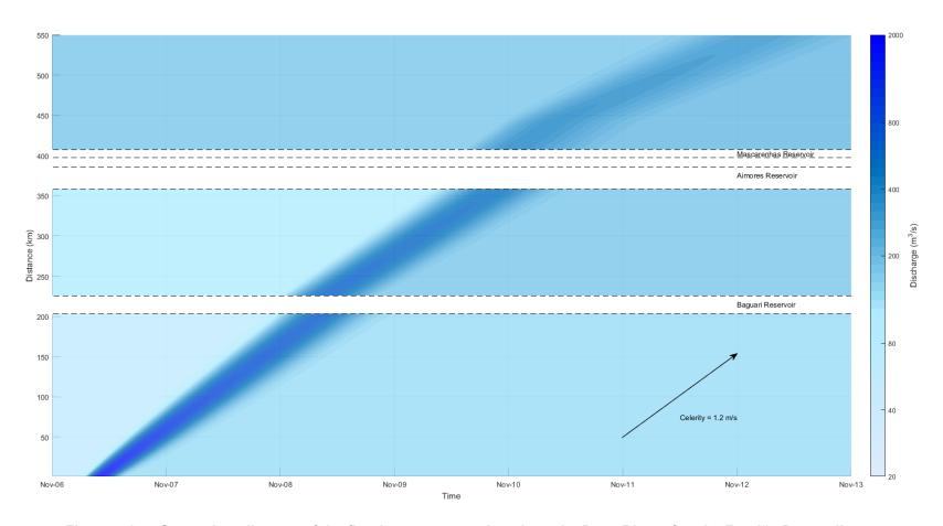
Figure 5.15 – Space time diagram of the floodwave propagation along the Doce River after the Fundão Dam collapse
