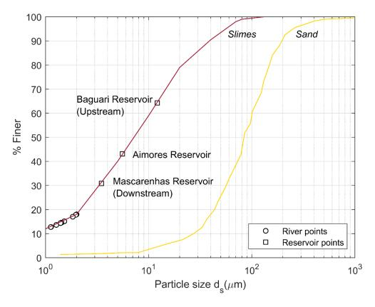
Figure 4.13 – Comparison of the particle size distribution of the material stored in the Fundão Dam reservoir and the particle size related with the settling rate observed in the Doce River and in the reservoirs
