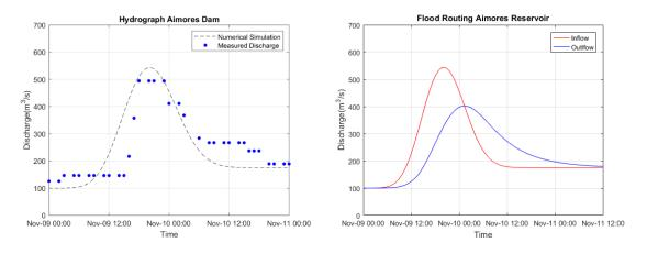
Figure 5.13 – Hydrograph and flood routing at Aimorés Dam
