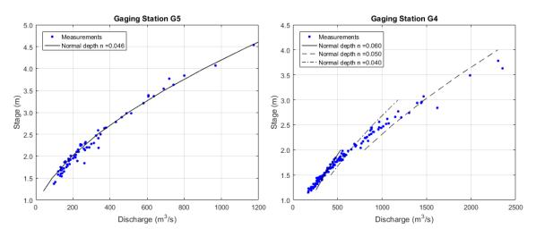
Figure 3.13 - Stage-discharge curves at stations G5 and G4
