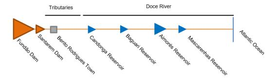
Figure 1.2 – Sketch of floodwave propagation along the Doce River basin
