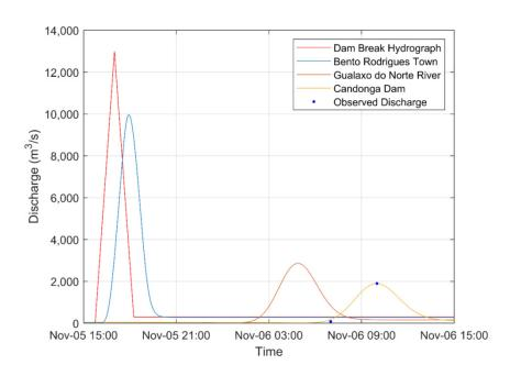
Figure 5.3 - Floodwave simulation at the Upper Reach
