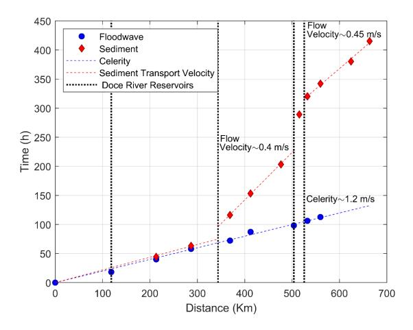
Figure 4.16 - Comparison between the floodwave celerity and sediment velocity in Doce River
