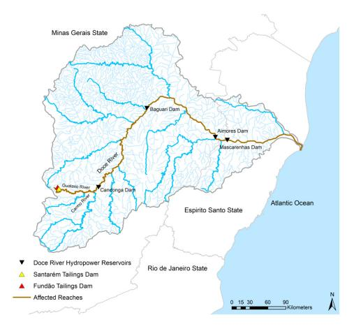
Figure 3.7 – Fundão Dam location and the mud flood path
