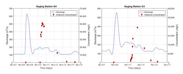
Figure 3.20 - Hydrograph and suspended sediment concentration at gaging stations G4 and G3
