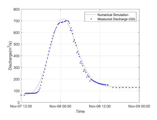
Figure 5.8 – Application of the new hydraulic diffusivity coefficient on the Doce River reach using the Crank Nicolson scheme (G6 – G5)
