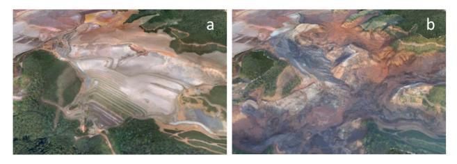
Figure 3.6 – Fundão Dam before (a) and after failure (b) (Morgenstern et al., 2016)
