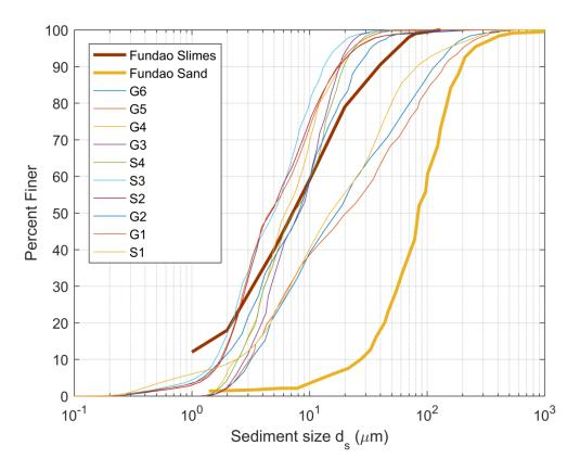
Figure 3.22 – Particle size distribution of the Fundão Dam impounded material and observed along the Doce River
