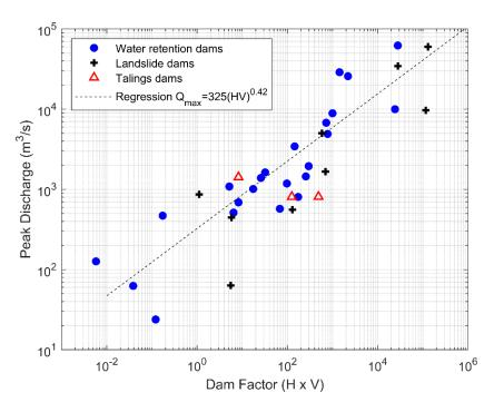
Figure 2.3 - Relationship between peak discharge and dam factor (Rico et al., 2008)
