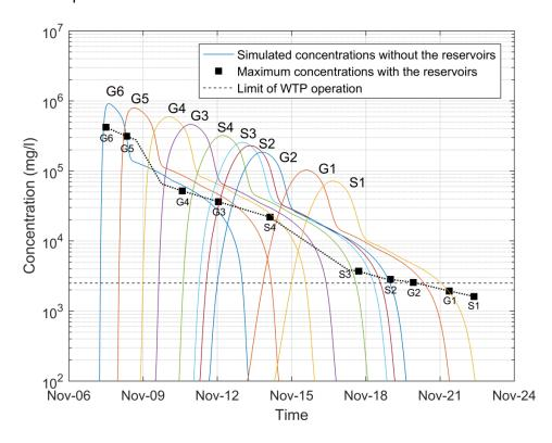
Figure 6.7 – Suspended sediment simulation considering the hypothesis of inexistence of the Doce River hydropower reservoirs
