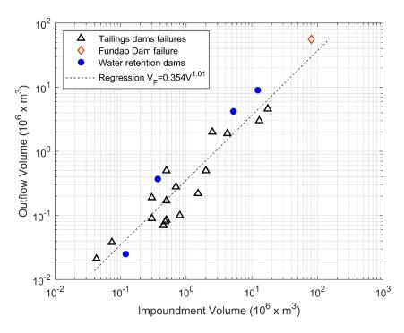
Figure 2.2 – Relationship between Impoundment Volume and Outflow volume (Rico et al., 2008)
