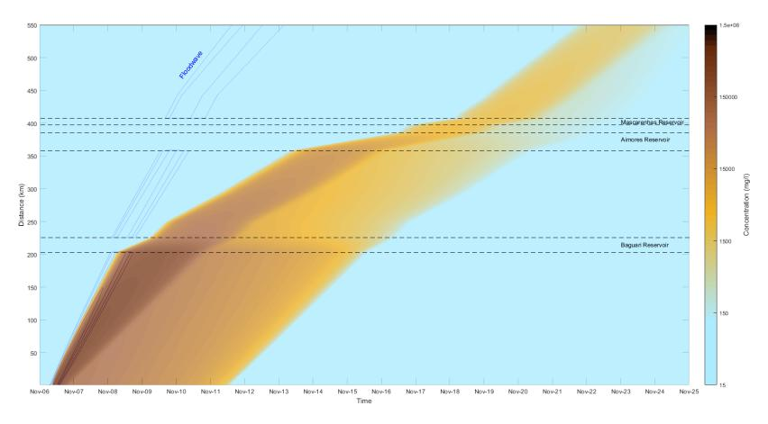
Figure 6.5 – Space time diagram of the sediment concentration and floodwave propagation along the Doce River after the Fundão Dam collapse
