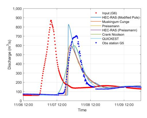
Figure 5.5 – Test of flood routing procedures, Reach A downstream (G6 – G5)
