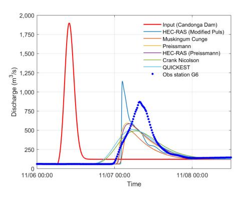
Figure 5.4 – Test of flood routing procedures, Reach A upstream (Candonga Dam – G6)
