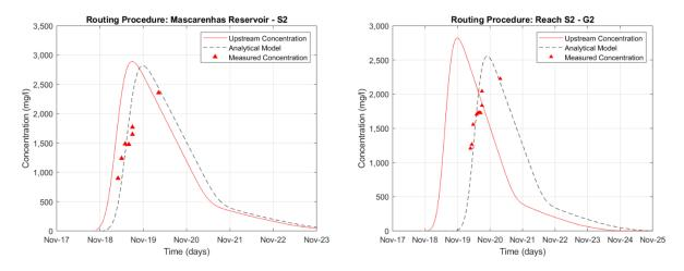
Figure 4.8 – Routing procedure result in the reaches: Mascarenhas reservoir-S2 and S2-G2
