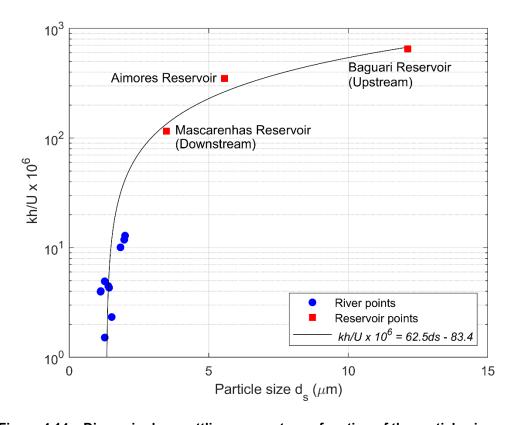
Figure 4.14 – Dimensionless settling parameter as function of the particle size
