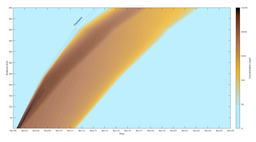
Figure 6.9 – Space time diagram of the suspended sediment propagation and the floodwave assuming the hypothesis of inexistence of the reservoirs
