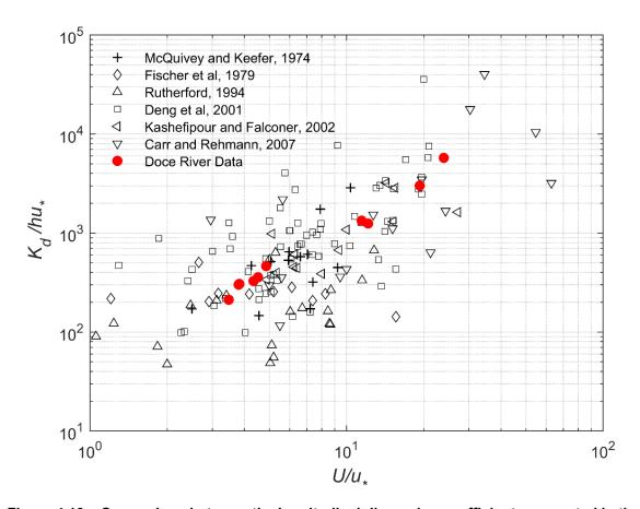
Figure 4.10 – Comparison between the longitudinal dispersion coefficients presented in the literature and the Doce Rive data (McQuivey & Keefer, 1974; Fischer et al., 1979; Rutherford, 1994; Deng, Singh, & Bengtsson, 2001; Kashefipour & Falconer, 2002; Carr & Rehmann, 2007).
