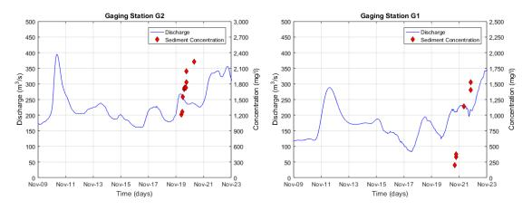
Figure 3.21 - Hydrograph and suspended sediment concentration at gaging stations G2 and G1
