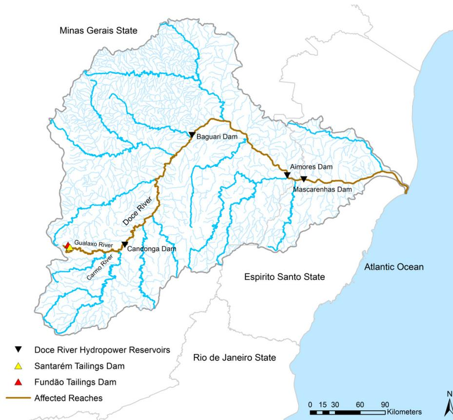
**Figure 3.7 – Fundão Dam location and the mud flood path**
