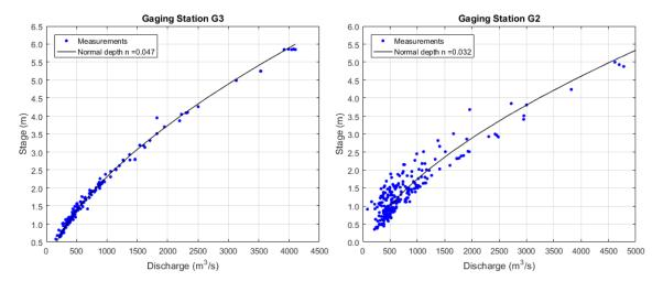
Figure 3.14 - Stage-discharge curves at stations G3 and G2
