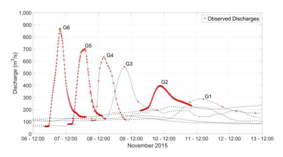
Figure 3.17 - Observed hydrographs after the Fundão Dam failure
