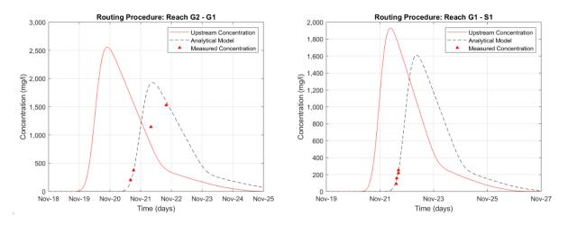
Figure 4.9 - Routing procedure result in the reaches: G2-G1 and G1-S1
