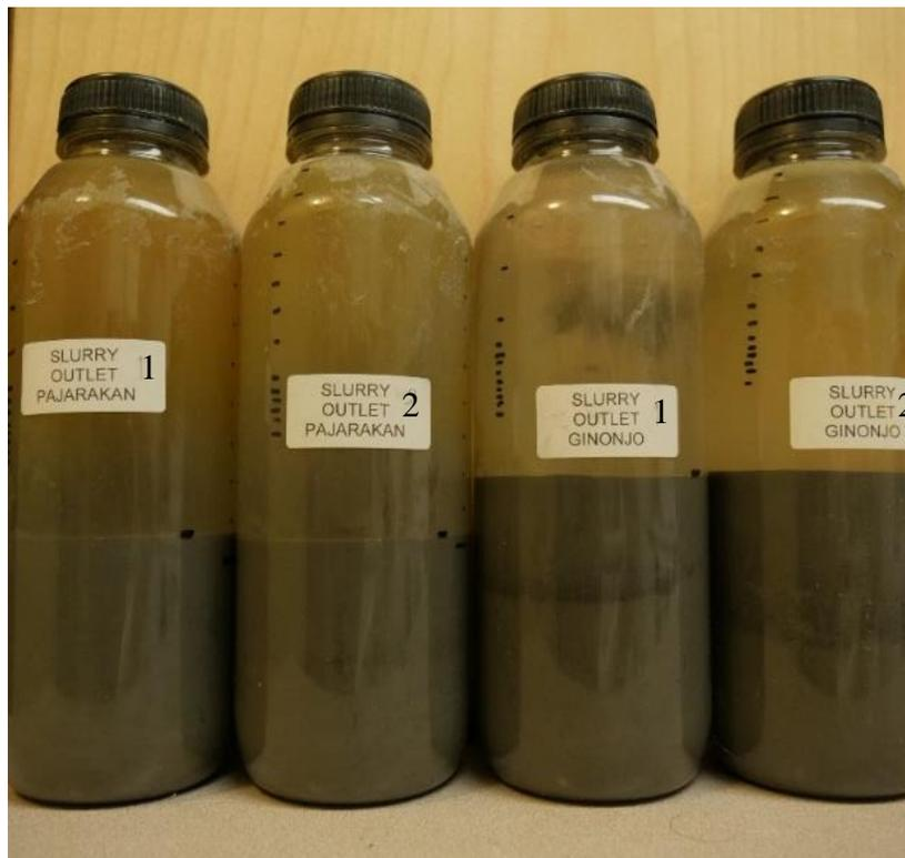
*Figure 32* Samples from Pejarakan and Ginonjo Outlet. Sample from left: P1, P2, G1 and G2; deflocculant were added to P2 and G2.
