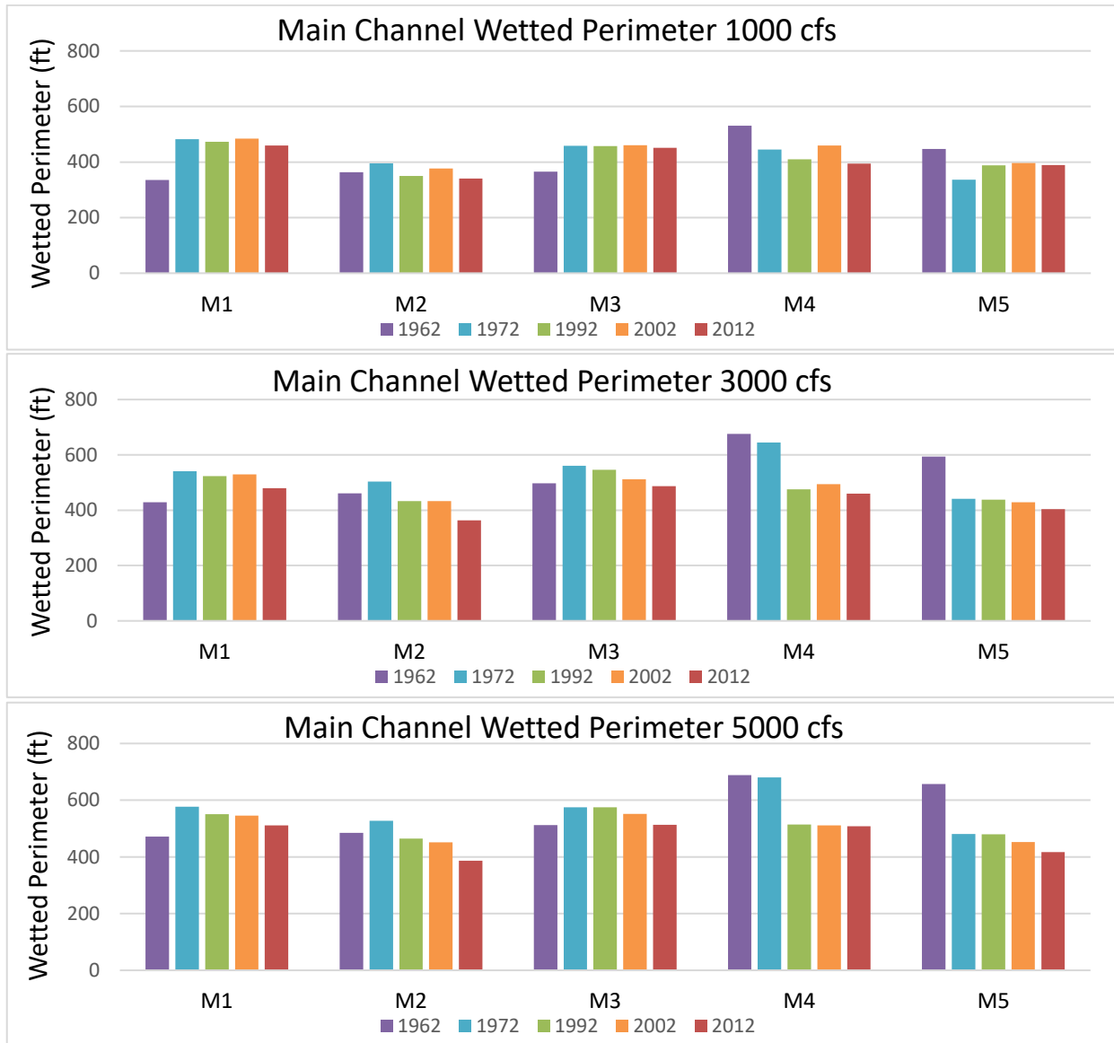
Figure 3-16 HEC-RAS main channel wetted perimeter at 1,000 cfs (top), 3,000 cfs (middle), 5,000 cfs (bottom).
