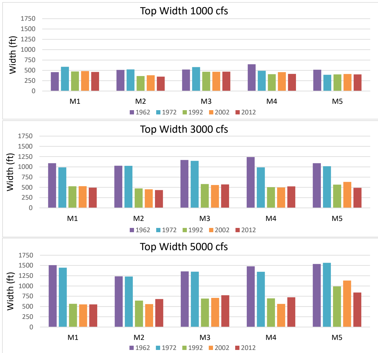
Figure 3-14 HEC-RAS wetted top width of Montañó Subreaches at 1,000 cfs (top), 3,000 cfs (middle), and 5,000 cfs (bottom).
