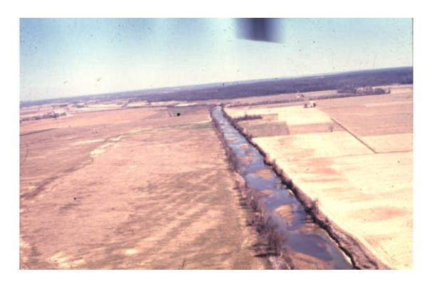
Figure 2.8 Typical Alternate Bar Pattern
