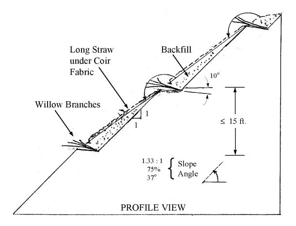
**Figure 41.** Brush layering with coir woven fabric and long straw under fabric. Coir fabric and straw help control rillying and gullying between layers. (Adapted from Gray and Leiser, 1982)
