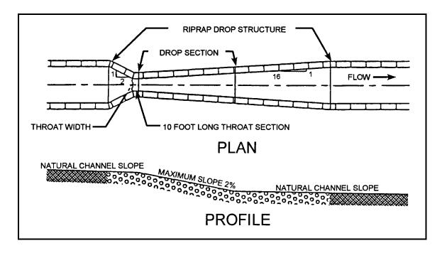
Figure 12.13 Riprap Lined Drop Structures (adapted from Tate, 1991)
