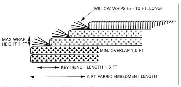
**Figure 31.** Cross-section of Vegetative Geogrid, also called Fabric-Encapsulated Soil with vegetation. (adapted from Miller, 1992)
