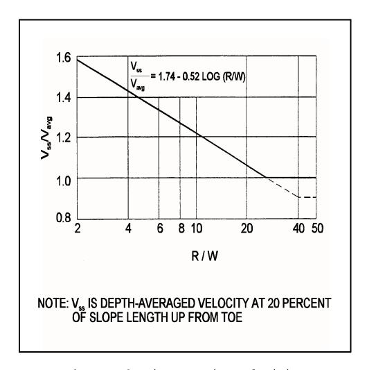
Figure A.2a Riprap Design Velocities
