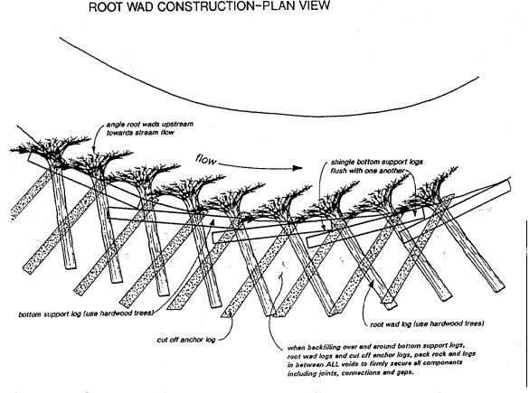
**Figure 17.** Schematic of root wad construction (from Bowers, 1992).
