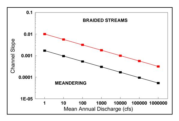
Figure 2.10 Lane's (1957) Relationship Between Channel Patterns, Channel Gradient, and Mean Discharge
