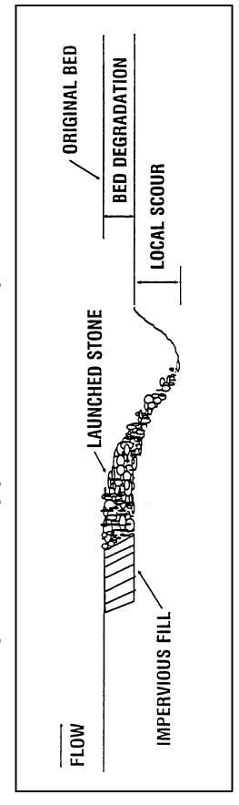
Figures 12.5b Launching of Riprap at Grade Control Structure in Response to Bed Degradation and Local Scour
