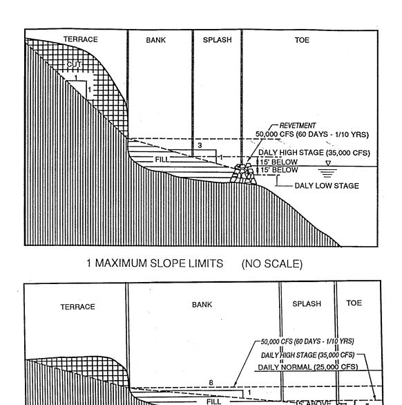
2 MINIMUM SLOPE LIMITS (NO SCALE)
