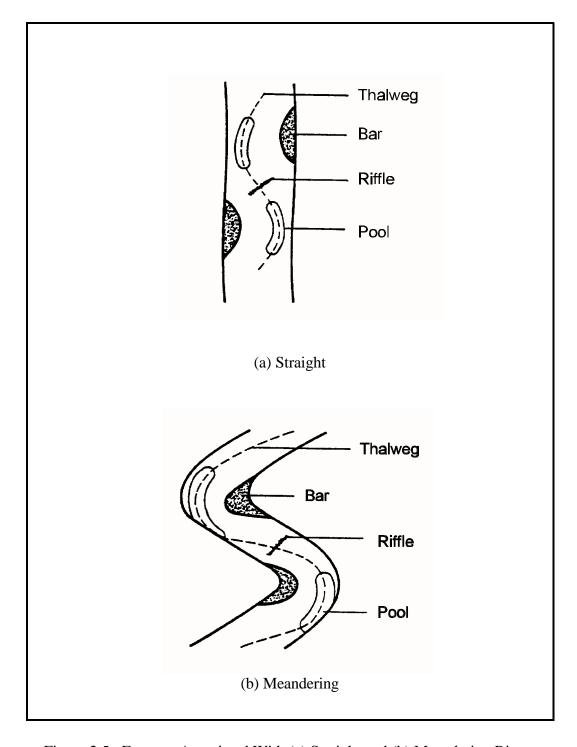
Figure 2.5 Features Associated With (a) Straight and (b) Meandering Rivers
