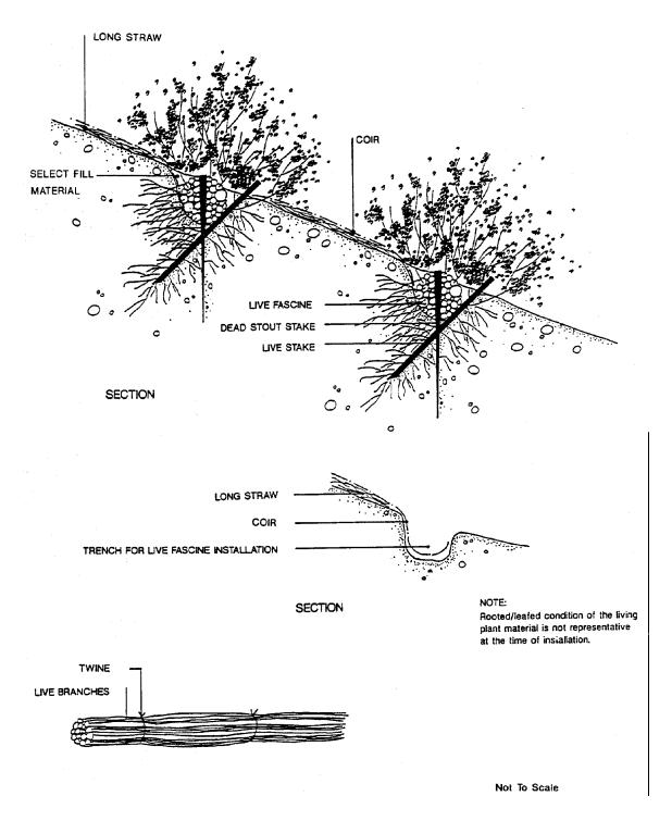
**Figure 40.** Schematic illustration of live fascine bundles with coir rope mesh fabric and long straw installed between the bundles. (from US Army Corps of Engineers, Nashville, 1993; schematic drawn by Robin B. Sotir & Associates, 1993)
