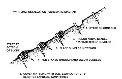
**Figure 39b**. Procedures for installing wattling bundles on slope in the bank zone. (from Leiser, 1983)
