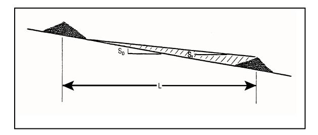
Figure 12.1 Spacing of Grade Control Structure (adapted from Mussetter, 1982)
