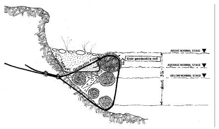
**Figure 19.** Schematic of log revetment with coir geotextile roll and plantings on top of backfill soil over a geotextile filter. (Designed by Alan Czenkusch, Colo. Division of Wildlife)
