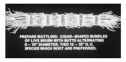
**Figure 39a**. Schematic of wattling bundle with preparation specifications. (from Leiser, 1983)
