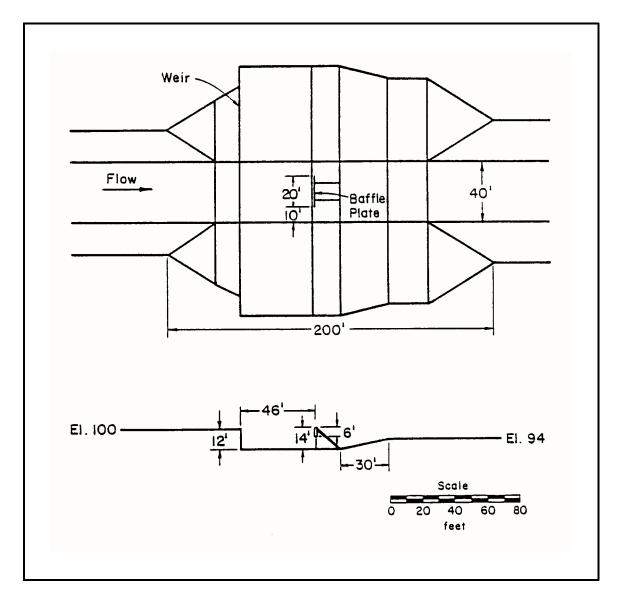
Figure 12.10 Schematic of Modified ARS-Type Grade Control Structure (Abt et al., 1994)
