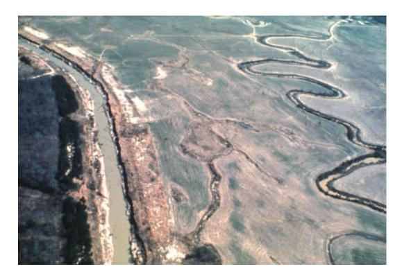
Figure 2.16 Channelized Stream and Abandoned Old Channel
