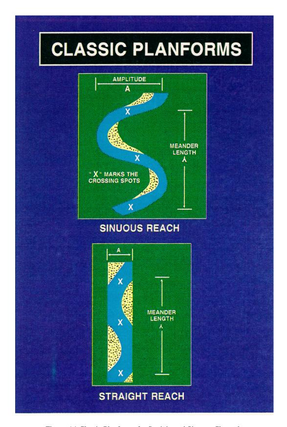
Figure 6.1 Classic Planforms for Straight and Sinuous Channels
