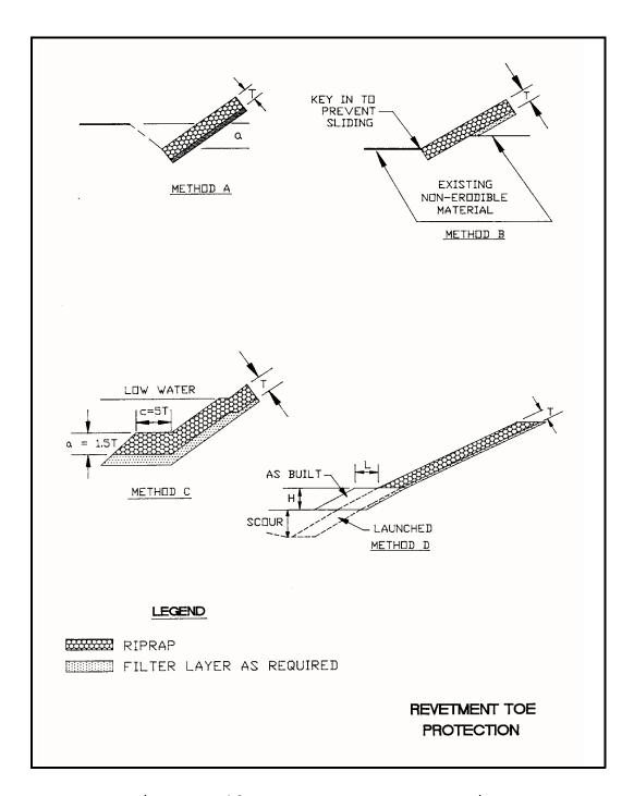
Figure A.10 Revetment Toe Protection
