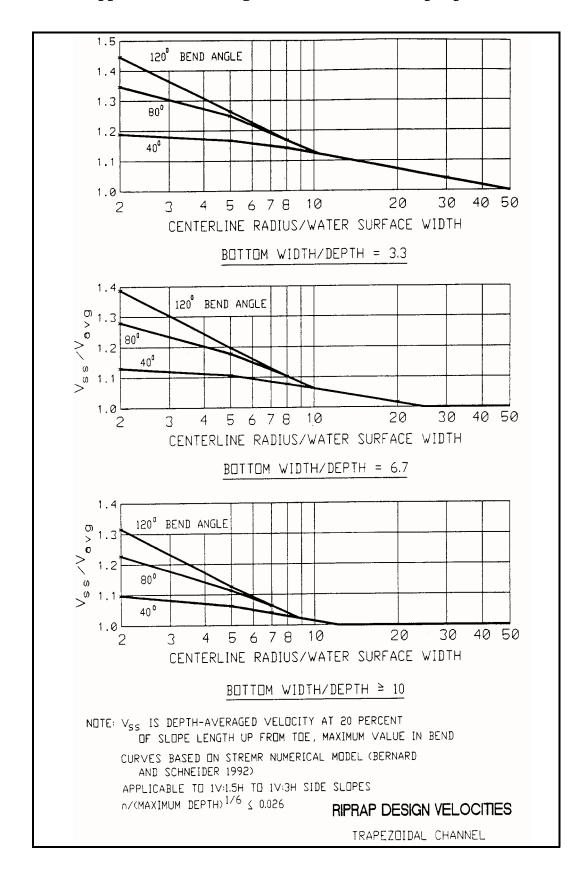
Figure A.2b Riprap Design Velocities
