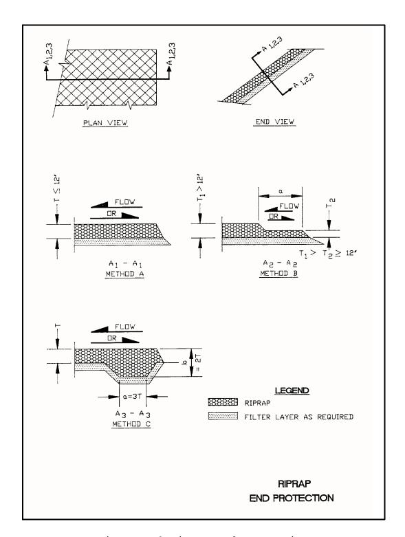
Figure A.9 Riprap End Protection
