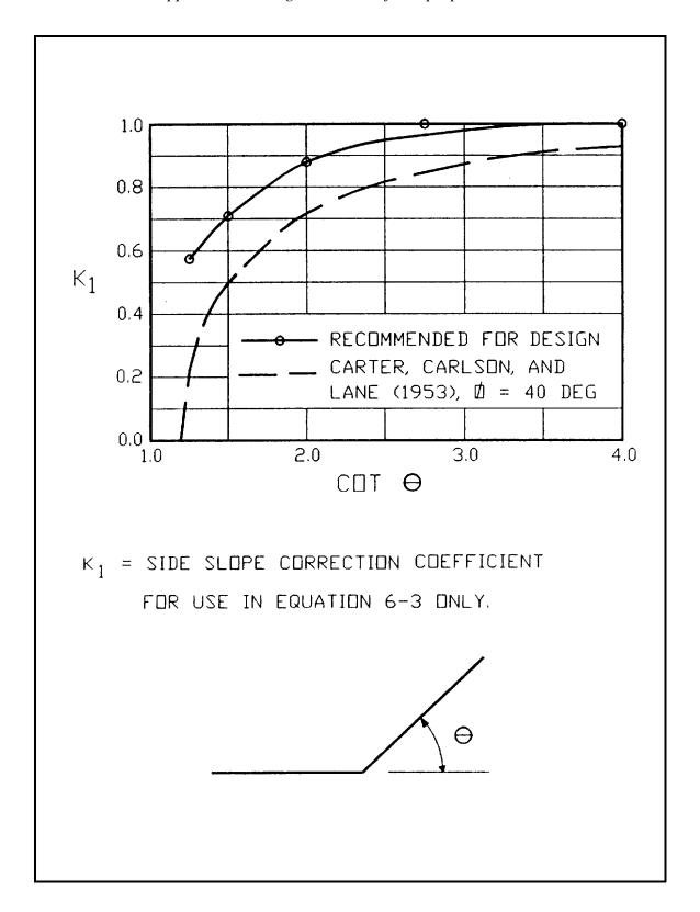
Figure A.7 Correction for Side Slope Angle
