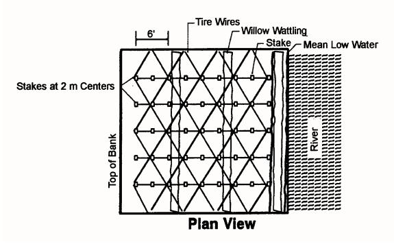
**Figure 7.** Schematics of bioengineering treatment used with a weighted rock toe with vegetation in the form of a brush mattress (to be discussed later) used above it.
