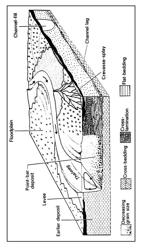
Figure 2.2 Landforms for a Meandering River (Collinson, 1978 after Allen, 1970)
