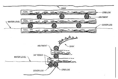
**Figure 15.** Bank crib with cover log used to protect unstable streambanks while concurrently providing excellent overhead cover for fish. (Courtesy of US Forest Service)
