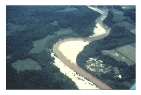
Figure 2.3 Typical Meandering River
