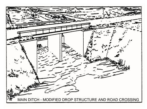
Figure 12.2 Combination Grade Control Structure and Road Crossing (adapted from U.S. Soil Conservation Service, 1976)
