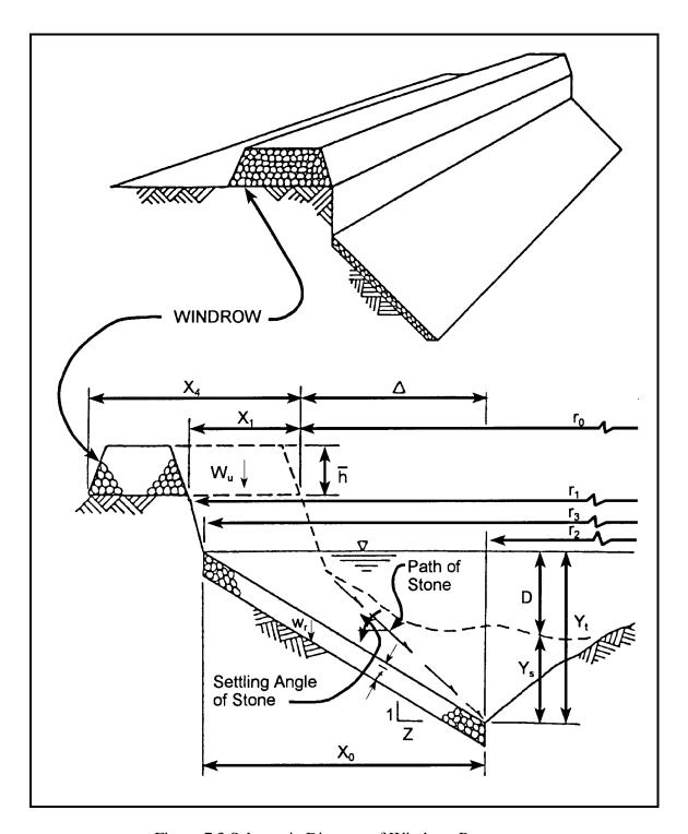
Figure 7.3 Schematic Diagram of Windrow Revetment
