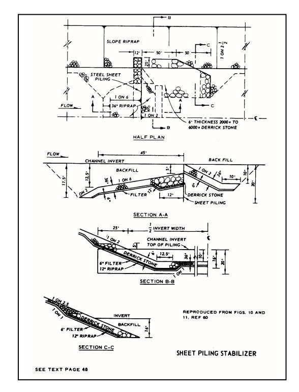
Figure 12.8 Bed Stabilizer Design with Sheet Pile Cutoff (U.S. Army Corps of Engineers, 1970)
