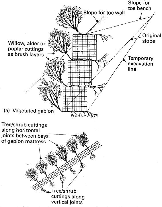
**Figure 13.** Schematic of gabions used with woody plants to form a hard structure to prevent undercutting and flanking. Can be used in the toe zone or installed higher in the splash and bank zones. (from Coppin and Richards, 1990)
