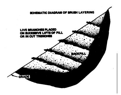
**Figure 28.** Schematic diagram of brush layering. (from Leiser, 1983)
