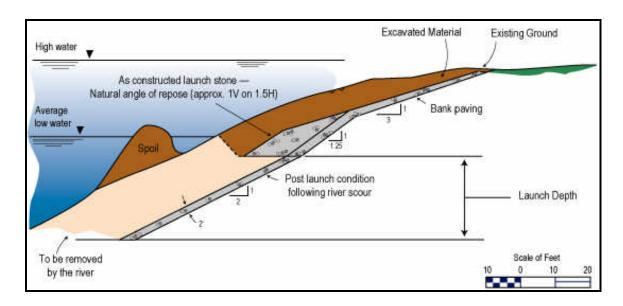
Figure 7.1 Typical Cross Section of a Trenchfill Revetment
