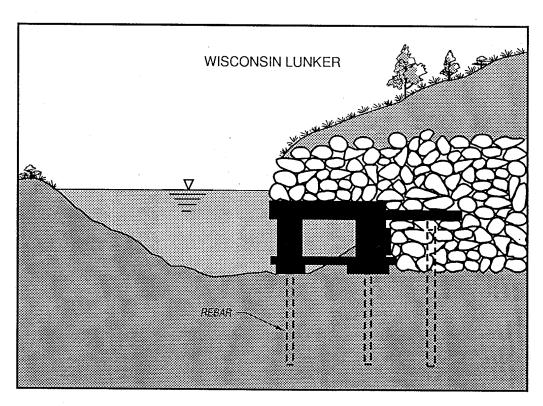
**Figure 14.** Two schematics (two different versions) of a LUNKERS structure designed to provide overhanging shade and protection for fish while serving to stabilize the toe of a streambank. Both versions use rebar although rebar is not shown on the upper schematic.
