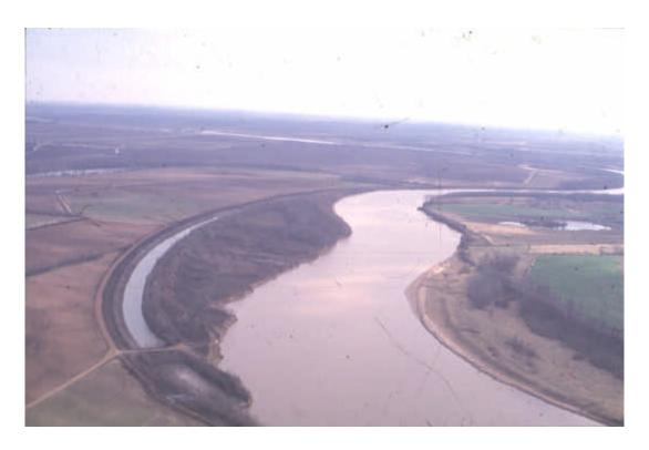
Figure 7.2 Aerial View of Trenchfill Revetment With Foreshore Material Still in Place
