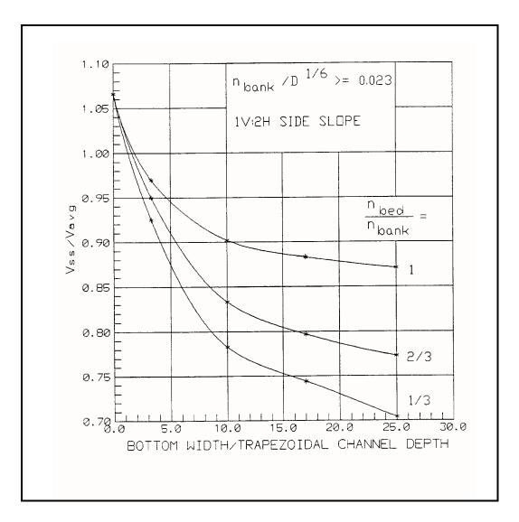
Figure A.3  $V_{\rm ss}/V_{\rm avg}$  for Straight Channels Sufficiently Far From (>5w-10w) Upstream Bends
