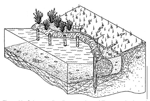
**Figure 23.** Coir geotextile rolls are used to stabilize streambanks and permit planting of wetland vegetation within them. The coconut fiber accumulates sediment and biodegrades as plant roots develop and become a stabilizing system. (From Bestmann Ingenieurbiologie, Wedel, Germany)
