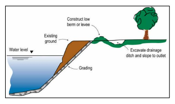
Figure 6.5 Construction of Berm or Levee to Control Overbank Drainage
