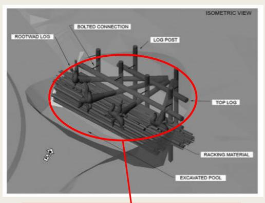
Structure is rootwads stabilized by cross-logs and bolted in place. Aggregate at downstream end for additional stability/ability for vegetation to be established
