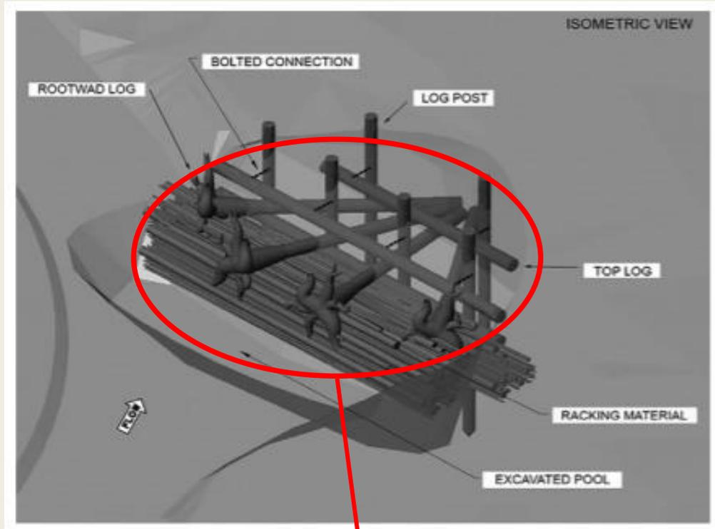
Stability provided by posts anchored to 12 ft below the bed
