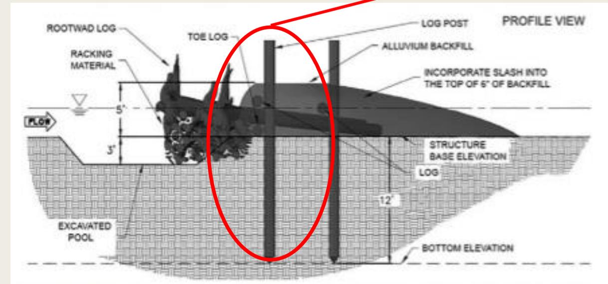
Structure is rootwads stabilized by cross-logs and bolted in place. Aggregate at downstream end for additional stability/ability for vegetation to be established
