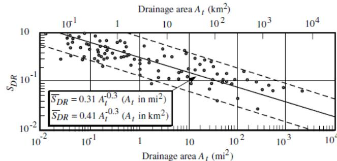
Figure 3.28. Sediment–delivery ratio (modified after Boyce, 1975).
