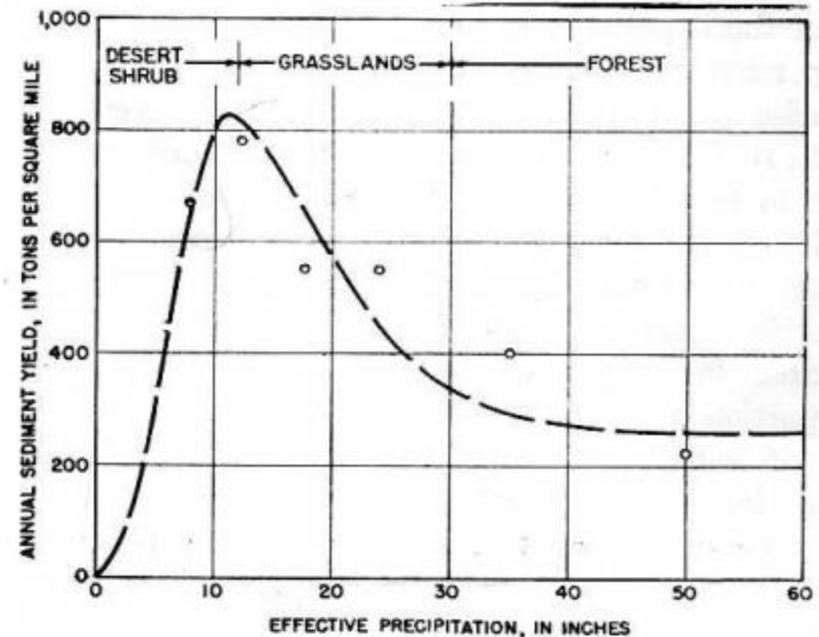
FIG. 2 – Climatic variation of yield of sediment as determined from records at sediment stations
