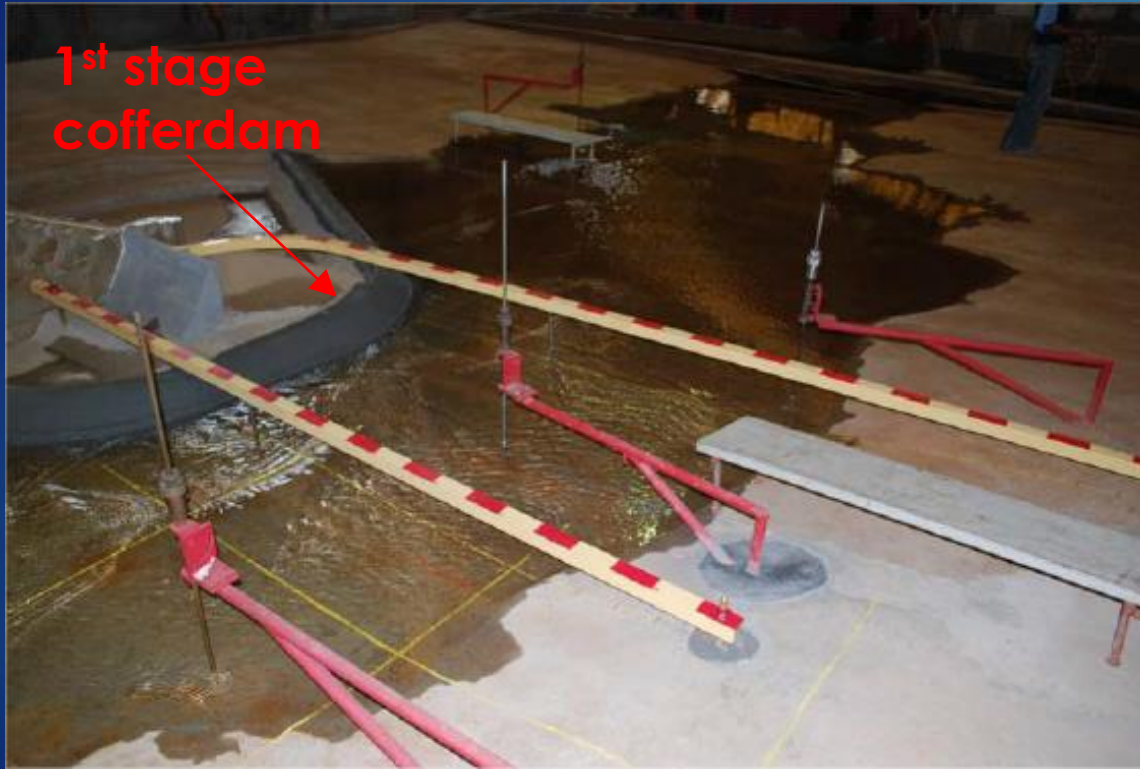
Physical model of 1 st stage of Ijuí River diversion Geometric scale 1:75
