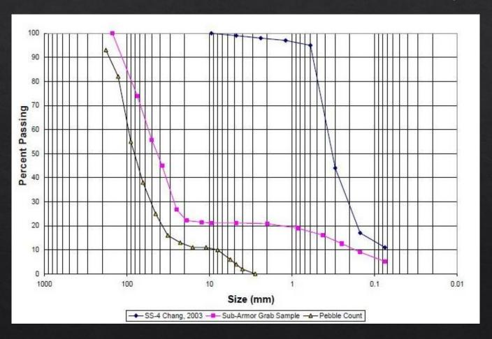
Particle size distributions showing coarsening over time (Engineering and Hydrosystems 2009)
