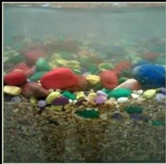
Armor layer in flume experiment. Coarse layer on surface clearly visible with fine grained substrate below.
