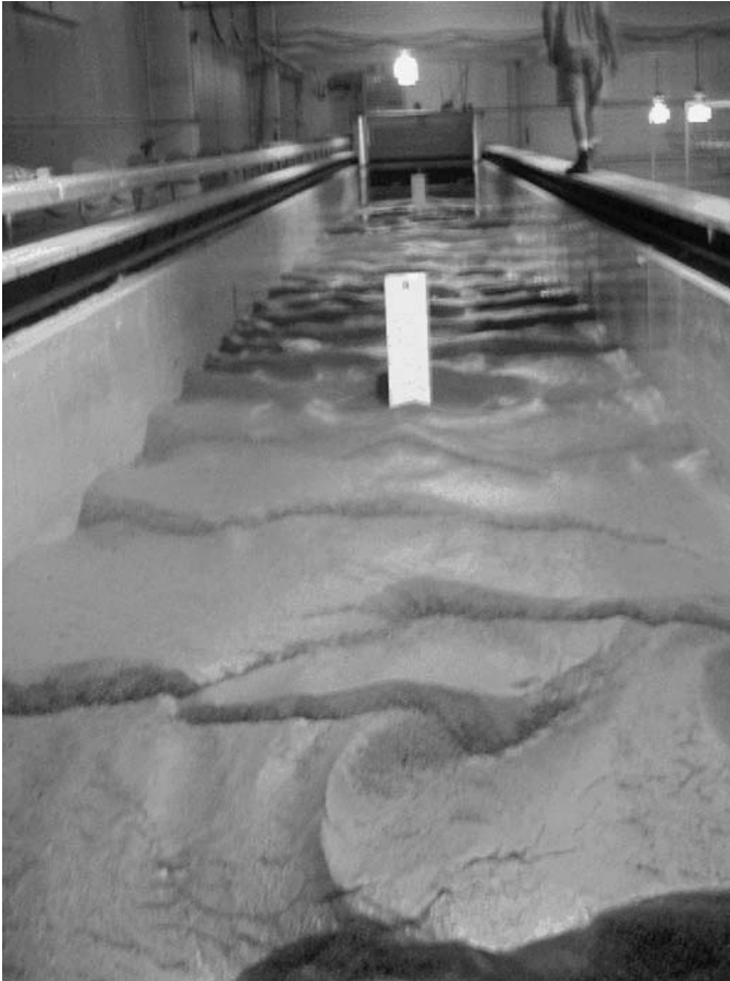
Figure 3.44. Square (8-in) piers in the 8-ft wide, indoor flume (looking upstream) used for NCHRP Project 24-07(2).
