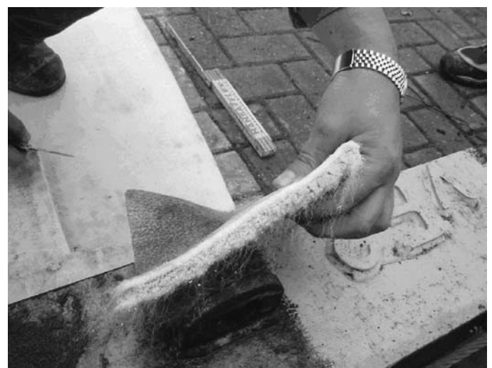
Figure 3.18. Close-up photo of SandMat™ geocomposite blanket, NCHRP Project 24-07(2).
