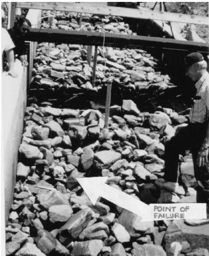
Figure 3.66. Riprap failure in 1994 tests ( d_{50} = 15.2 in [386 mm]).
