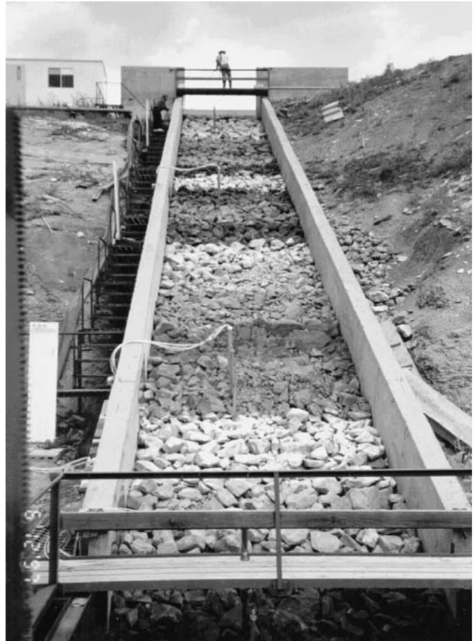
Figure 3.52. Test set up for 1997 ( d_{50} = 10.7 in [271 mm]).
