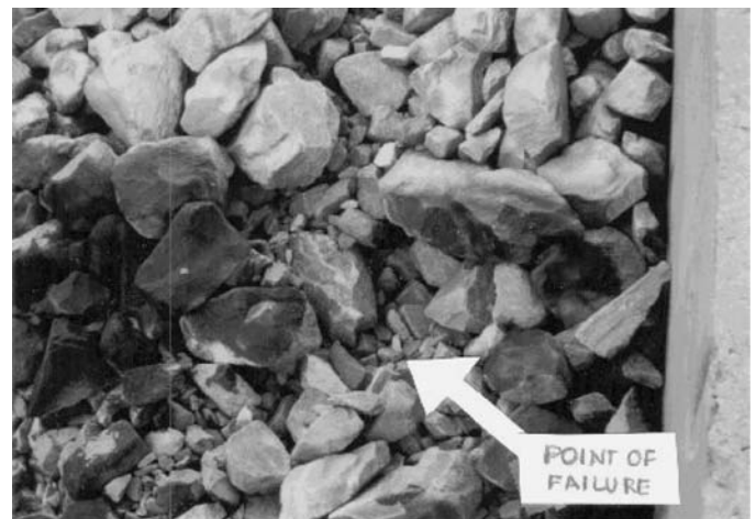
Figure 3.67. Riprap failure in 1997 tests ( d_{50} = 10.7 in [271 mm]).
