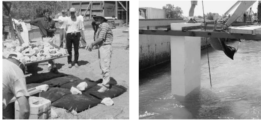
a. Demonstrating puncture resistance of geocontainers
