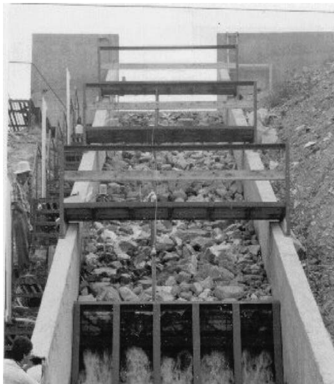
Figure 3.51. Test set up for 1994 ( d_{50} = 15.2 in [386 mm]).
