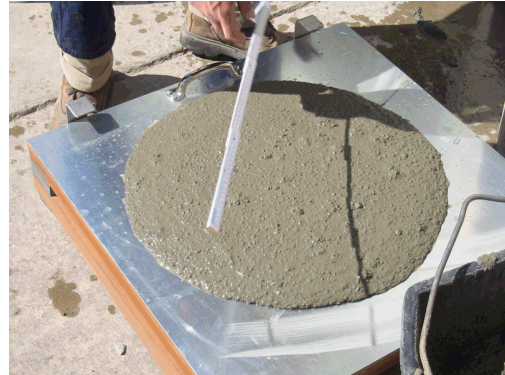
b. Measuring grout slump diameter
