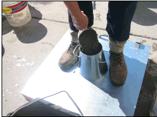
a. Slump cone and test table
