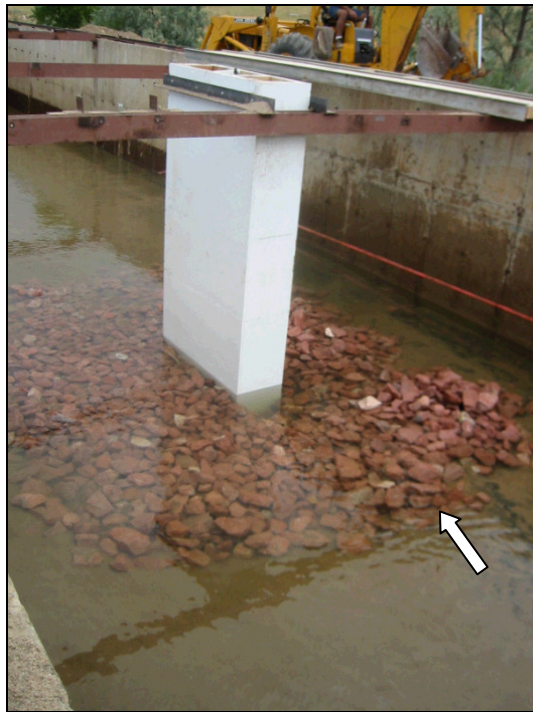
Figure 11.14. Riprap armor over geotextile containers.
