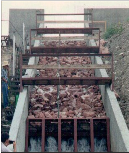
Figure 5.3. Test set up for 1994, d_{50} = 1.27 ft (386 mm).
