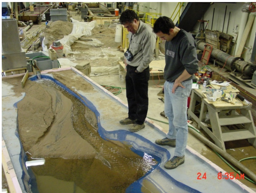
Figure 29.—Gordon Grant (left) inspects the physical model constructed by Chris Bromley (right) at the Saint Anthony Falls Laboratory, MN of Lake Mills behind Glines Canyon Dam to investigate reservoir sediment erosion processes.
