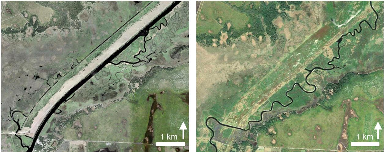
**Figure 13.—Channelized reach of Kissimmee River (left) [77], and restored reach with meandering planform and channelized Reach Filled (Right) [78].**
