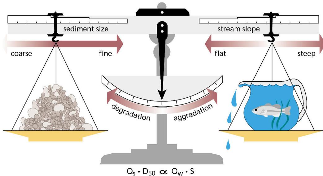
**Figure 1.—Lane's channel stability balance describes how changes in sediment load, size, stream slope, discharge, and channel roughness determine whether a channel will aggrade or incise [7].**
