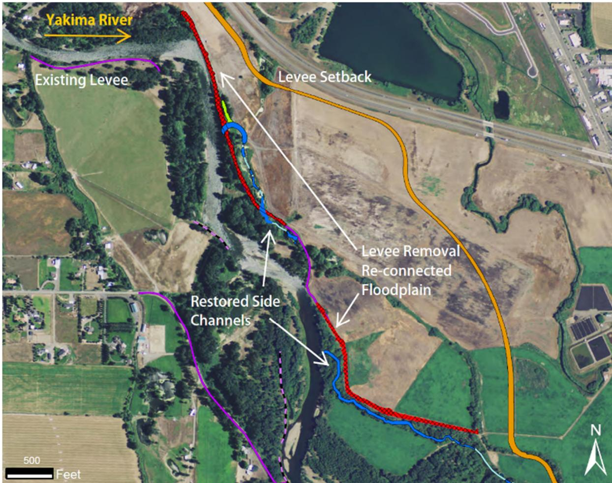
**Figure 10.—An example of a proposed levee setback and side-channel rehabilitation project on the Yakima River, Washington. Hydrologic connection restored to western floodplain. Map courtesy of Robert Hilldale, Bureau of Reclamation. Setback alignment still under discussion.**
