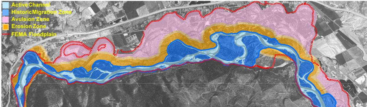
**Figure 4.—Example of a channel migration zone study depicting the active channel (light blue), historic channel migration zone (dark blue), future erosion buffer (orange), potential channel avulsion zone (pink), and regulatory floodplain (dashed red line). Clark Fork River, Montana, Applied Geomorphology, Inc., DTM Consulting, Montana State Geographic Information Clearinghouse.**
