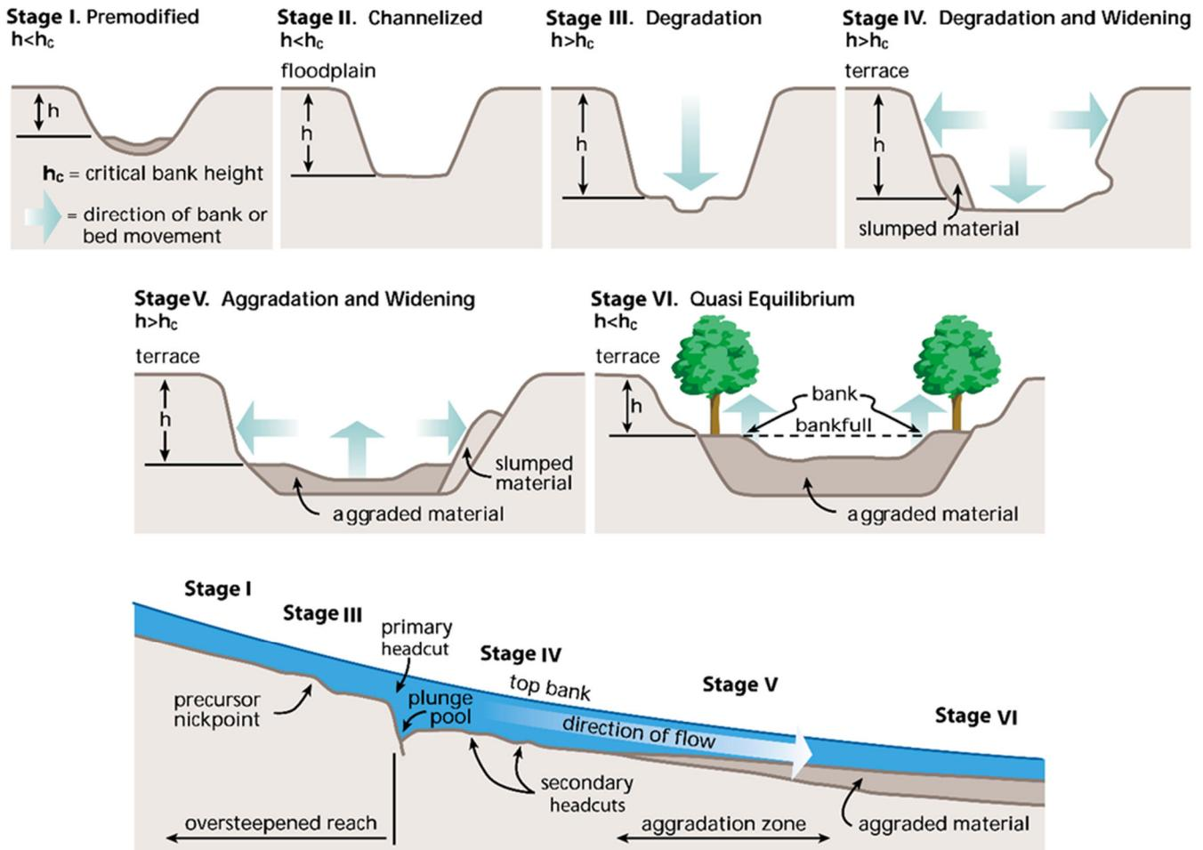
Figure 2.—Channel evolution model for incised channel response after a disturbance ([7], adapted from [11]).
