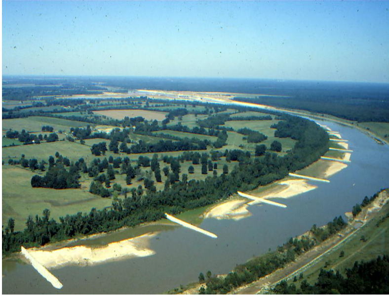
FIGURE 4.3 Hog Lake additional contraction structures
