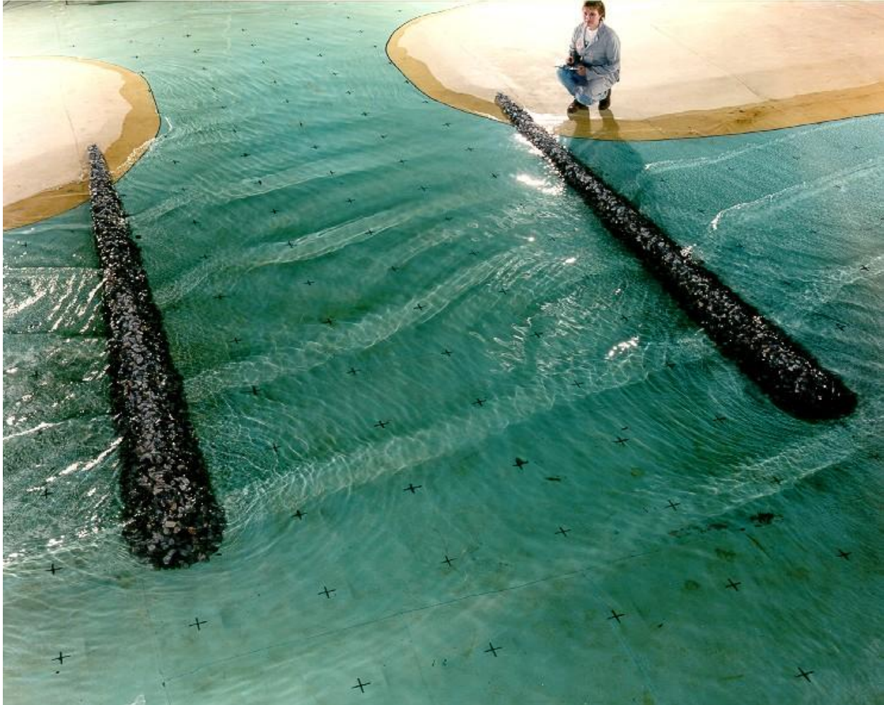
FIGURE 11.1 Idealized model inlet shown in a physical model
