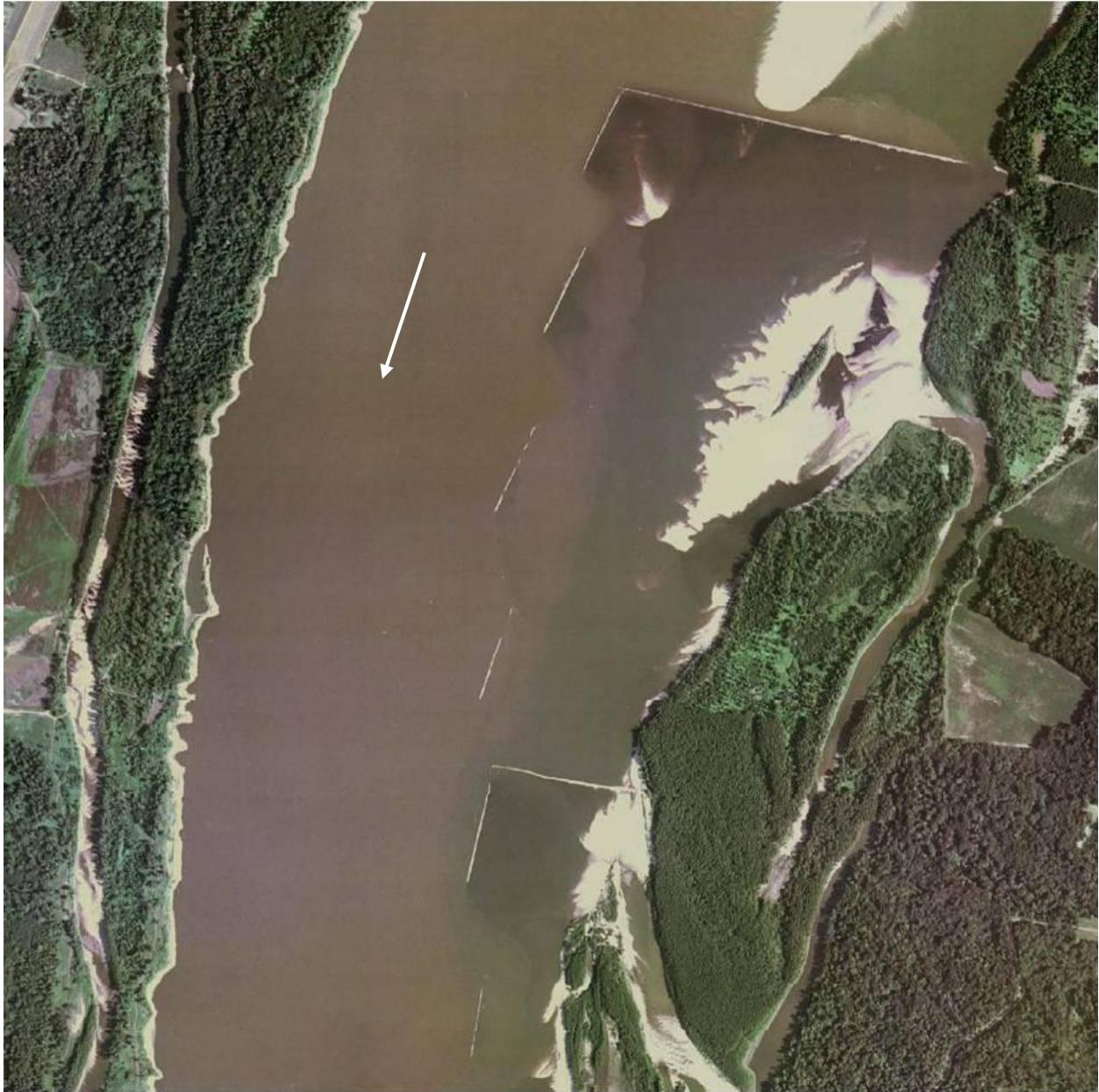
FIGURE 5.11 Vane dikes between L-head dikes on Mississippi River near Providence, LA
