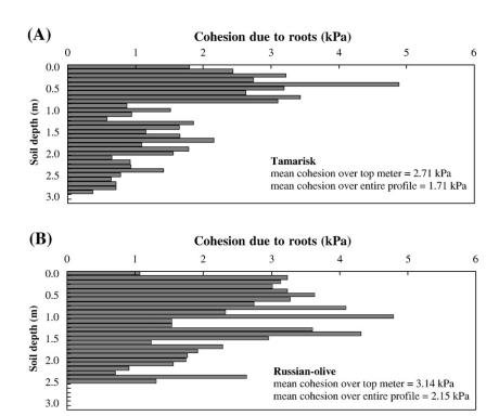
Fig. 3. Average values for cohesion from roots in each 0.1-m soil layer for Tamarisk (A) and Russian-olive (B).
