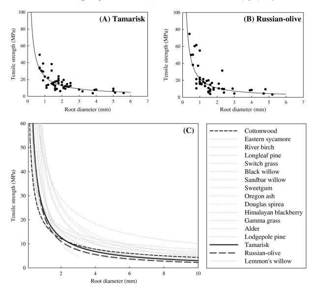
Fig. 2. Root tensile-strength measurements for Tamarisk (A) and Russian-olive (B) and relations for these species compared to other riparian species tested by the authors (C). To distinguish the specific curves of other species see Simon and Collison (2002), Pollen and Simon (2005), Simon et al. (2006).
