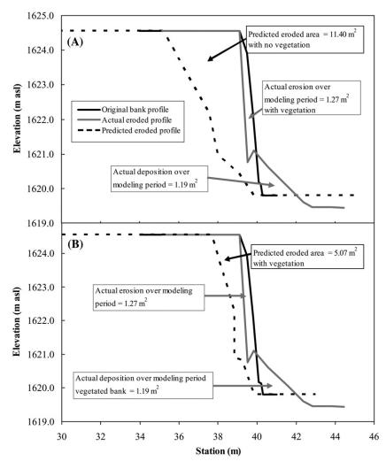
Fig. 8. Bank geometries for Sliding Rock site (SLR) at the beginning of the modeled period and after actual and predicted erosion. (A) Shows predicted erosion assuming no vegetation was present and (B) shows predicted erosion assuming Tamarisk and Russian-olive were present. In both (A) and (B) the final survey at the end of the modeled preiod is shown for comparison.
