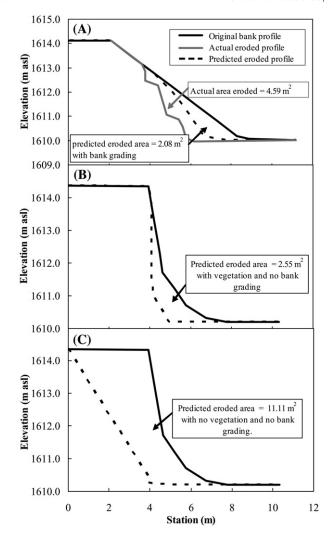
**Fig. 9.** Bank geometries for Upper White House site (UWH) at the beginning of the modeled period and after actual and predicted erosion. (A) Shows predicted erosion assuming no vegetation was present but the bank had been graded to a shallower angle. (B) and (C) show predicted erosion without grading of the bank with vegetation and without vegetation, respectively.
