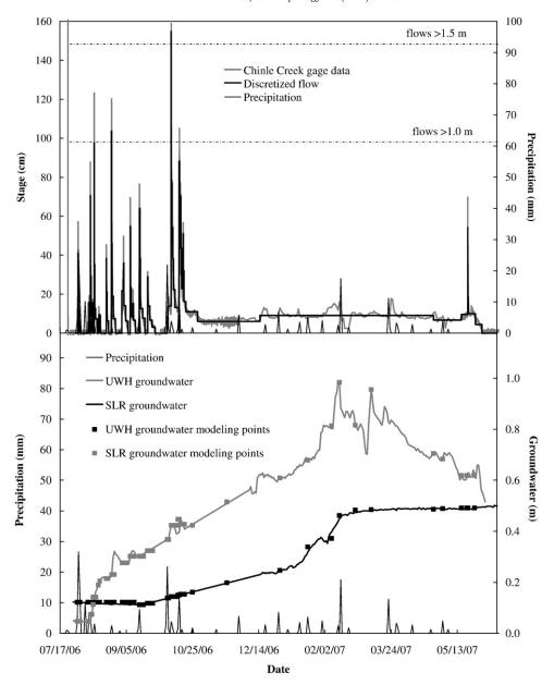
Fig. 5. Hydrologic data for modeled period (July 2006–July 2007), including precipitation, stage, groundwater elevation in wells, and discretized flow record for BSTEM modeling. For each discretized flow event the corresponding groundwater elevation was used in BSTEM.
