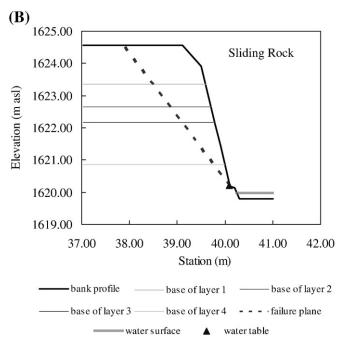
Fig. 4. Initial stable-bank configurations with vegetation for both study reaches.
