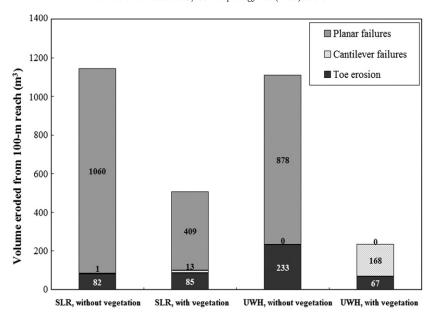
Fig. 7. Volumes of erosion predicted by BSTEM for a 100-m reach at UWH and SLR during interative modeling of toe erosion and bank stability. Total volumes of erosion are split into that emanating from hydrauilc scour of the toe versus that coming from planar and cantilever failures of the upper bank.
