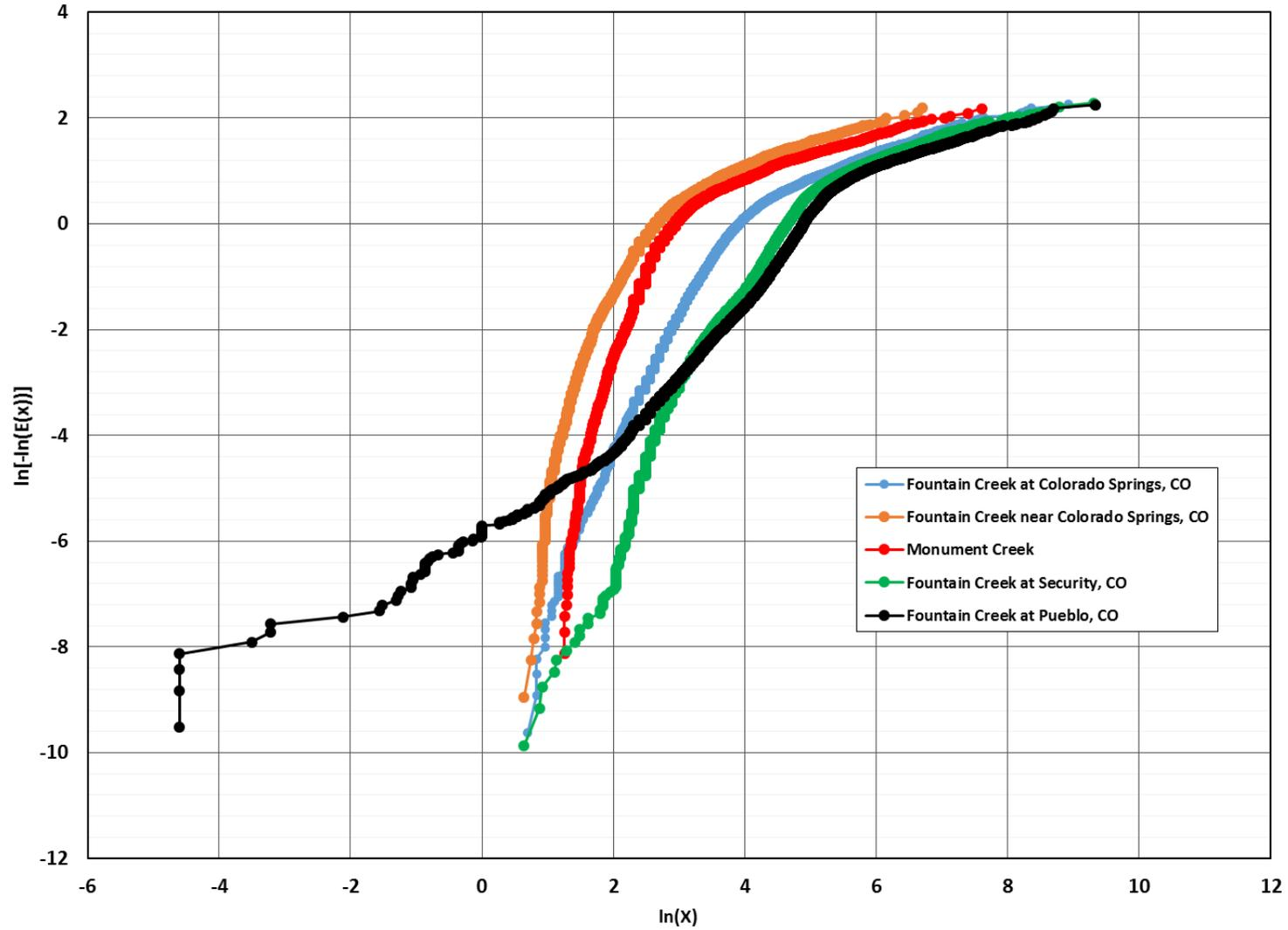
Figure 3. Relationship of  $\ln(x)$  and  $\ln[-\ln(E(x))]$  plotted to get the slope and intercepts for calculating the  $\hat{b}$  parameters.
