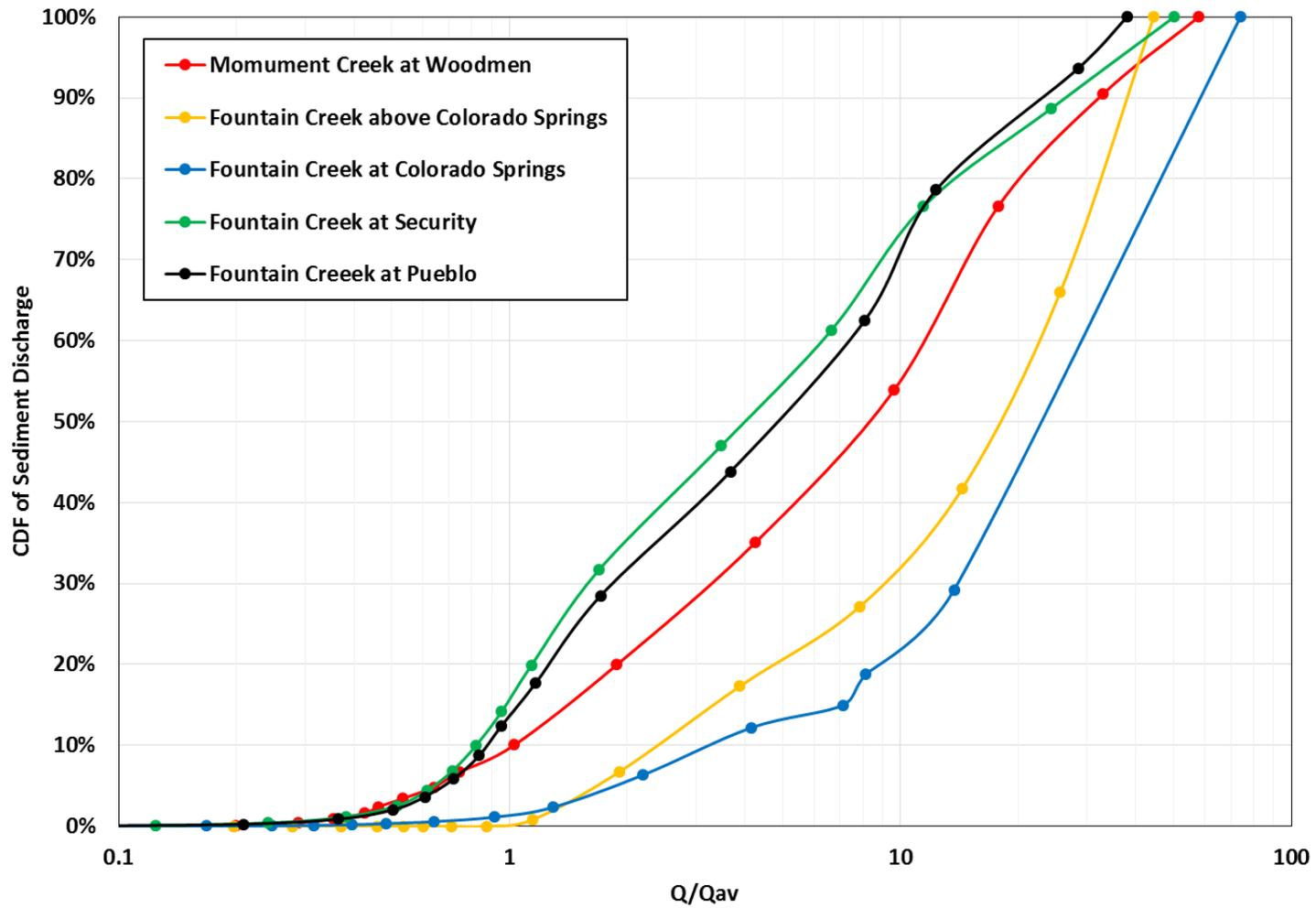
Figure 6. Summary of cumulative distribution function of sediment discharge as a function of  $Q/Q_{av}$ .
