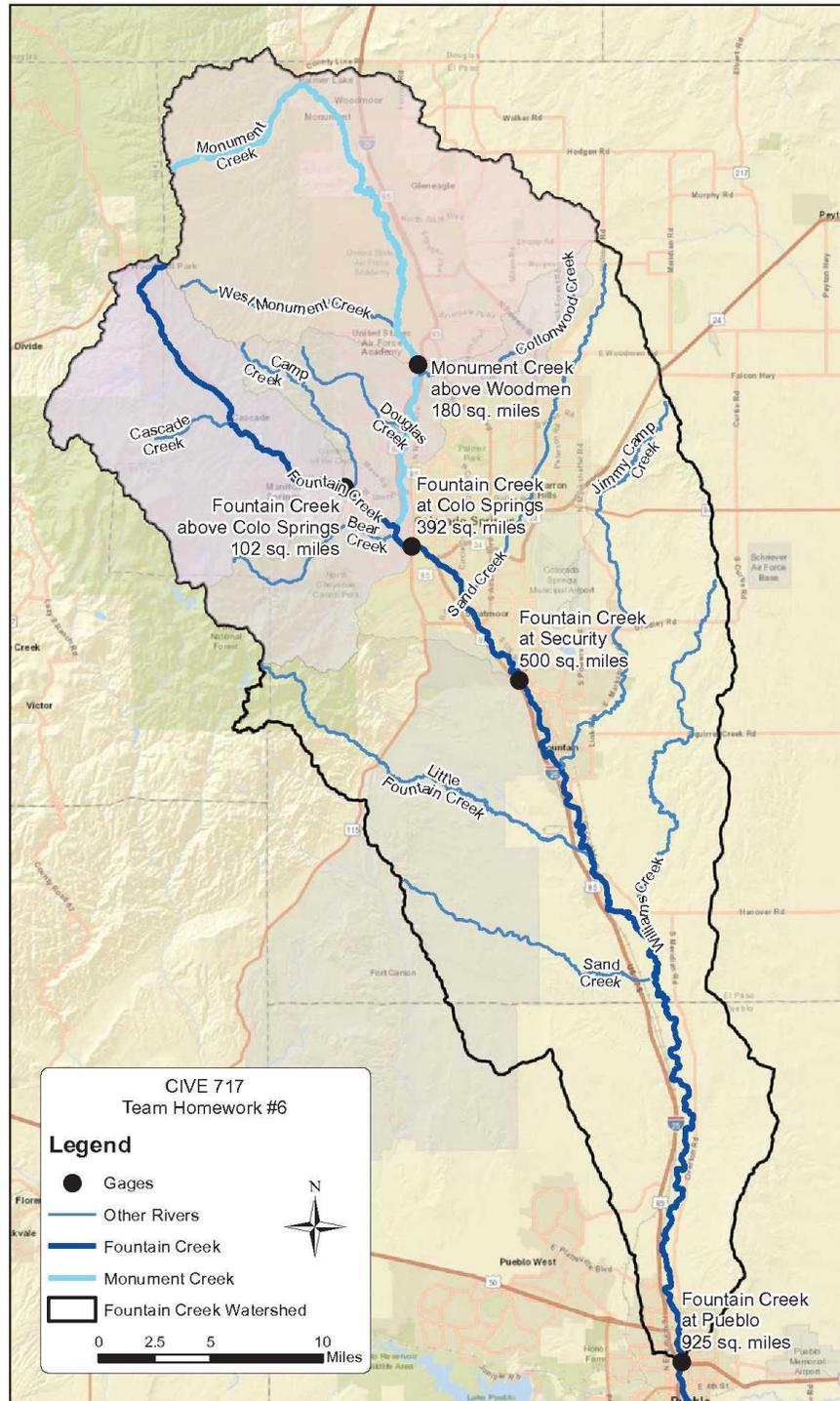
Figure 1. The five Fountain Creek and tributary gages and drainage areas in plan view.
