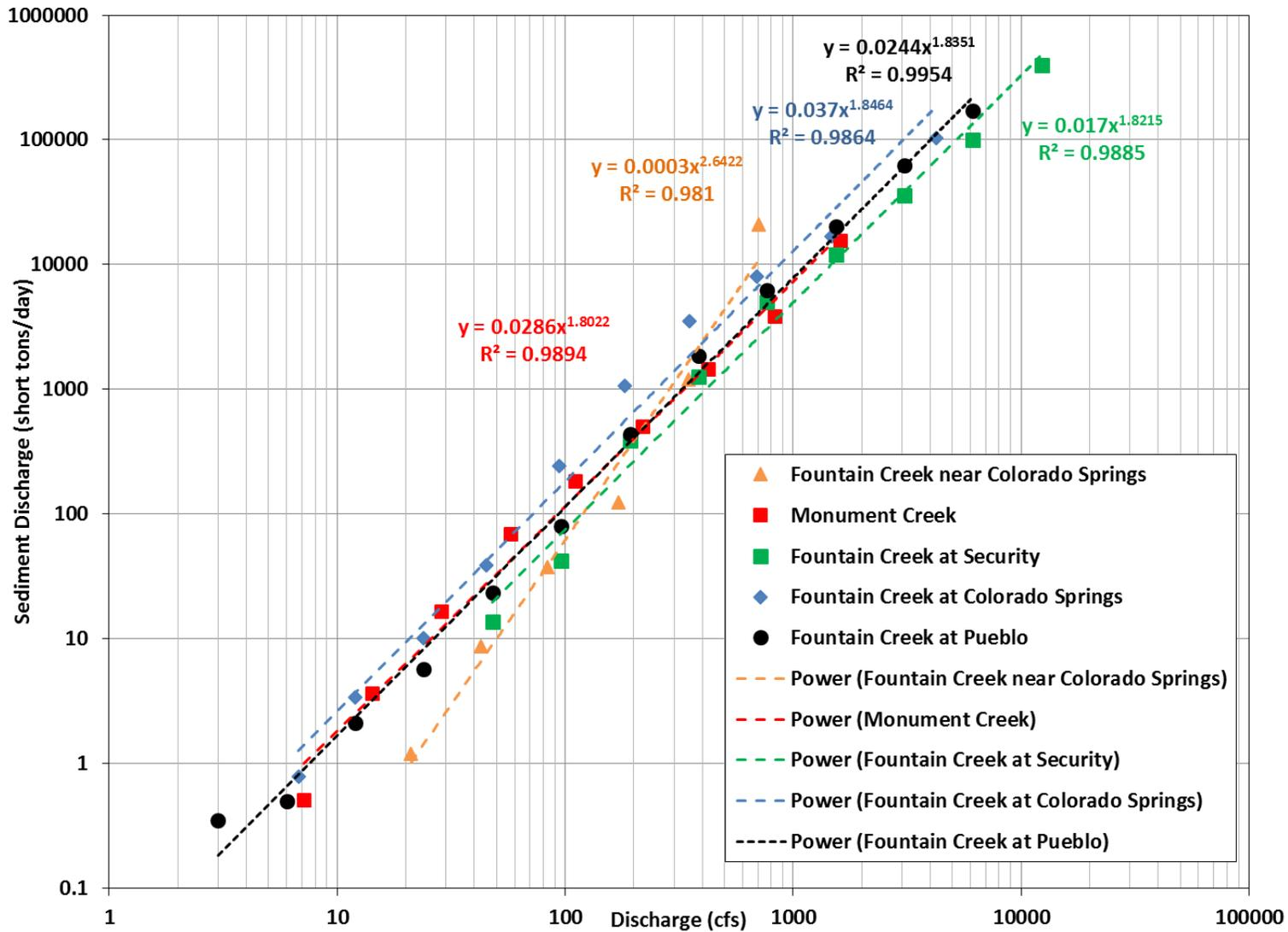
Figure 5. Sediment rating curves for all gages based on the averaged bin method.
