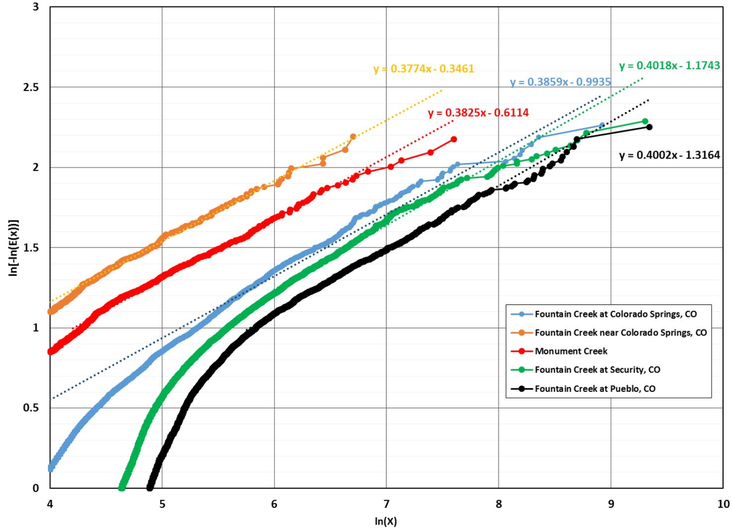
Figure 4. Close up of the best fit line for the  $\ln(x)$  and  $\ln[-\ln(E(x))]$  of the flow duration curve.
