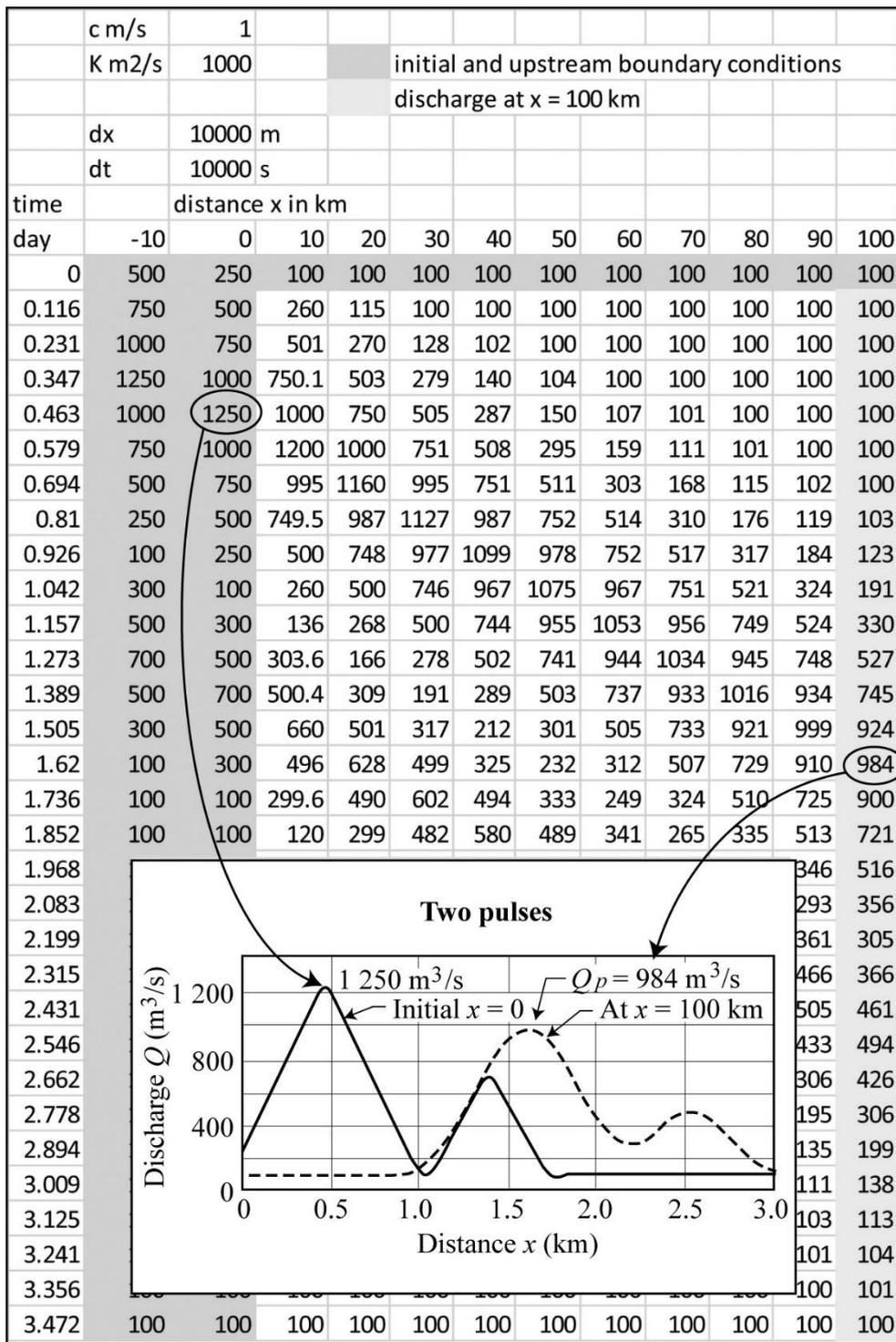
Fig. E-11.2. Numerical calculation table for floodwave propagation
