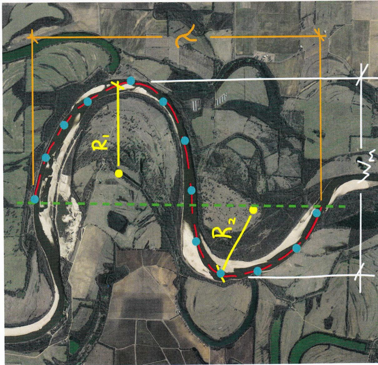
**Figure 1.** Red River meandering planform geometry
