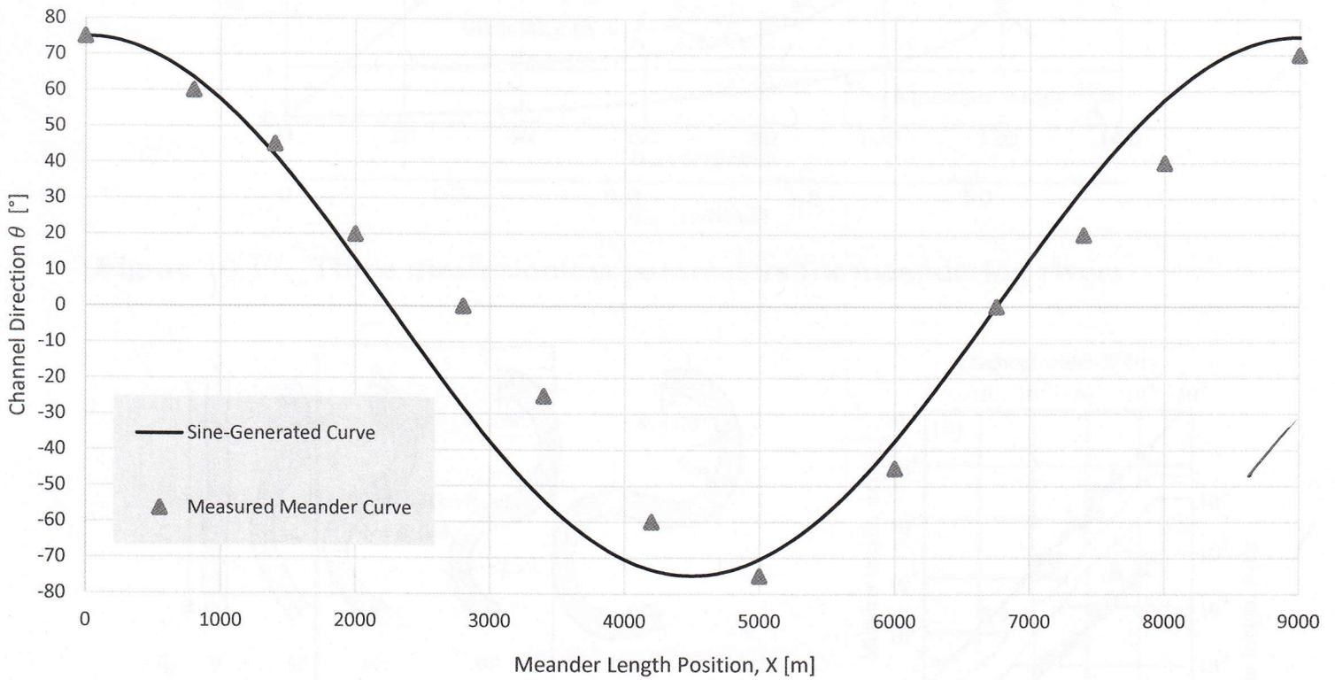
Figure 3. Sine-generated curve with measured meandering planform geometry
