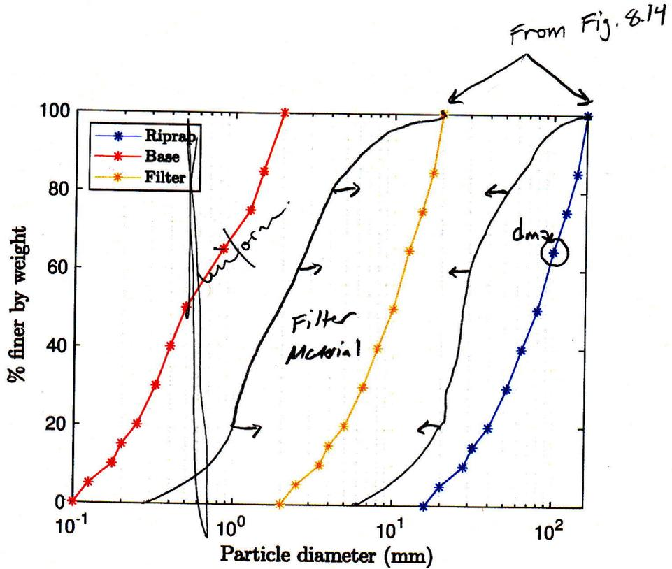
Figure 1: Gradation curve for riprap design, with  $d_m \approx 100$  mm.
