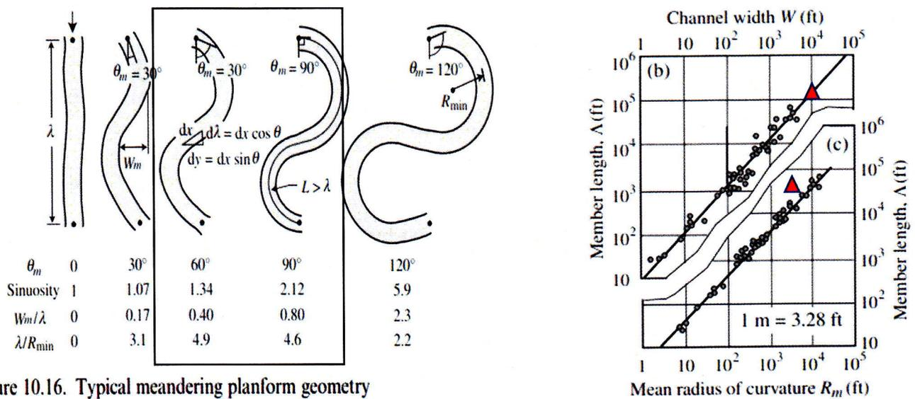
Figure 10.16. Typical meandering planform geometry
