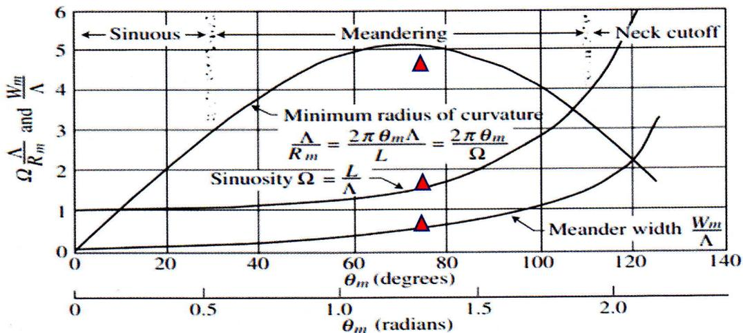
Figure 10.17. Three dimensionless parameters for meandering rivers
