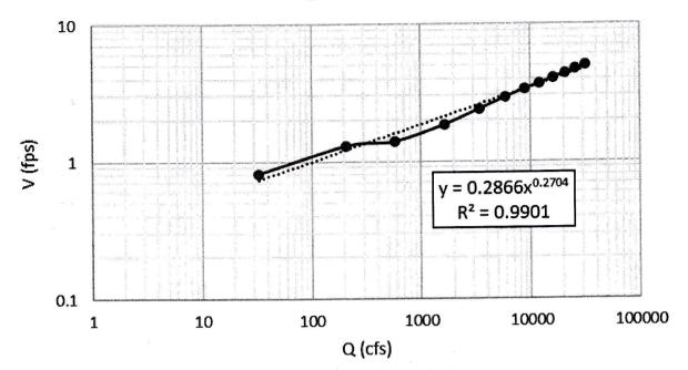
Figure 5. Plot of relationship between discharge and flow velocity.
