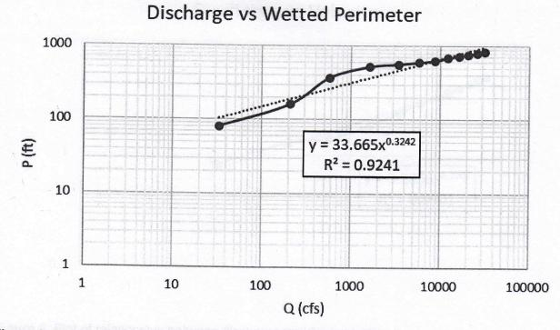
Figure 3. Plot of relationship between discharge and wetted perimeter.
