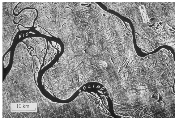
Figure 4.7 Side-looking-airborne-radar mosaic of large tract of floodplain between tributary rio Japurá and rio Solimões (local name for Amazon mainstem between Peru-Brazil border and confluence with rio Negro). River flow is from upper left to lower right. From Projeto RADAM (1973). This specific imagery has almost become a poster for large-scale changes in river-channel configuration: it was used, for example, as the dust-jacket picture for the book, River Channel Changes (Gregory, 1977). Since the time the imagery was collected (1971), the channel configurations here have continued to change. Within the last few years, for example, the narrow chute channel with the single near-perfect sine-curve meander that crossed the outer part of the neck of the great meander of rio Solimões (left side of figure) has widened, deepened, and straightened itself sufficiently to become part of the preferred navigation channel used by ocean-going ships to reach the upper-river ports of Leticia, Colombia, and Iquitos, Peru (Jacson Miranda, Amazon river pilot, personal communication, 2001). Other large tracts of stored fluvial sediment on floodplains of the Amazon and Madeira Rivers are described by Latrubesse (2002), Latrubesse and Franzinelli (2002), and by Mertes and Dunne in their chapter in the present volume (Chapter 8)
