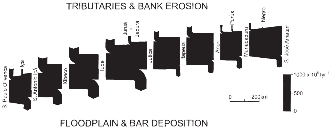
Figure 4.8 Diagrams showing average annual fluxes and exchanges of sediment between channels and floodplains of a 1500 km segment of the Amazon mainstem of Brazil, between the Peru-Brazil border and the confluence with rio Madeira. (a) Generalized diagram that shows schematically the averaged values for the entire 1500 km reach. Quantities of sediment exchanged through the erosion of banks and through deposition on point bars and floodplains significantly exceed the flux of sediment from upriver (including tributary inputs) or the flux continuing downriver. (b) An exploded version of (a), showing the individual sediment budgets for each of eight consecutive reaches of the mainstem Amazon between São Paulo de Olivença and São José do Amajari. The upper left corners show the quantities of sediment contributed to the eight segments from bank erosion. The lower right corners show the quantities removed from the channel by overbank deposition onto floodplains and pointbars. Details of the calculations and compilations are given by Dunne et al. (1998)
