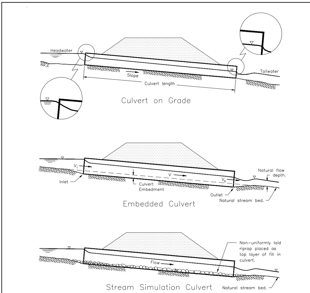
**Figure 2.4a** Culvert placement.
