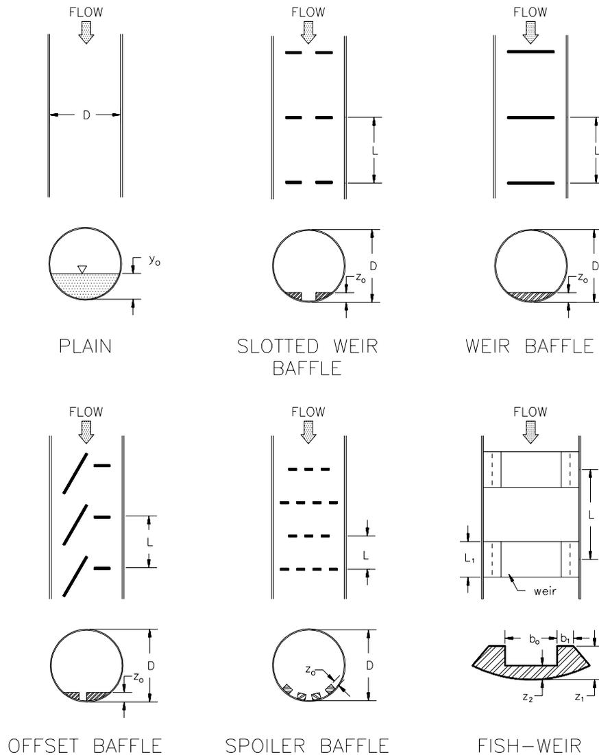
**Figure 5.6** Culvert fishways - baffle and weir arrangements.
