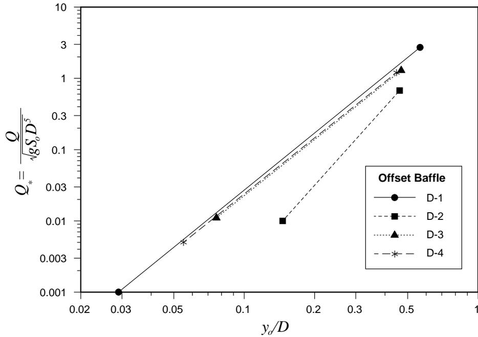
Figure 5.7 Offset baffle dimensionless discharge curves.
