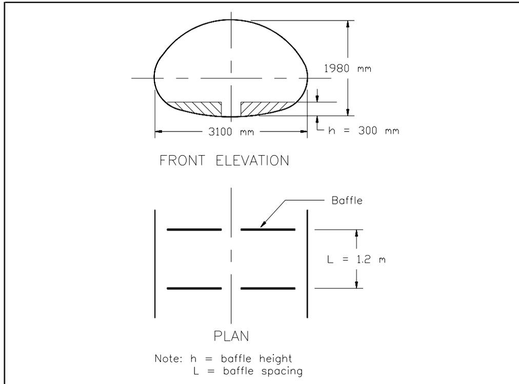
**Figure 8.3** Slotted weir culvert fishway for Altrude Creek.
