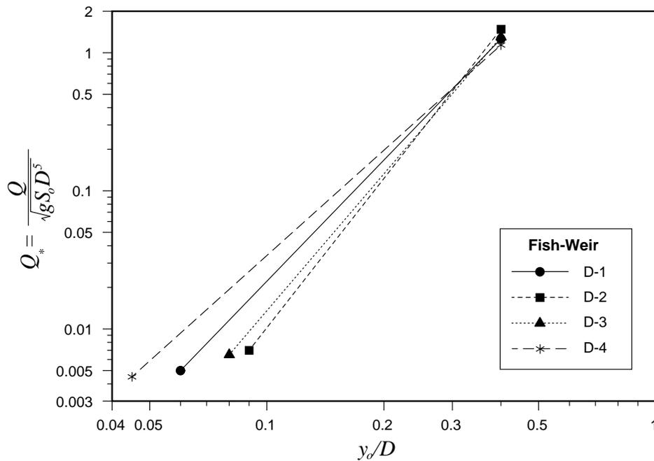
**Figure 5.13** Fish-weir dimensionless discharge curves.
