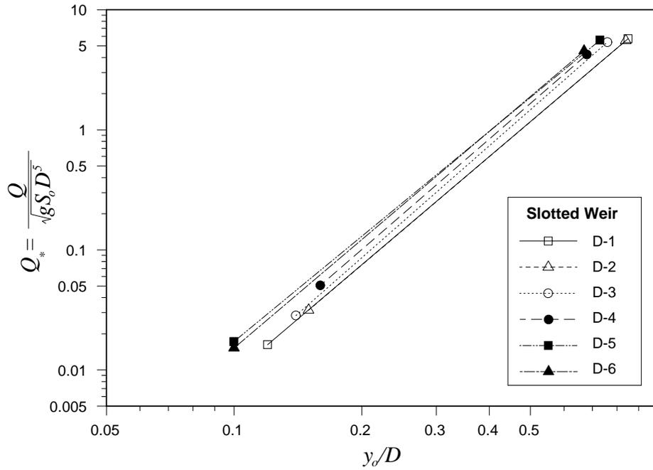
**Figure 5.11** Slotted weir baffle dimensionless discharge curves.
