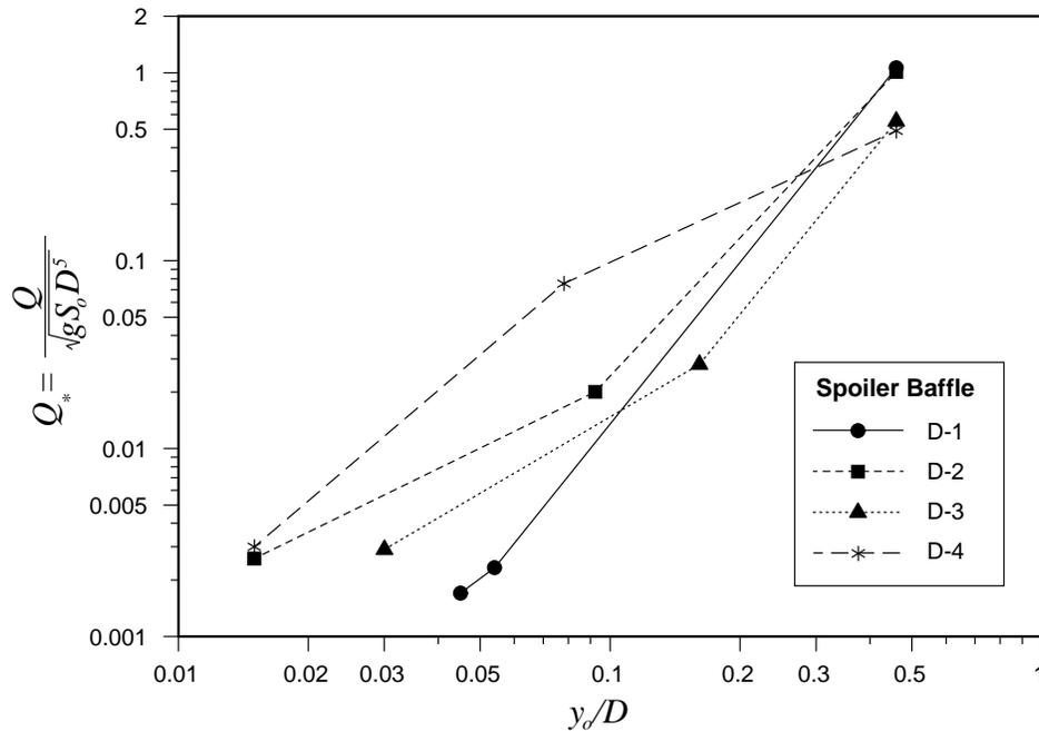
**Figure 5.14** Spoiler baffle dimensionless discharge curves.
