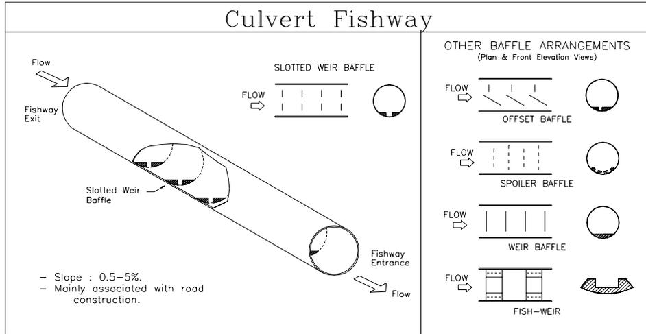
**Figure 2.4b** Culvert fishway.
