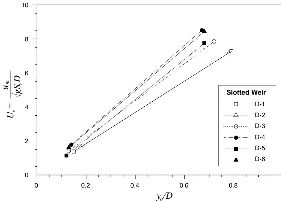
**Figure 5.12** Slotted weir baffle dimensionless velocity scales.
