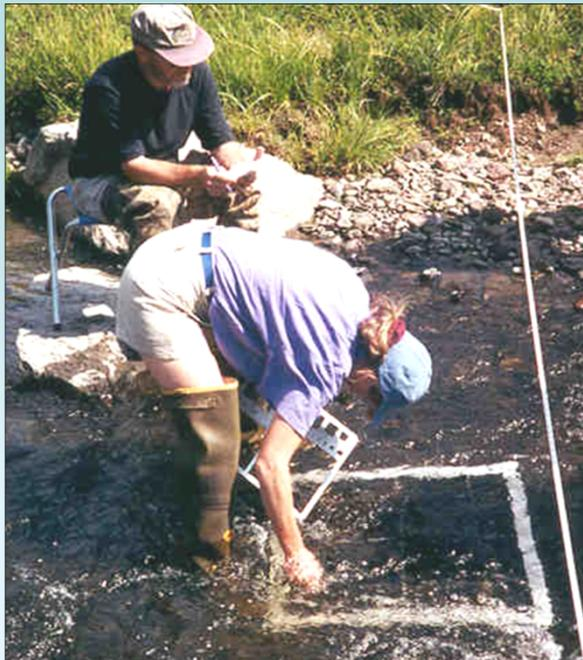
If the bed is not clearly visible, grid intersections (close to the bed) serve to guide the finger to the particle to be selected. There is a bias against hidden fines. Use plexiglass viewer to improve visibility.
