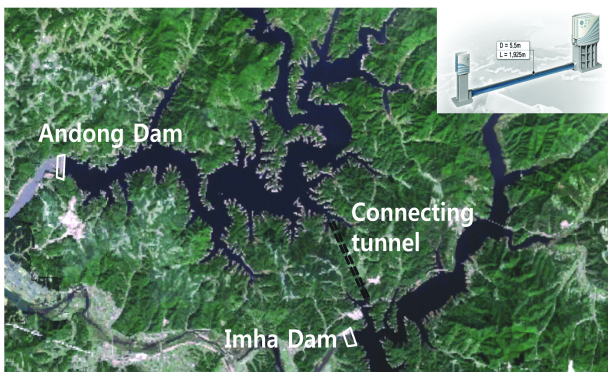
Fig. 1. A satellite image showing study area and the location where the diversion tunnel from Imha Reservoir to Andong Reservoir is constructed.
