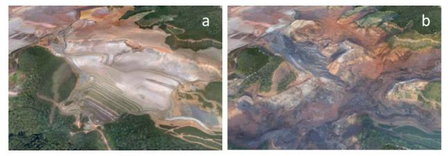
Figure 1 – Fundão Dam before (a) and after failure (b) (Morgenstern et al., 2016)
