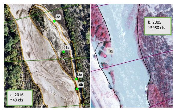
Figure 39: a. A dry side channel (3c) and islands (6b and 6e) are depicted above in an aerial photograph from 2016. Agg/Deg lines are shown in green lines perpendicular to the main channel. The active channel is outlined in orange. b. 1a depicts shoreline complexity in an aerial photograph from June of 2005. Agg/Deg lines are shown in purple perpendicular to the main channel. The active channel is outlined in black. The flow is going to the bottom of the page for both images.
