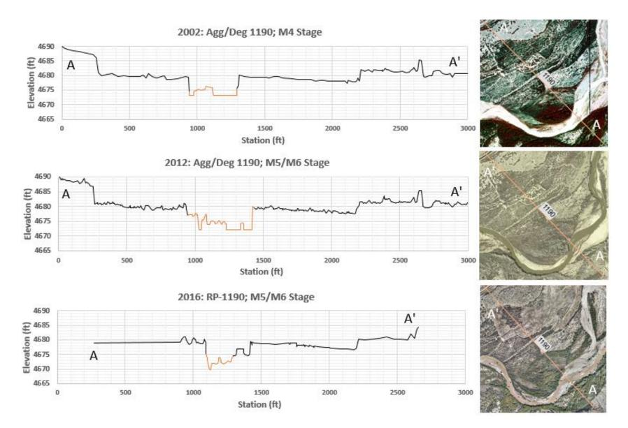
*Figure 30: 2002, 2012 and 2016 cross-section and planform views (planform to the right of each corresponding year). A denotes the left bank and A' denotes the right bank. The active channel is in orange and the channel classification is denoted at the top of the graph.*
