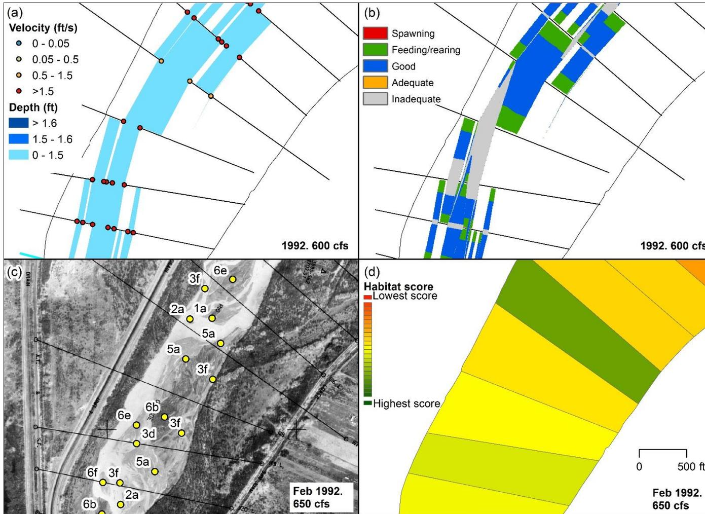
Summary of HEC-RAS and GIS habitat at subreach P1, agg/deg 1115 to 1121. (a) Velocity and depth of the simulation. (b) Habitat criteria mapped based on velocity and depth. (c) Habitat features mapped out by points and letters. (d) Habitat color scheme based on habitat features.
