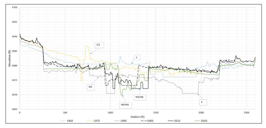
Figure 28: Comparison of cross-section 1190 from 1962-2016. Each stage classified by USBR is in a box and has an arrow pointing to the crosssection that it describes. These cross-sections are not compared after station 2600 because it is far away from the main channel. Also, there is very little variation in that area from year to year.
