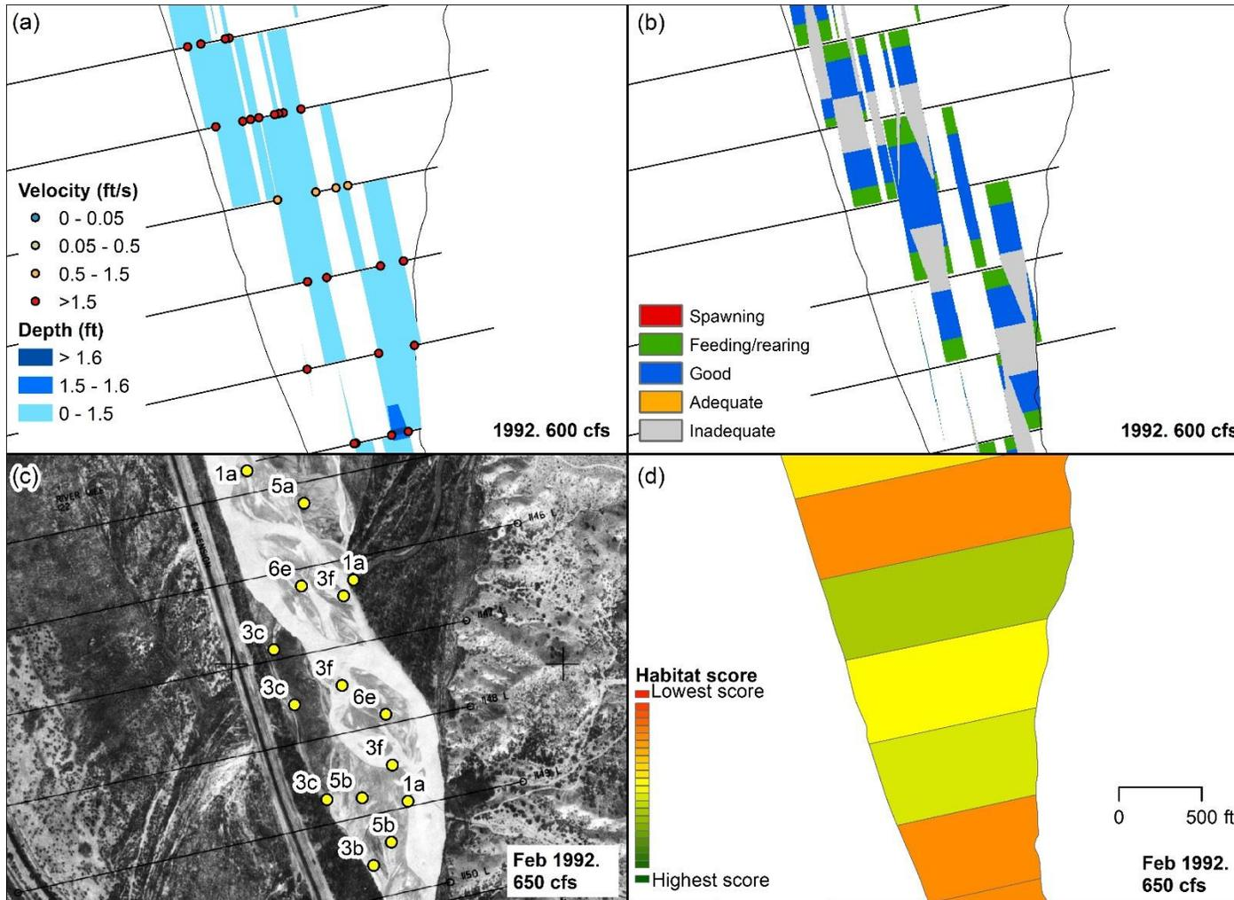
Summary of HEC-RAS and GIS habitat at subreach P2, agg/deg 1145 to 1150. (a) Velocity and depth of the simulation. (b) Habitat criteria mapped based on velocity and depth. (c) Habitat features mapped out by points and letters. (d) Habitat color scheme based on habitat features.
