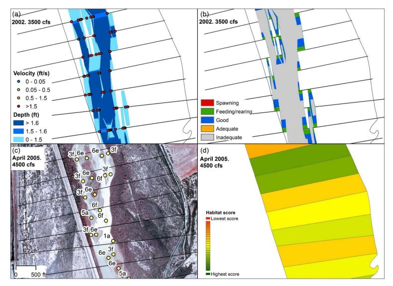
*Figure 55: Summary of HEC-RAS and GIS habitat at subreach P2, agg/deg 1137 to 1143. (a) Velocity and depth of the simulation. (b) Habitat criteria mapped based on velocity and depth. (c) Habitat features mapped out by points and letters. The description of these points is given in Appendix A and section 5.2.3. (d) Habitat color scheme based on habitat features.*
