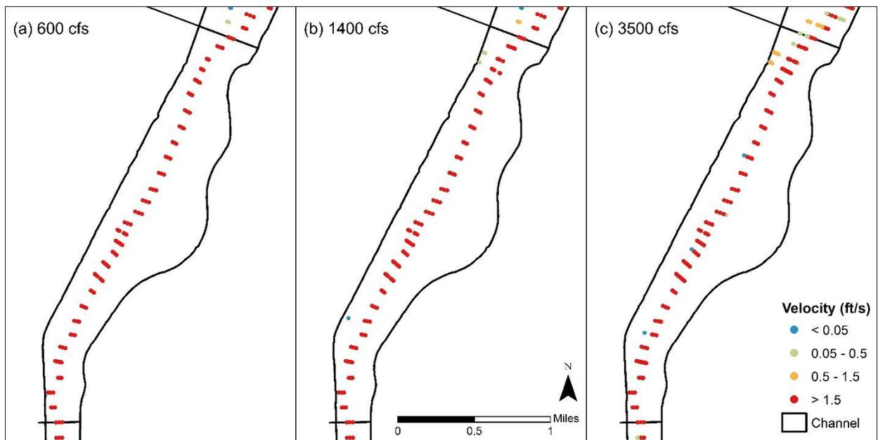
Figure 33: Simulated velocity at subreach I1 at flow rate 600, 1400, and 3500 cfs in 2012.
