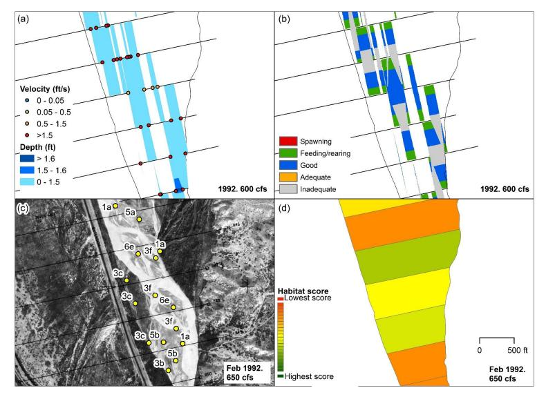
*Figure 54: Summary of HEC-RAS and GIS habitat at subreach P2, agg/deg 1145 to 1150. (a) Velocity and depth of the simulation. (b) Habitat criteria mapped based on velocity and depth. (c) Habitat features mapped out by points and letters. The description of these points is given in Appendix A and section 5.2.3. (d) Habitat color scheme based on habitat features.*
