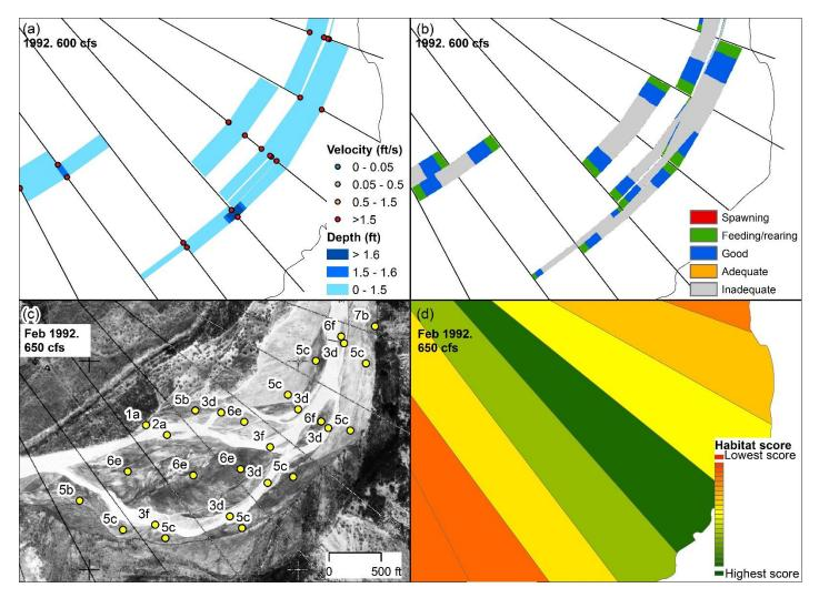
Summary of HEC-RAS and GIS habitat at subreach P4, agg/deg 1187 to 1193. (a) Velocity and depth of the simulation. (b) Habitat criteria mapped based on velocity and depth. (c) Habitat features mapped out by points and letters. (d) Habitat color scheme based on habitat features.
