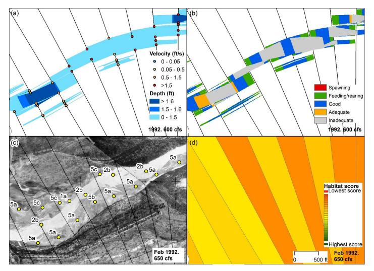
Summary of HEC-RAS and GIS habitat at subreach P5, agg/deg 1196 to 1204. (a) Velocity and depth of the simulation. (b) Habitat criteria mapped based on velocity and depth. (c) Habitat features mapped out by points and letters. (d) Habitat color scheme based on habitat features.
