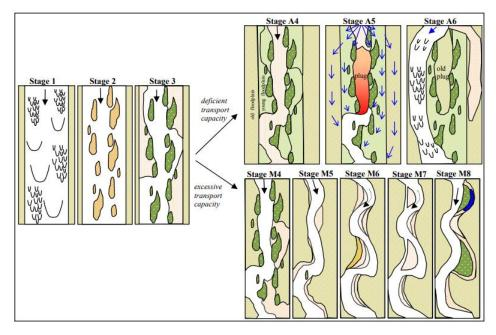
*Figure 27: Planform evolution model from Massong et al. (2010). The river undergoes stages 1-3 first and then A4-A6 or M4-M8 depending on the transport capacity.*
