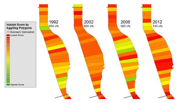
Figure 46: Subreach P2 summation of habitat scores indicated by the color scheme in the legend and separated by agg/deg lines. Only years around 650 cfs are shown. 2001 is excluded because location of the gage is far away from this study site, so this information is not as accurate.
