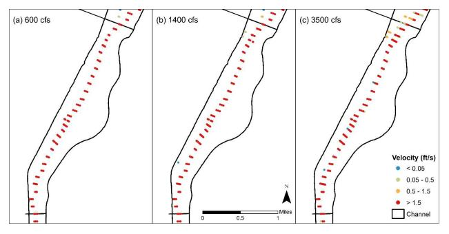
Figure 33: Simulated velocity at subreach I1 at flow rate 600, 1400, and 3500 cfs in 2012.
