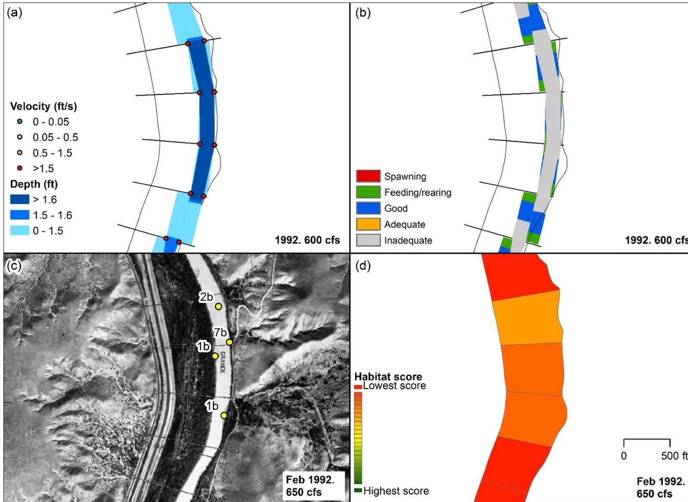
Summary of HEC-RAS and GIS habitat at subreach P3, agg/deg 1162 to 1167. (a) Velocity and depth of the simulation. (b) Habitat criteria mapped based on velocity and depth. (c) Habitat features mapped out by points and letters. (d) Habitat color scheme based on habitat features.
