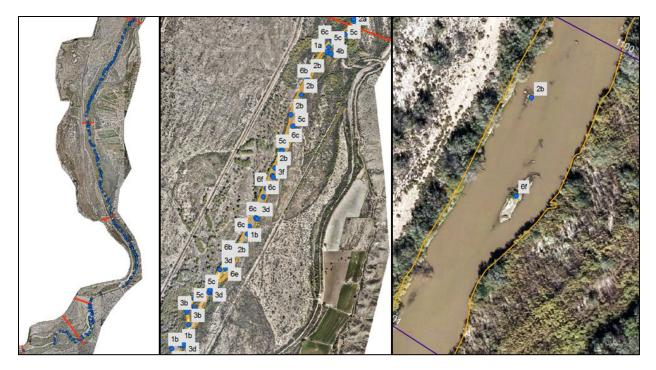
Figure 40: Examples of points being assigned zoomed in at three different magnitudes. The right is the furthest zoomed in and depicts points between two agg/deg lines. The left most image is the entire Rio Puerco Reach. Blue dots are points assigned to features and the orange line outlines the active channel.
