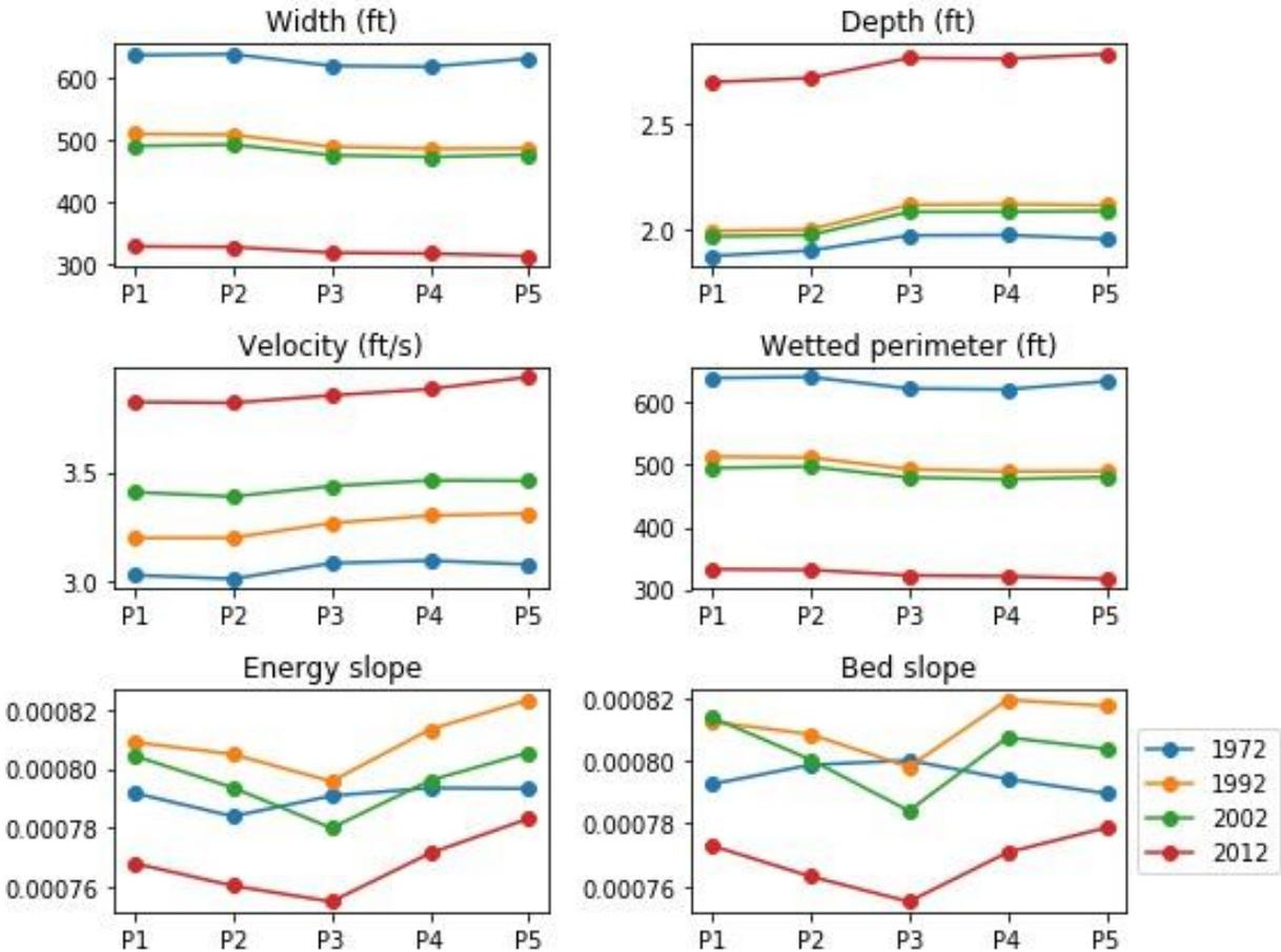
Figure 26: Width, depth, velocity, wetted perimeter, energy slope, and bed slope at each subreach for 1972, 1992, 2002, and 2012 at 3000 cfs.
