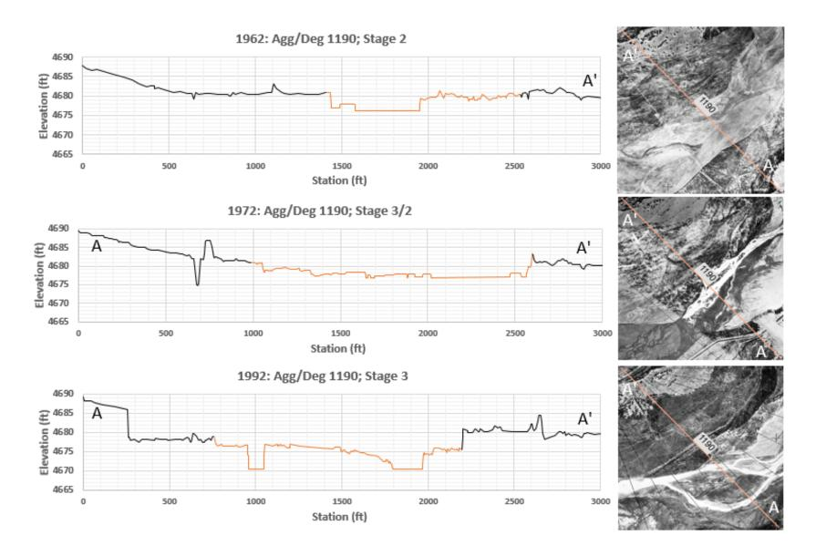
*Figure 29: 1962, 1972 and 1992 cross-section and planform views (planform to the right of each corresponding year). A denotes the left bank and A' denotes the right bank. The active channel is in orange and the channel classification is denoted at the top of the graph.*
