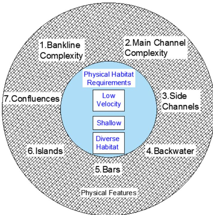
Figure 38. Physical habitat requirements are listed in the blue inner circle. Physical features that meet these requirements and can be seen from aerial photography are in the outer circle.
