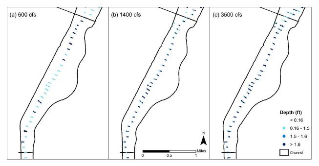
Figure 32: Simulated depth at subreach I1 at flow rate 600, 1400, and 3500 cfs in 2012.
