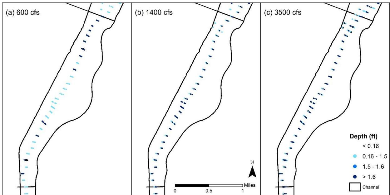
Figure 32: Simulated depth at subreach I1 at flow rate 600, 1400, and 3500 cfs in 2012.
