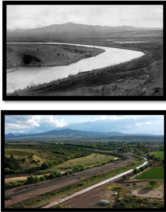
Figure 8. Comparison of Indian Hills Farm, TX, before (1905) and after (2014) floodway construction (McDonald, 2015)
