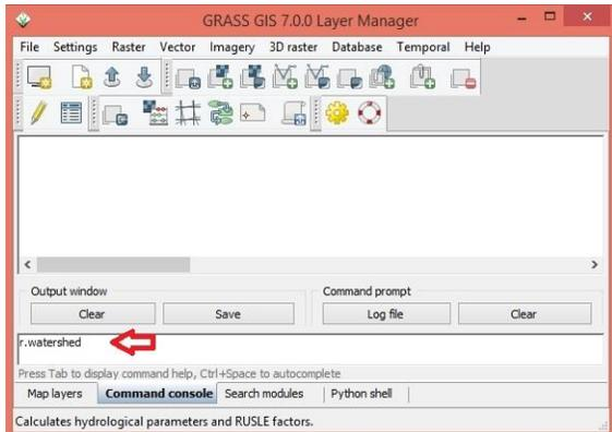
2. At “r.watershed” window you will set the parameters “(elevation=name)” with the raster layer that you have containing terrain elevations. Also, you will fill the blank “(threshold=integer)” with the value of the minimum watershed area that you expect, then you must divided it per your resolution’s layer (i.e.  $62 = 500000\text{m}^2 / (90 \times 90\text{m}^2)$ ).
