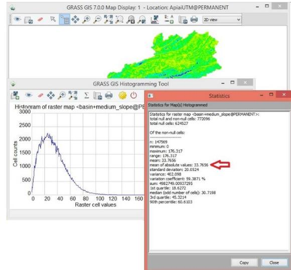
Figure 12: Result of the mean slope at the watershed area.
