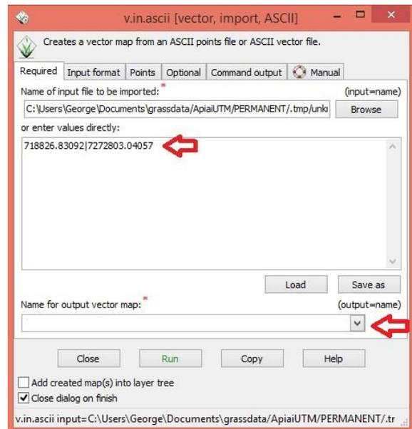
9. The expected result to the “v.in.asc” command is going to be as the picture below.
