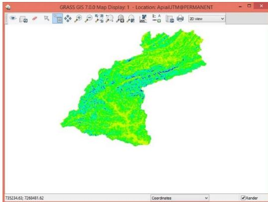
Figure 11: Result of cropping the slope map to the watershed shape.
