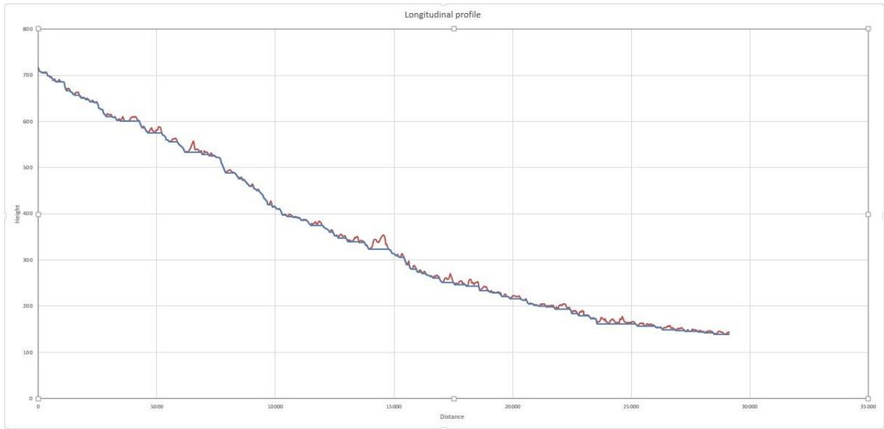
Figure 18: Result from plotting the original and the corrected data set of the mainchannel.
