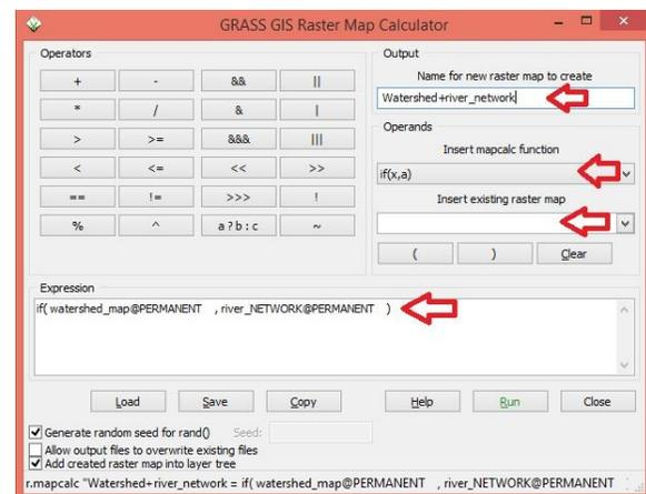
4. Since the checkbox “Add the generated raster map into layer tree” is checked, the resulting stream network will be shown with its name in the layer tree as well as into the Map Display window with the watershed shape as depicted in the Figure 13.
