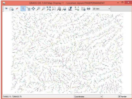
Figure 6: Obtained result from the topic “River network extraction” using a raster map with the ground elevations.
