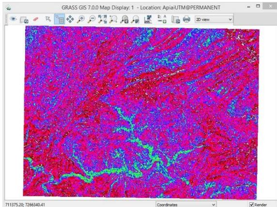
Figure 10: Result from using an elevations map to create a slope map.
