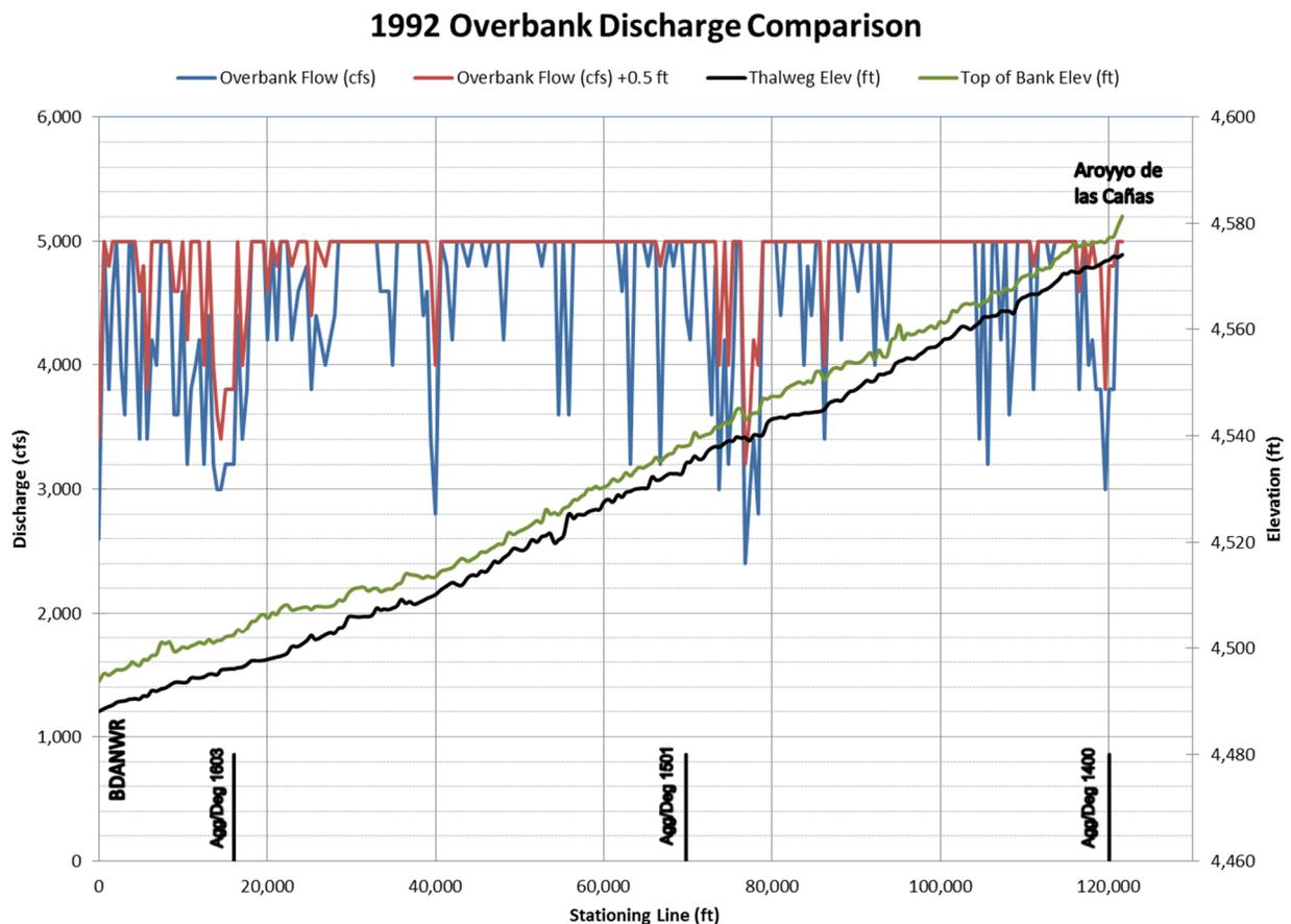
Figure 32 – 1992 comparisons of low bank line elevation and 0.5 ft higher
