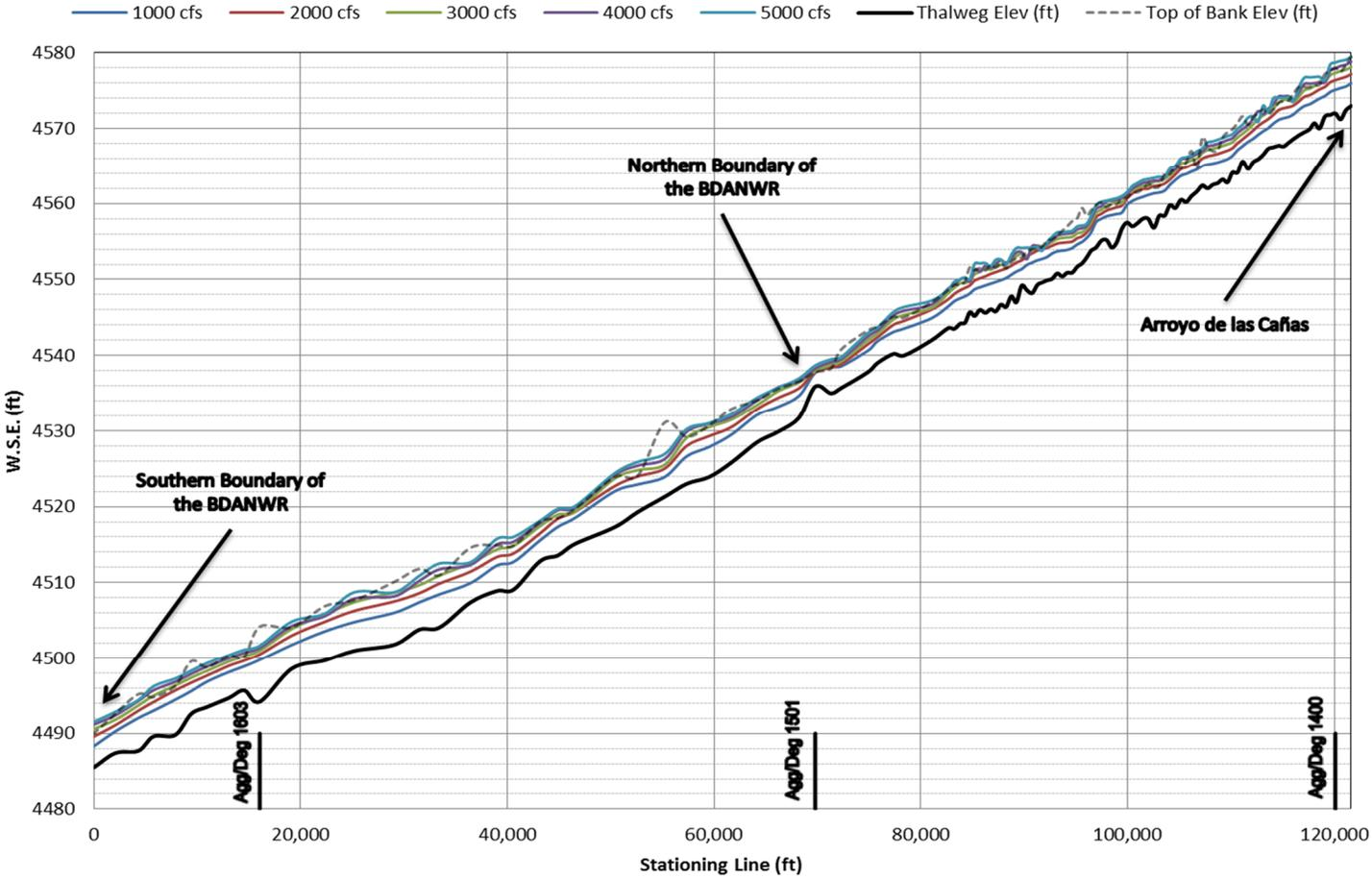
Figure 17 – 1972 Water surface profile plot vs. upstream distance
