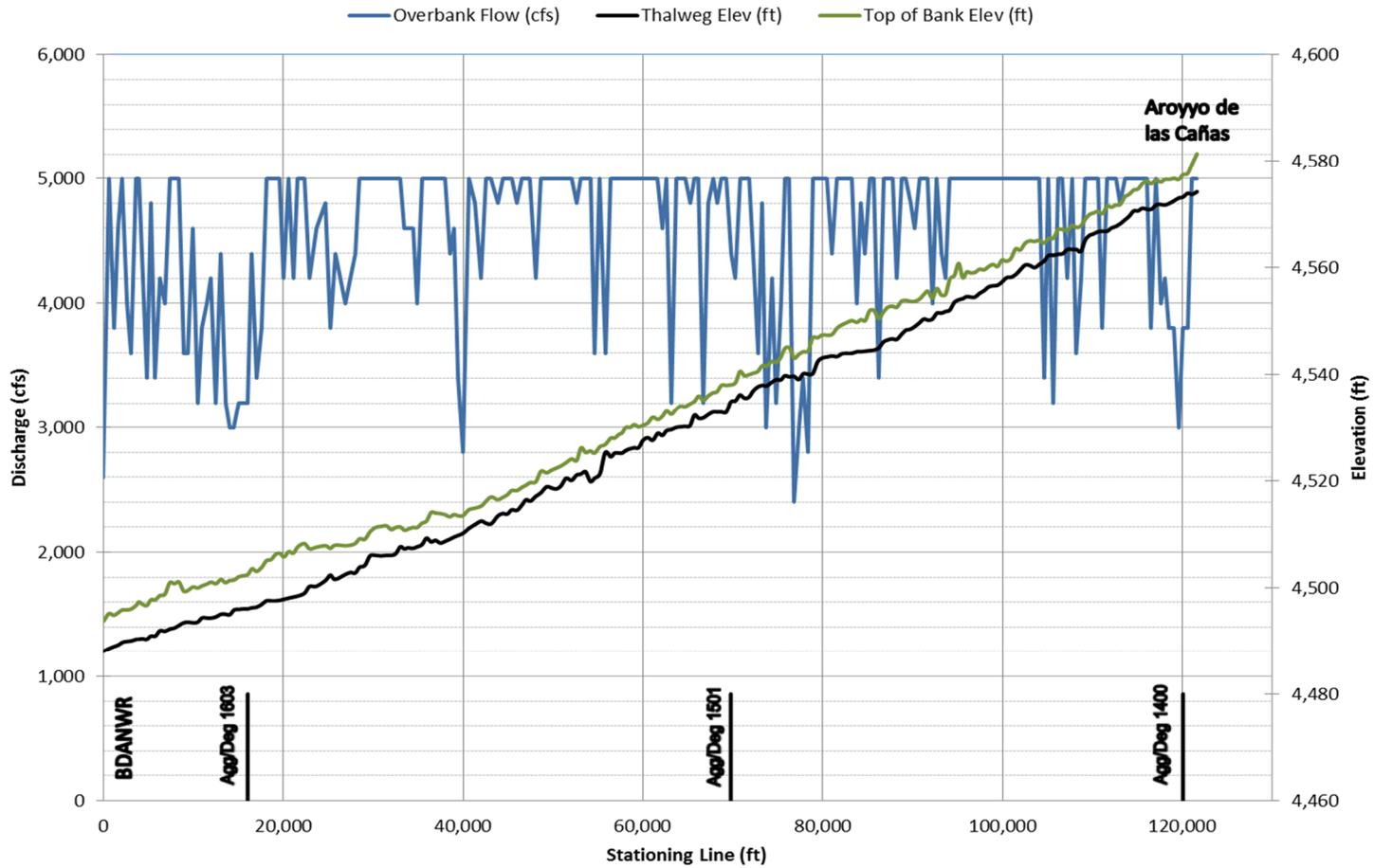
Figure 27 – 1992 Overbank flow vs. upstream distance
