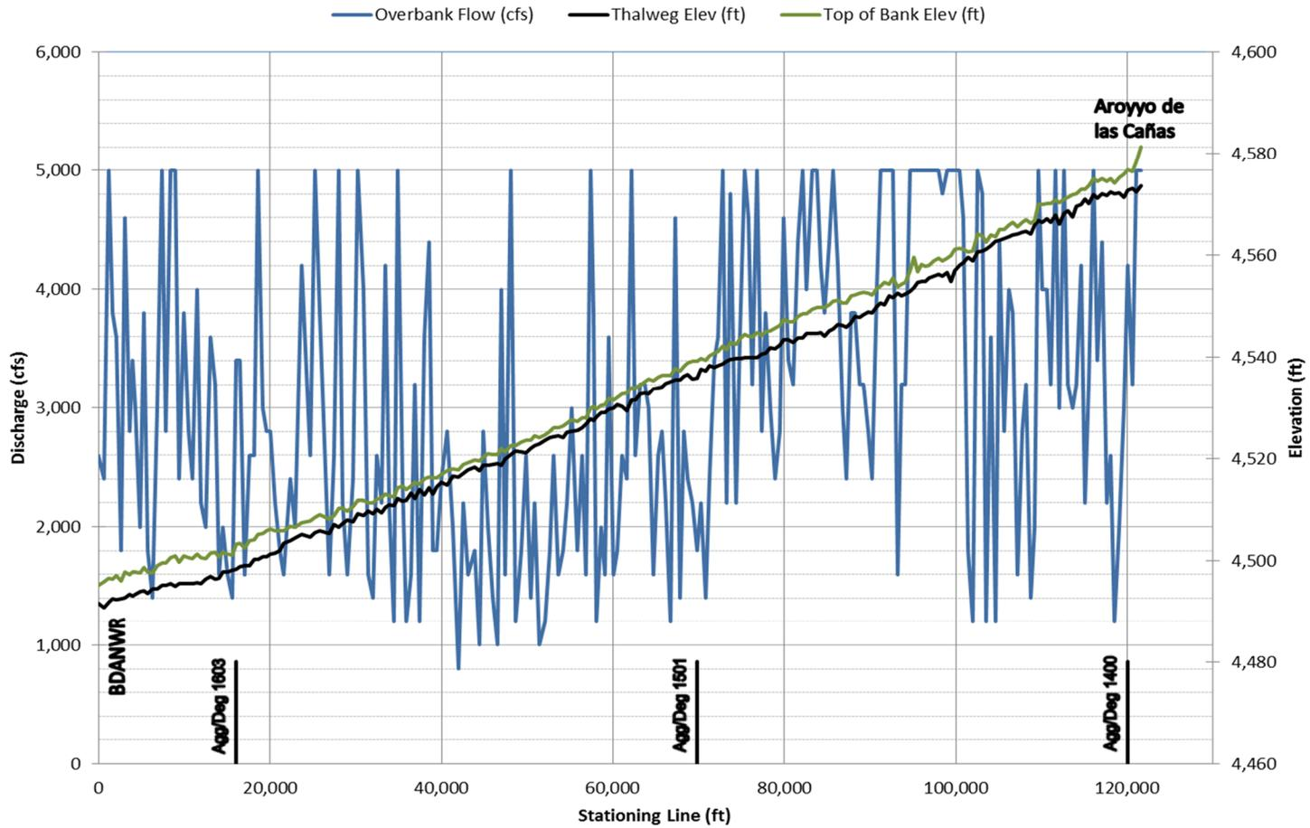
Figure 28 – 2002 Overbank flow vs. upstream distance
