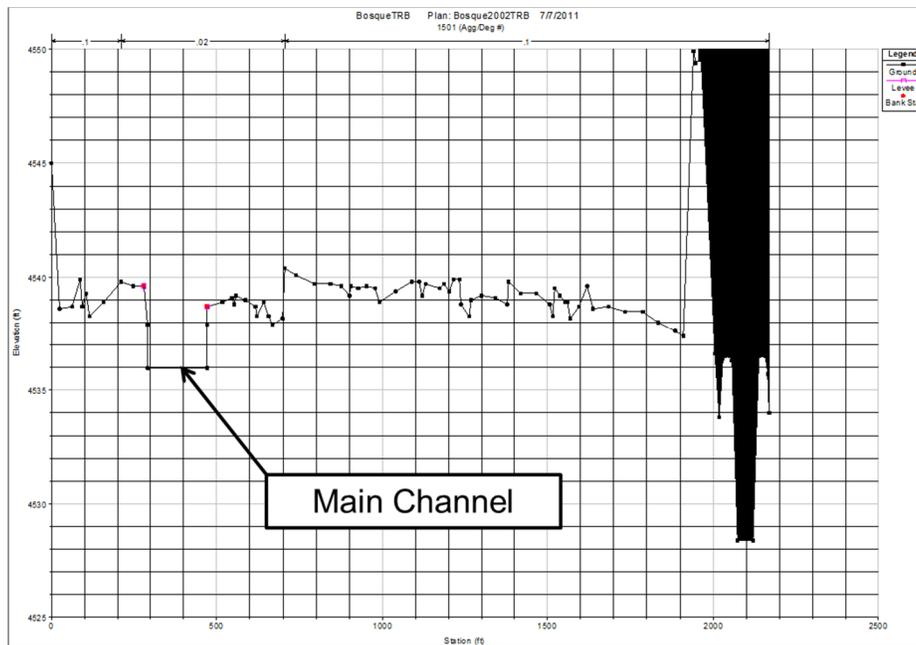
*Figure 5 – Typical HEC-RAS cross-section*
