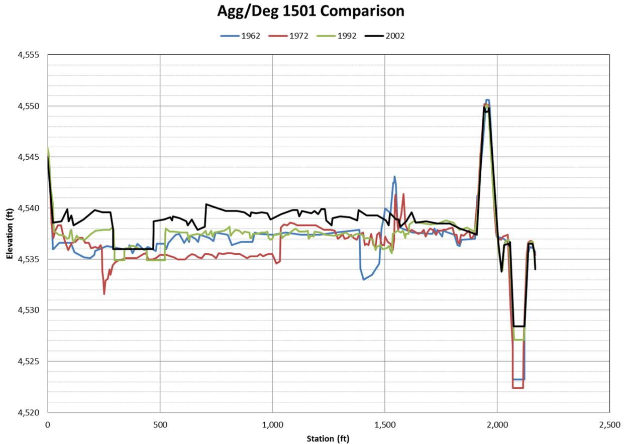
*Figure 39 – Agg/Deg 1501 geometry for 1692, 1972, 1992, and 2002*
