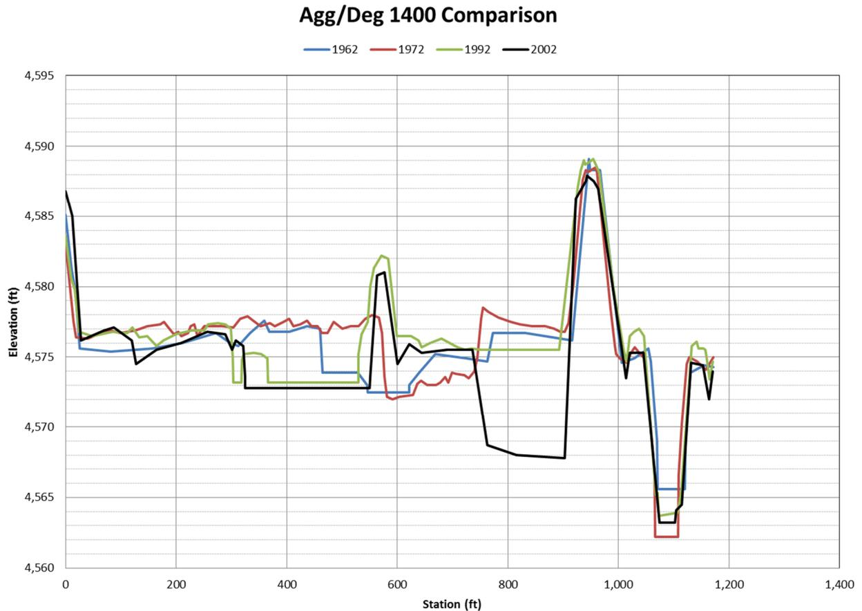
*Figure 38 – Agg/Deg 1400 geometry for 1962, 1972, 1992, and 2002*
