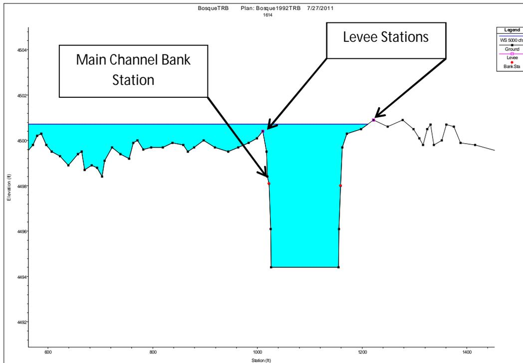
*Figure 12 – 1992 Agg/Deg 1614 cross-section*
