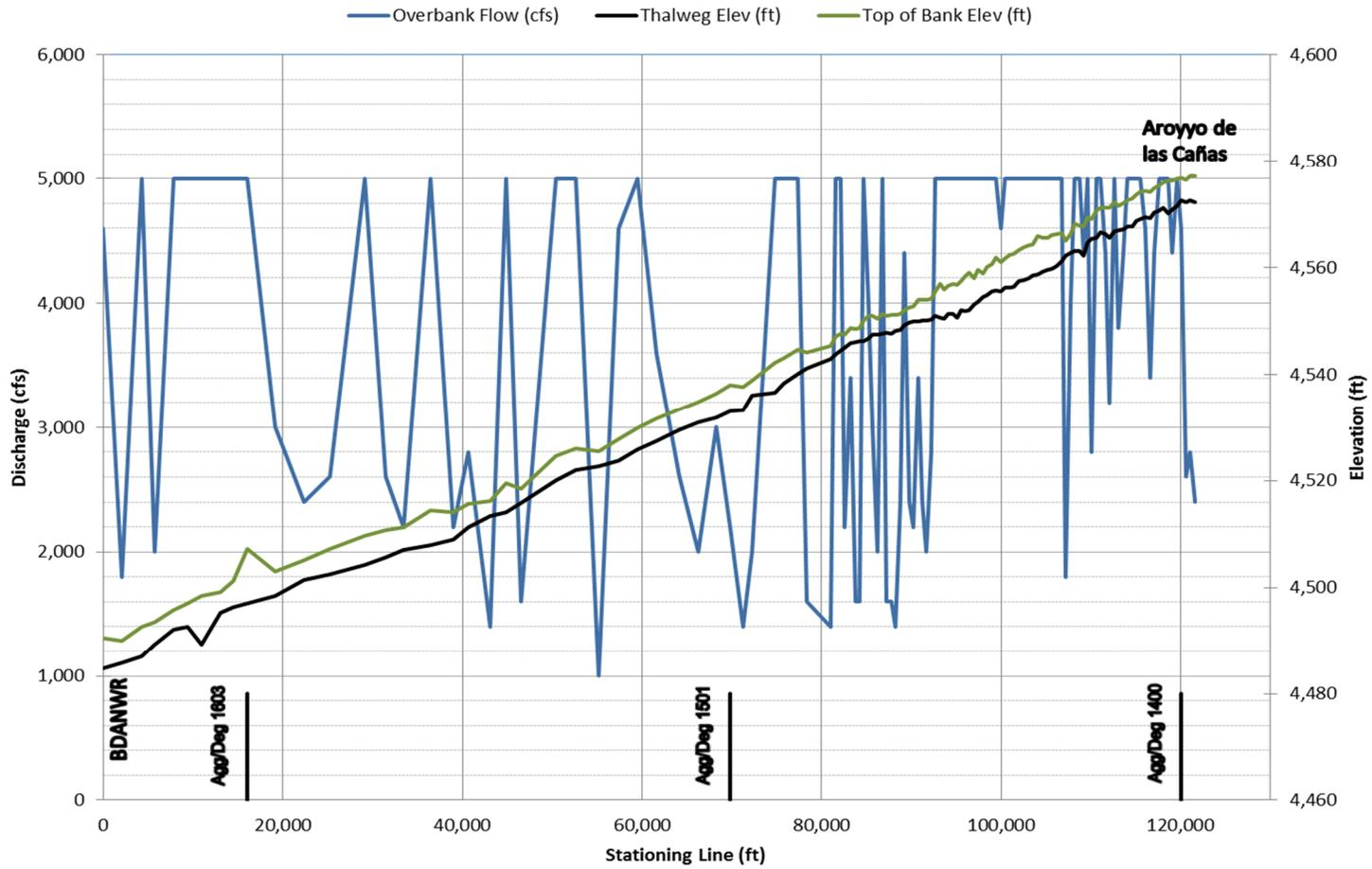
Figure 25 – 1962 Overbank flow vs. upstream distance
