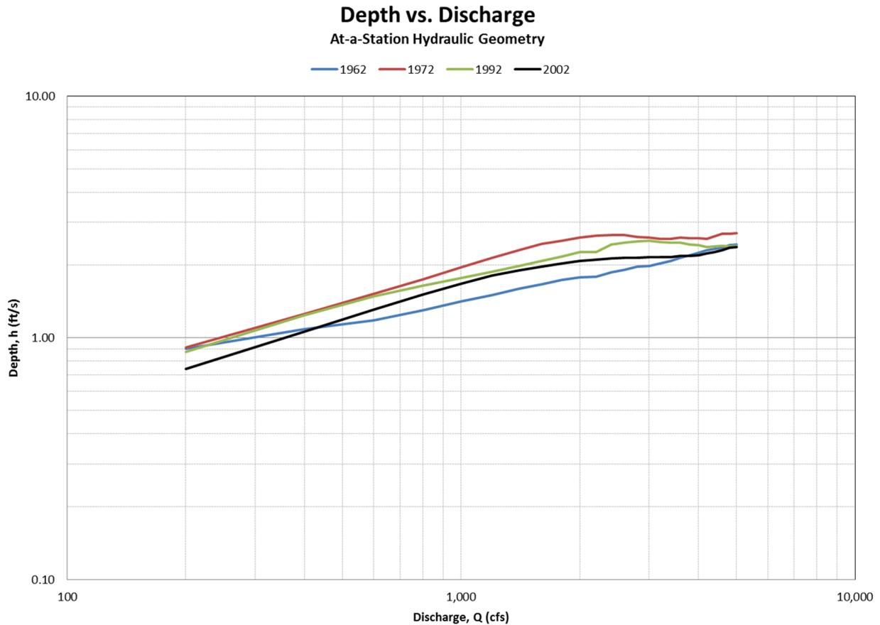
Figure 35 – Mean flow depth vs. discharge at-a-station relationship
