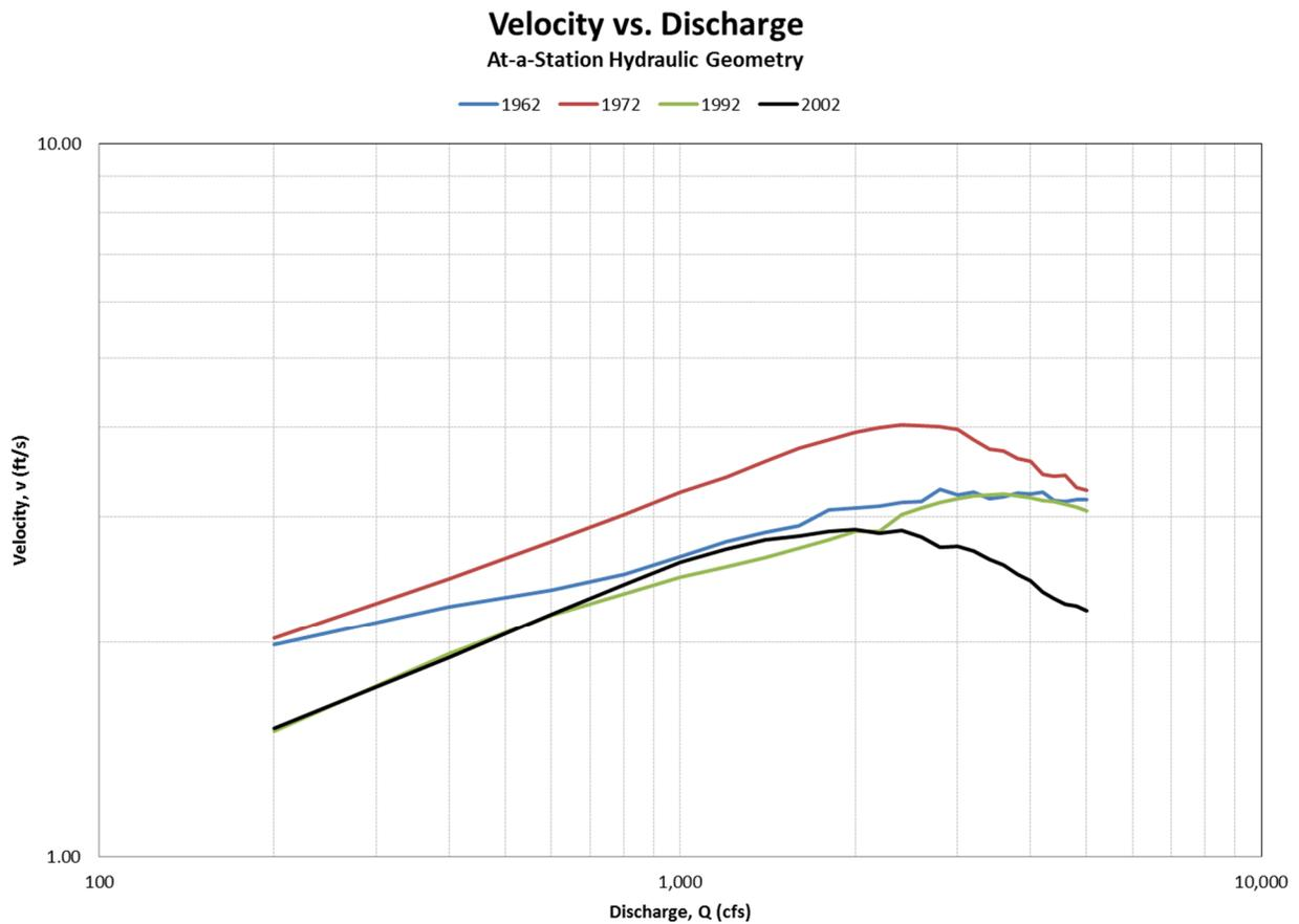
Figure 36 – Velocity vs. discharge at-a-station relationship
