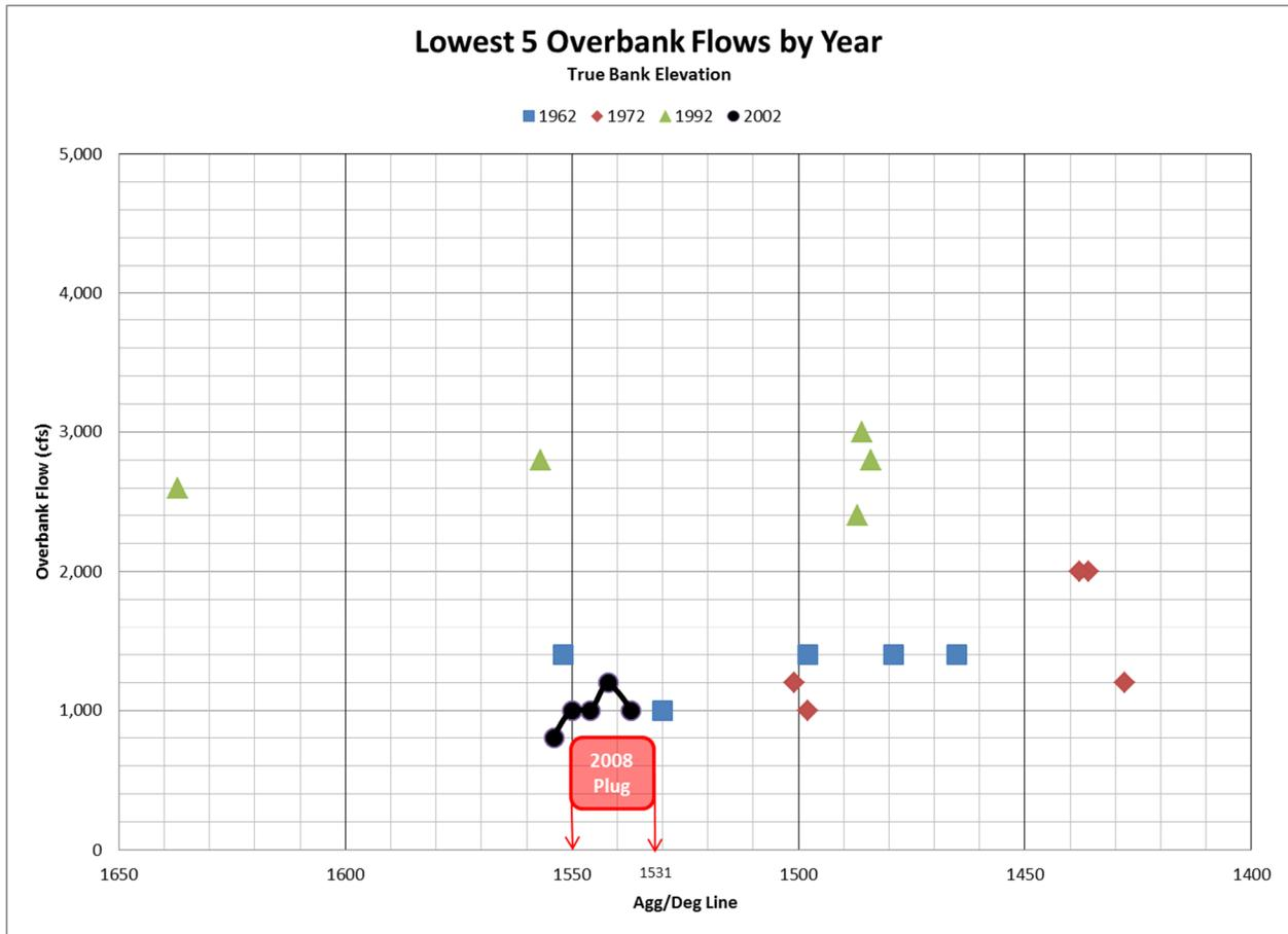
Figure 50 – Location of low overbank flows and sediment plug
