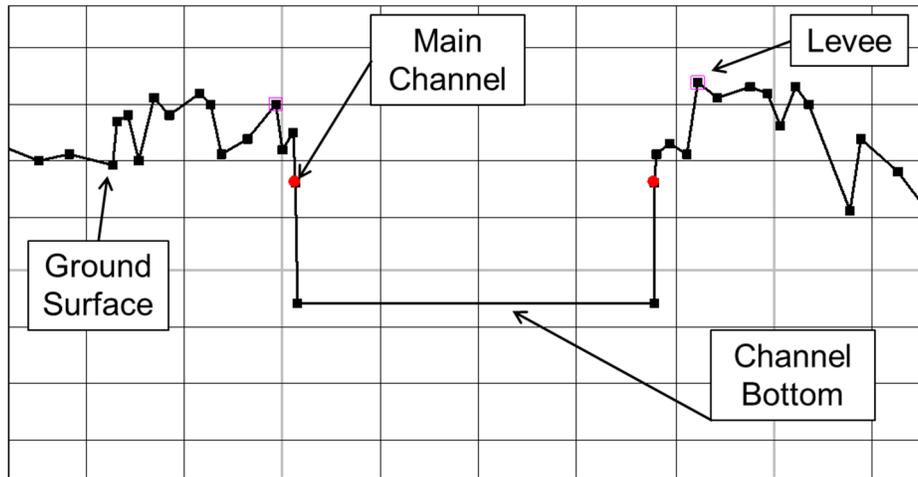
Figure 6 – Anatomy of a HEC-RAS cross-section
