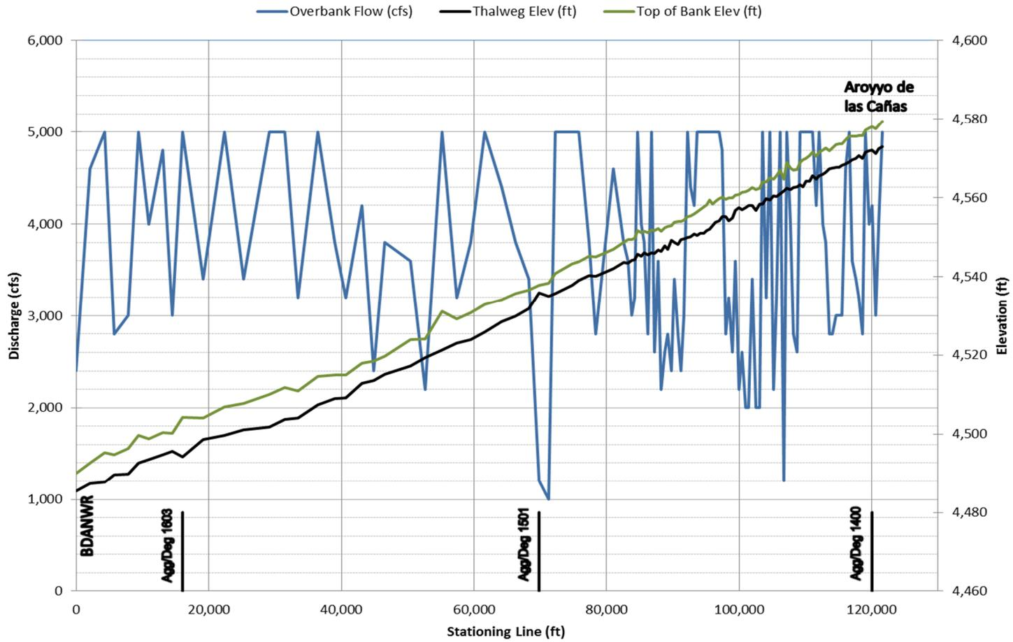
Figure 26 – 1972 Overbank flow vs. upstream distance
