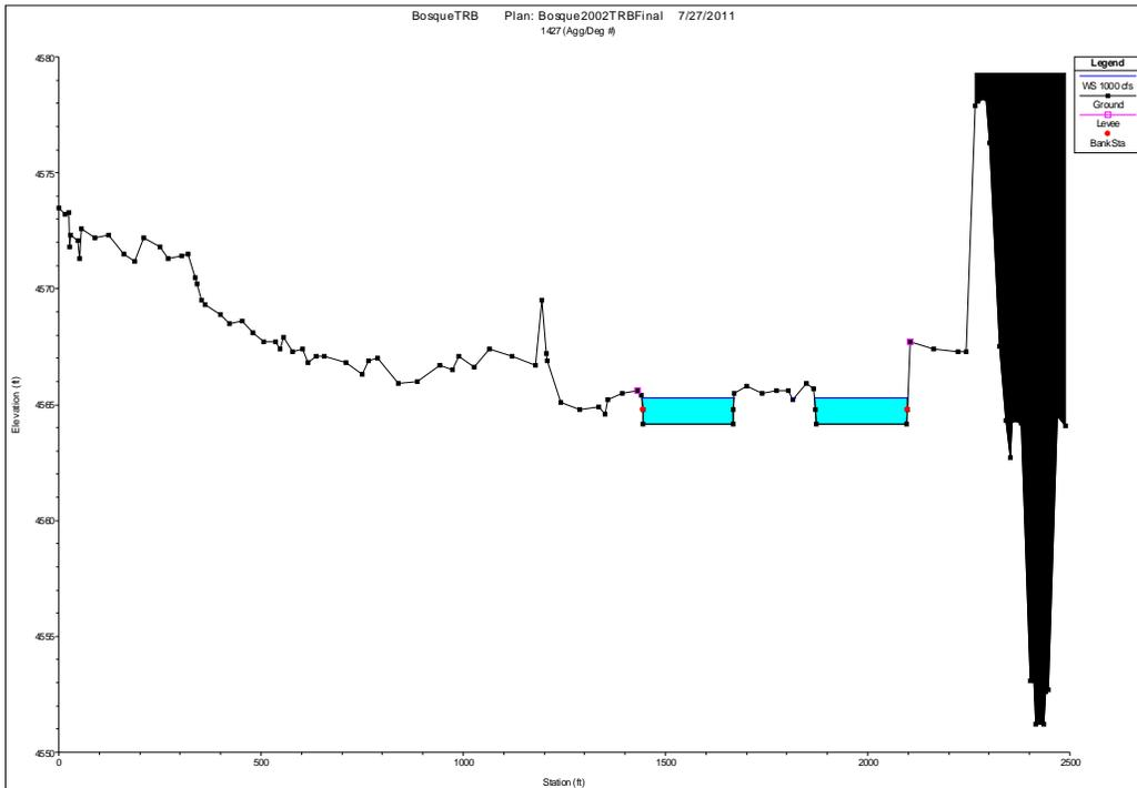
Figure 9 – 2002 Agg/Deg 1427 showing a split channel at 1,000 cfs
