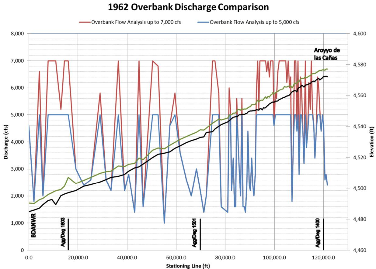
*Figure 33 – 7,000 cfs vs. 5,000 cfs overbank limits for 1962 data*
