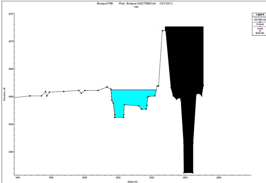
*Figure 13 – 1962 River channel at Agg/Deg 1440 adjacent to the LFCC levee (5,000 cfs)*
