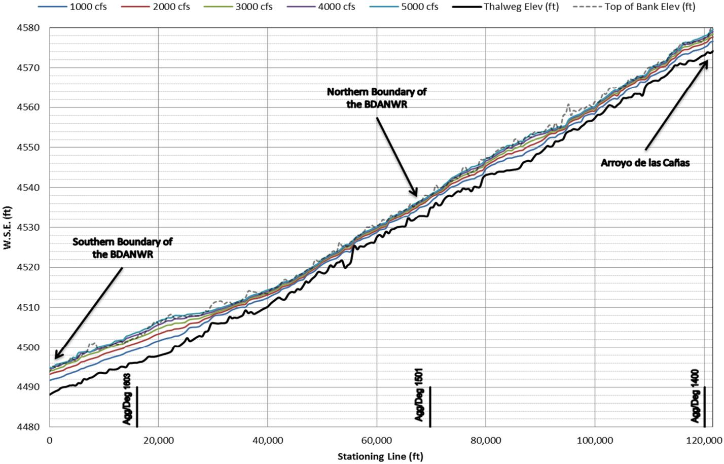
Figure 18 – 1992 Water surface profile plot vs. upstream distance
