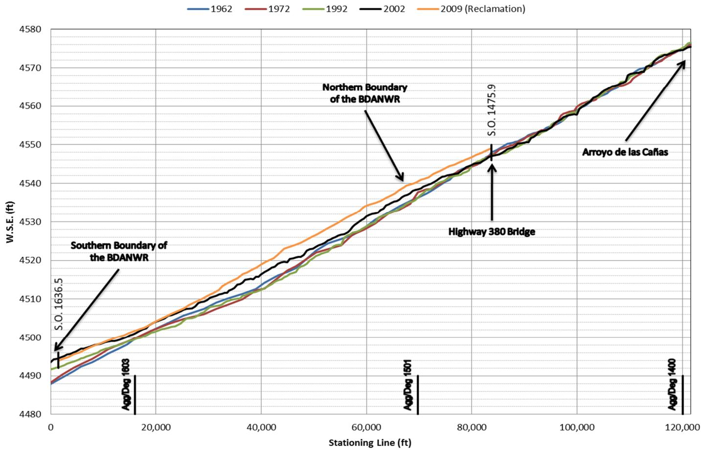
Figure 23 – Water surface profile comparison including 2009 Reclamation data
