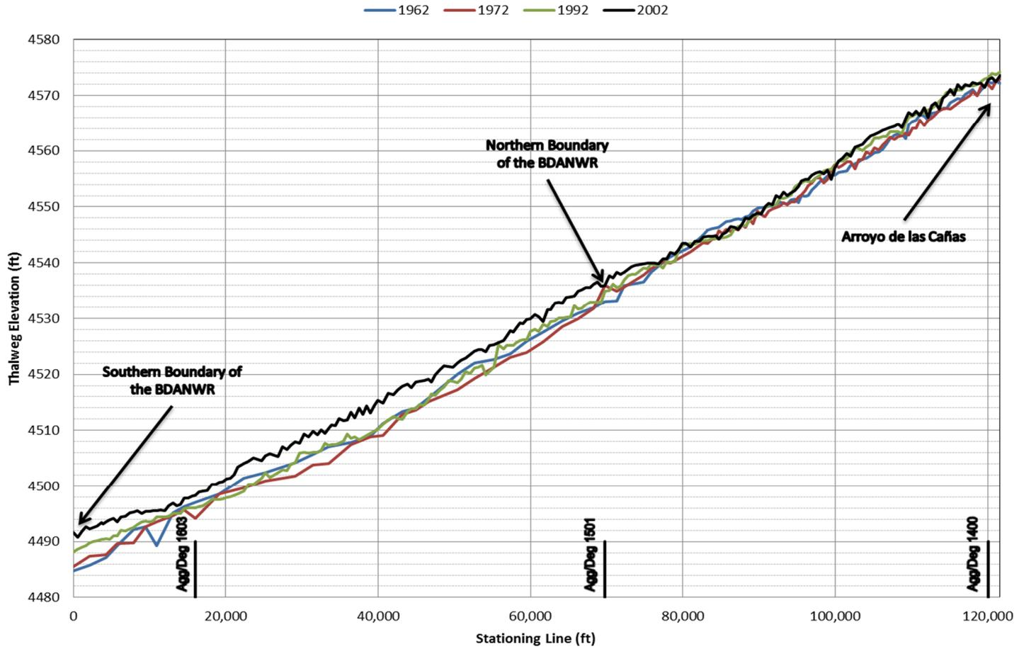
Figure 22 – Thalweg elevation profile comparison
