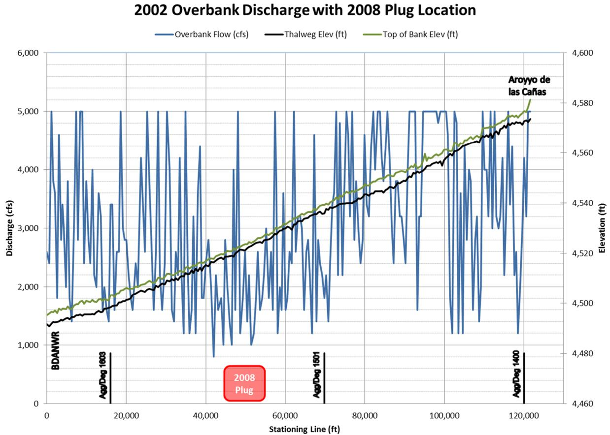
Figure 43 – Overbank flow comparison with sediment plug location
