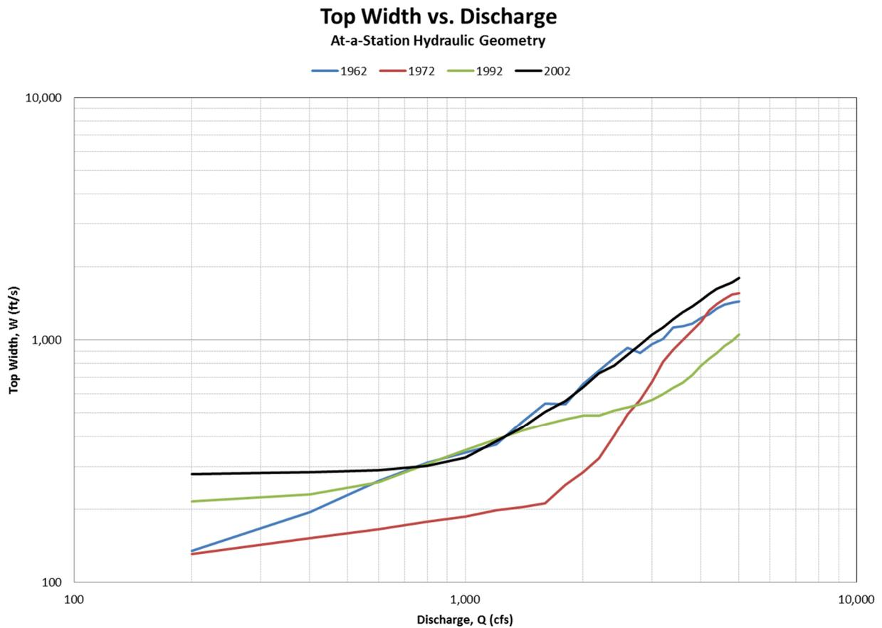
Figure 37 – Width vs. discharge at-a-station relationship
