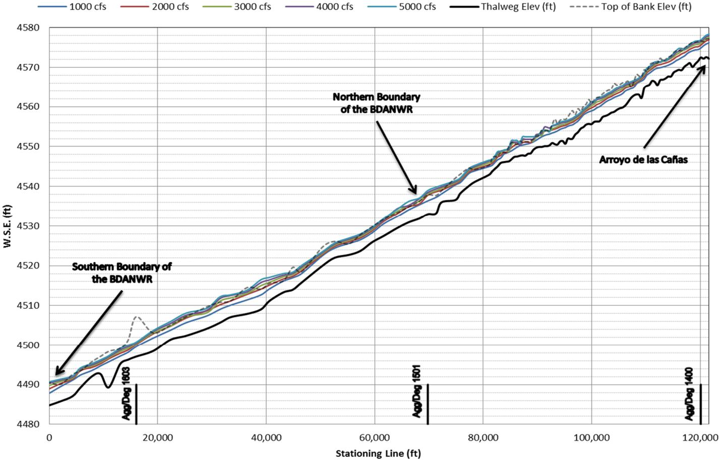
Figure 16 – 1962 Water surface profile plot vs. upstream distance
