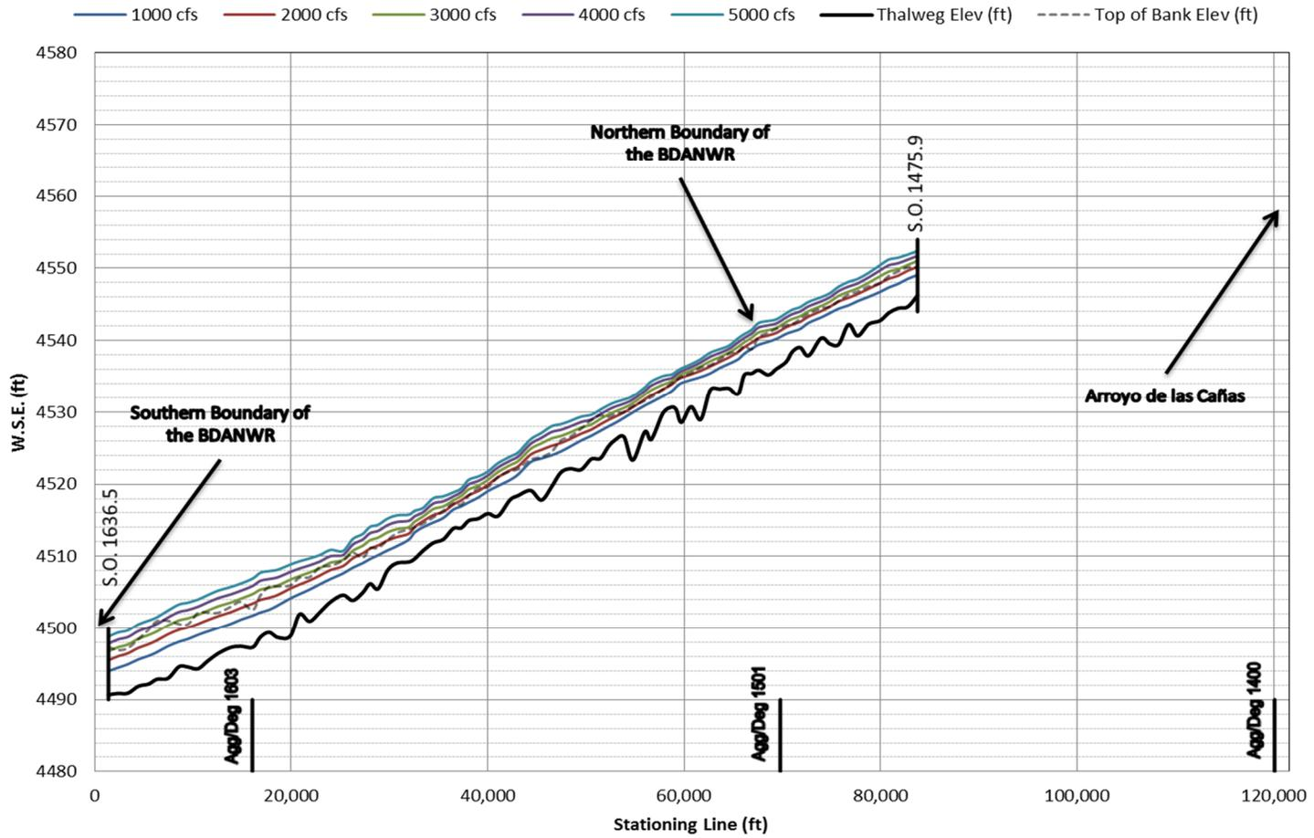
Figure 20 – 2009 Reclamation calculated water surface profile plot vs. upstream distance
