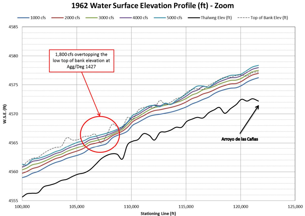
*Figure 21 – 1962 Water Surface Profile plot vs. upstream distance – Zoom*
