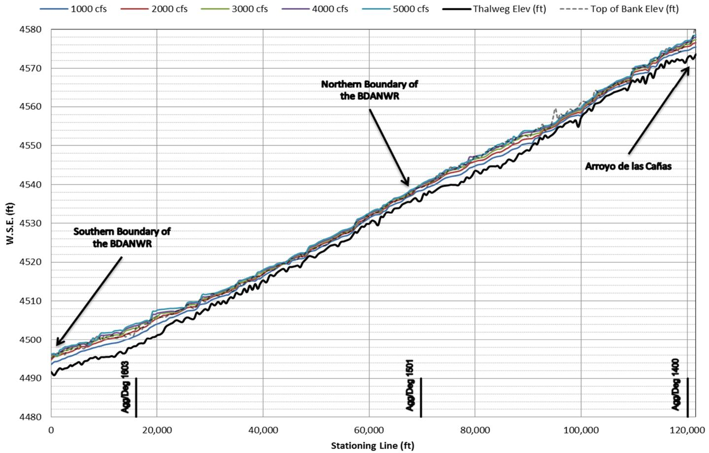
Figure 19 – 2002 Water surface profile plot vs. upstream distance
