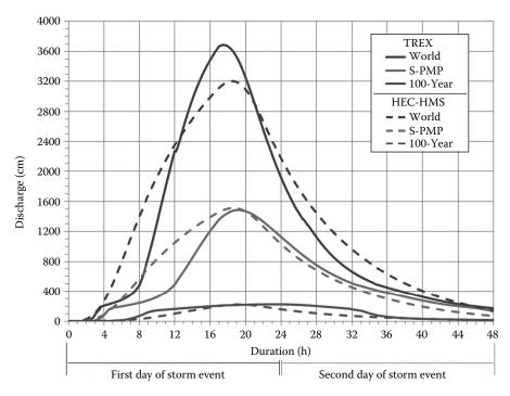
FIGURE 28.9 Flood hydrographs obtained from TREX and HEC-HMS models using the 16 h 100-year, PMP, and world's greatest storms.
