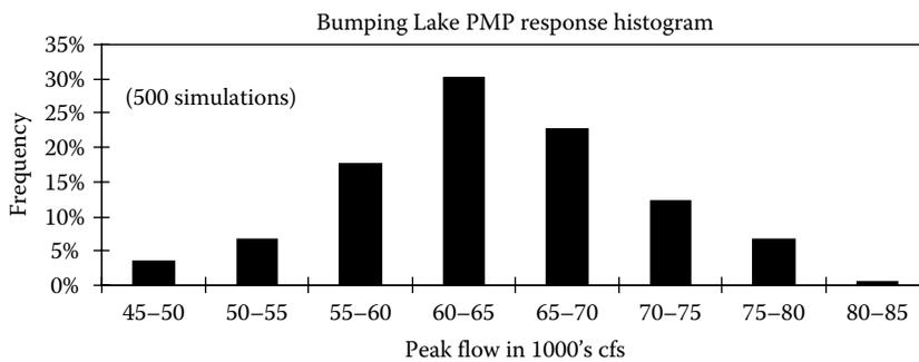
**FIGURE 28.10** Relative frequency distribution of the PMFs obtained from the 500 simulations for Bumping Lake using the PMP specified in HMR-57. (From Barker, B. et al., A Monte Carlo approach to determine the variability of PMF estimates, Final Report on Bumping Lake Dam for USBR Dam Safety Office, 1997. With permission.)
