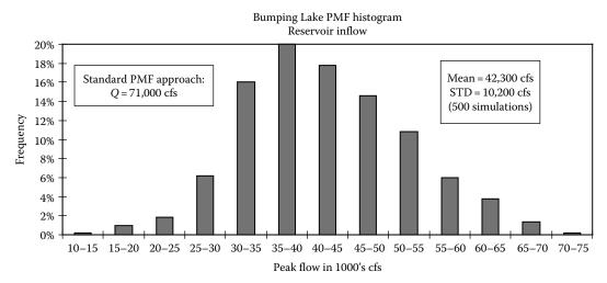
**FIGURE 28.11** Relative frequency distribution of the PMFs obtained from the 500 simulations for Bumping Lake where the 24 h precipitation was held constant at the PMP, while the other variables, including the precipitation temporal pattern, varied. (From Barker, B. et al., A Monte Carlo approach to determine the variability of PMF estimates, Final Report on Bumping Lake Dam for USBR Dam Safety Office, 1997. With permission.)
