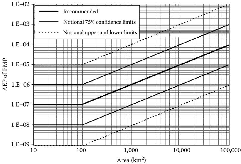
**FIGURE 28.2** Values of AEP of PMP as a function of the catchment area. (From Nathan, R.J. and Weinmann, P.E., Estimation of large to extreme floods, Book VI, *Australian Rainfall and Runoff: A Guide to Flood Estimation*, National Committee on Water Engineering, Institution of Engineers, Australia, 2001. With permission.)
