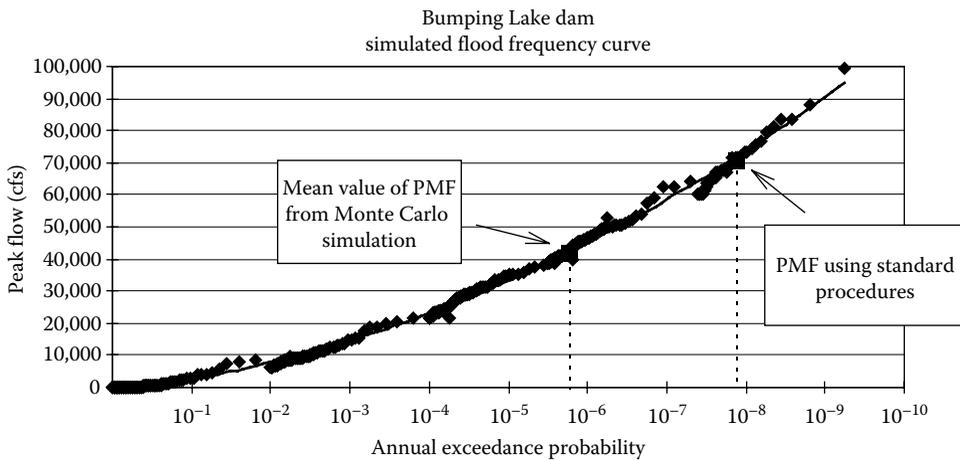
**FIGURE 28.12** Frequency distribution of the flood peaks obtained by Monte Carlo simulation considering the uncertainty of the 24 h annual maximum precipitation in addition to the uncertainty of the other driving variables to estimate the flood. (From Barker, B. et al., A Monte Carlo approach to determine the variability of PMF estimates, Final Report on Bumping Lake Dam for USBR Dam Safety Office, 1997. With permission.)
