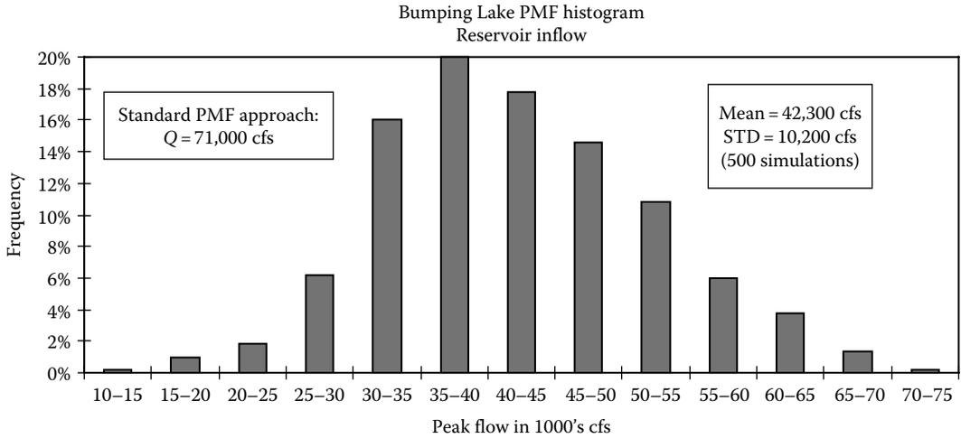
**FIGURE 28.11** Relative frequency distribution of the PMFs obtained from the 500 simulations for Bumping Lake where the 24 h precipitation was held constant at the PMP, while the other variables, including the precipitation temporal pattern, varied. (From Barker, B. et al., A Monte Carlo approach to determine the variability of PMF estimates, Final Report on Bumping Lake Dam for USBR Dam Safety Office, 1997. With permission.)
