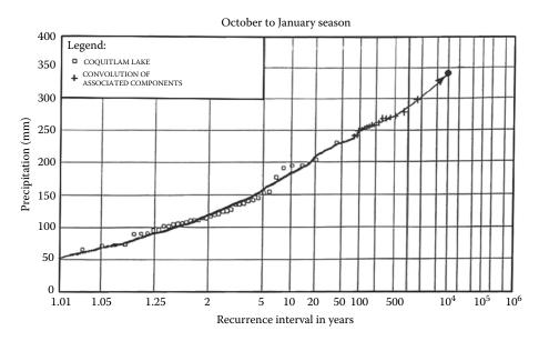
**FIGURE 28.4** Empirical frequency distribution of annual maxima of daily precipitation at Coquitlam Lake obtained from the 1600 combinations of the orographic and convergence components. (From Klemes, V. et al., *Dam Safety*, 1, 1992. With permission.)
