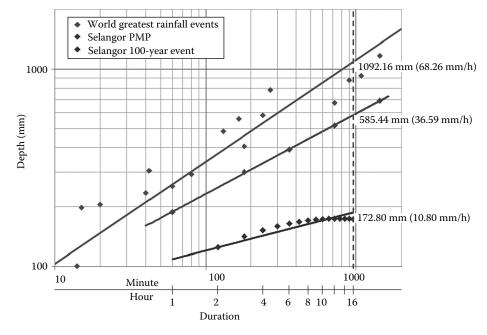
**FIGURE 28.7** PMP estimates for the state of Selangor, Malaysia, for various storm durations. For comparison, the 100-year rainfall depths and the world's greatest rainfall depths are also shown.
