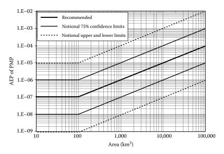
**FIGURE 28.2** Values of AEP of PMP as a function of the catchment area. (From Nathan, R.J. and Weinmann, P.E., Estimation of large to extreme floods, Book VI, *Australian Rainfall and Runoff: A Guide to Flood Estimation*, National Committee on Water Engineering, Institution of Engineers, Australia, 2001. With permission.)
