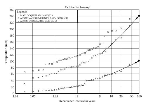
**FIGURE 28.3** Empirical frequency distribution of annual maxima of daily precipitation at Coquitlam Lake (CL, square symbol) and their orographic (x symbol) and convergence (triangular symbol) components. (From Klemes, V. et al., *Dam Safety*, 1, 1992. With permission.)
