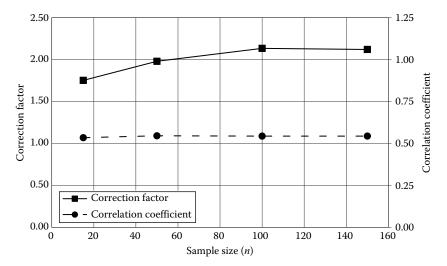
**FIGURE 28.5** Variation of the correction factor  $f_n$  and the correlation coefficient  $\rho(\overline{X}_n, S_n)$  as a function of the sample size n obtained by simulation using Gumbel random numbers (see Table 28.2). The correction factor  $f_n$  and the correlation coefficient  $\rho(\overline{X}_n, S_n)$  are used in developing  $\sigma(\hat{P})$  of (28.5).
