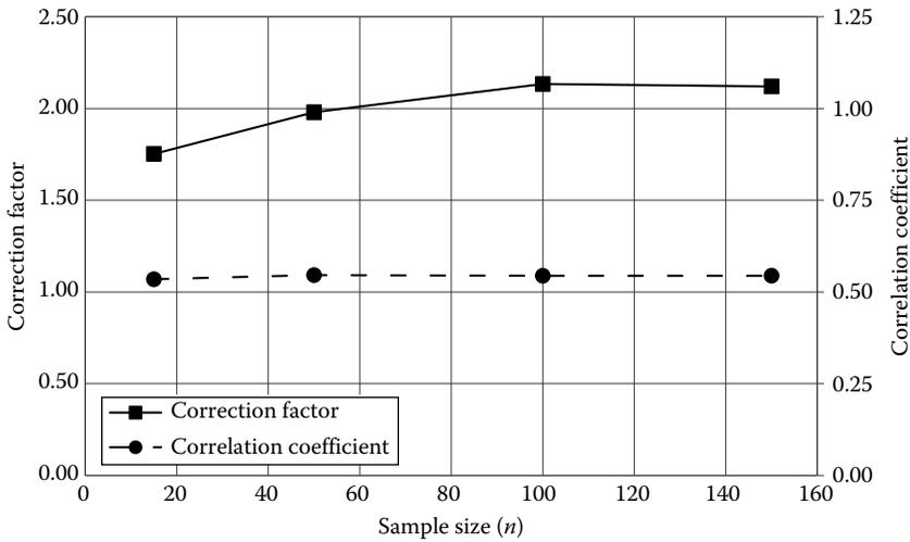
**FIGURE 28.5** Variation of the correction factor  $f_n$  and the correlation coefficient  $\rho(\bar{X}_n, S_n)$  as a function of the sample size  $n$  obtained by simulation using Gumbel random numbers (see Table 28.2). The correction factor  $f_n$  and the correlation coefficient  $\rho(\bar{X}_n, S_n)$  are used in developing  $\sigma(\hat{P})$  of (28.5).
