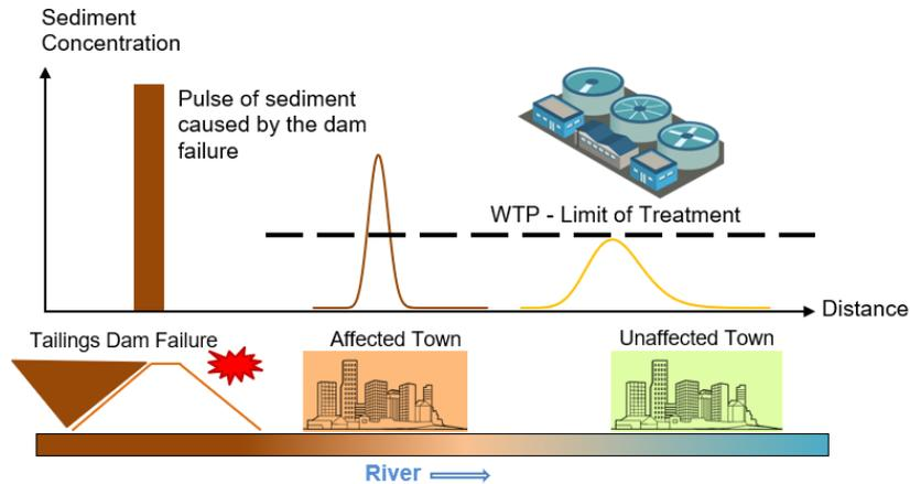
Figure 1 – Scheme of the sediment propagation after a hypothetical tailings dam failure
