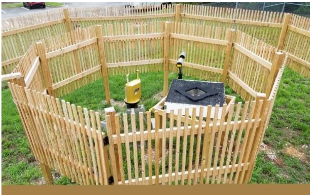
FIG. 1: (a) The MPS, 2DVD and Pluvio inside the double wind fence at the site near Greeley, Colorado (40.3273569N, 104.6093944W, 1.4 km AMSL). (b) MPS, 2DVD and Parsivel disdrometers inside the double wind fence at the Huntsville site (34.7233333N, 86.6419444W, 212 m AMSL).
