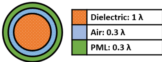
Fig. 1. Lossy dielectric sphere problem geometry. Using the QoI from [6], a posteriori EECEs were computed using higher-order adjoint solutions, as in as in [4], for all sub-problems. The double higher order finite element was used to solve each problem. These adjoint solutions were also applied to compute a QoI value and QoI gradient for each sub-problem using the methods of [6]. Note that all QoI values, QoI gradients, and element-wise error contribution estimates are complex-valued.
