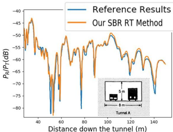
Fig. 1. Received/transmitted power along a rectangular tunnel ( $\epsilon_r = 5.5$ ,  $\sigma = 0.03$  S/m) excited with a vertically polarized half-wave dipole transmitter at 1 GHz: comparison of our SBR RT method and an SBR algorithm with IT path corrections from [7].
