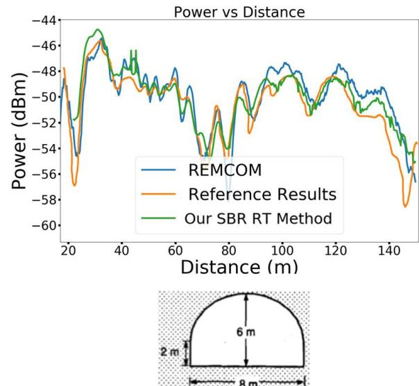
Fig. 2. Power [dBm] down the length of an arched tunnel (the tunnel cross section is shown;  $\sigma = 0.03$  S/m,  $\epsilon_r = 5.5$ ; excitation: vertically polarized dipole antenna at 1 GHz): comparison of our SBR RT method with the results by the hybrid SBR/IT RT solution [7] and by the commercial REMCOM Wireless InSite solver.
