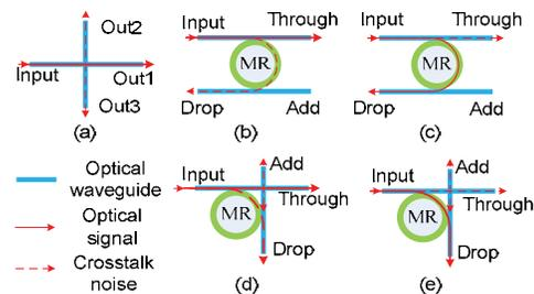
**Figure 1. Basic optical switching elements (a) Waveguide crossing (b) Parallel switching element in OFF state (c) Parallel switching element in ON state (d) Crossing switching element in OFF state (e) Crossing switching element in ON state**
