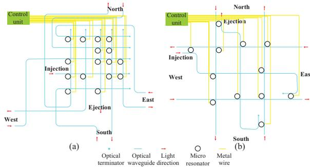
**Figure 2. 5x5 optical routers (a) The optimized optical crossbar router (b) Crux router**
