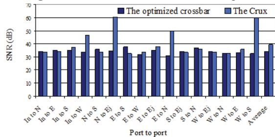
**Figure 4. Minimum SNR of each signal path**
