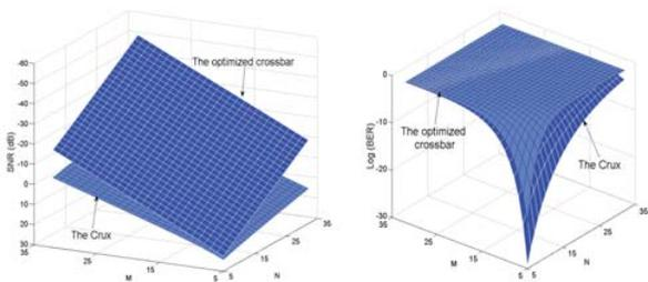
Figure 7. Minimum SNR and maximum BER in  $M \times N$  ONoCs
