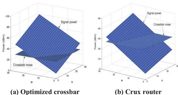
Figure 6. Signal and crosstalk noise power in the  $M \times N$  ONoCs
