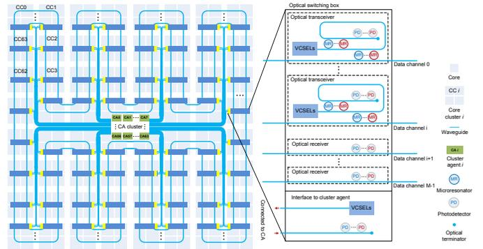
Fig. 3. The sectioned unidirectional optical ring (SUOR) structure [7].
