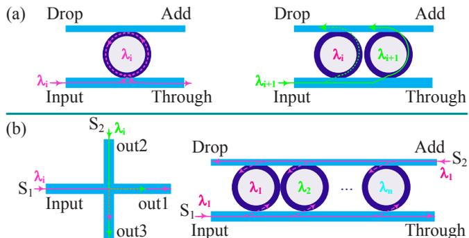
Fig. 1. Crosstalk and power loss in basic optical devices: (a) coherent crosstalk and (b) incoherent crosstalk.
