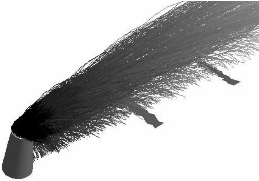
Figure 11 FLUENT predicted particle track trajectories for Rosin-Rammler particle distribution at source (Case A-1, d_{\text{mean}} = 0.09\text{mm} , n = 0.65 ).
