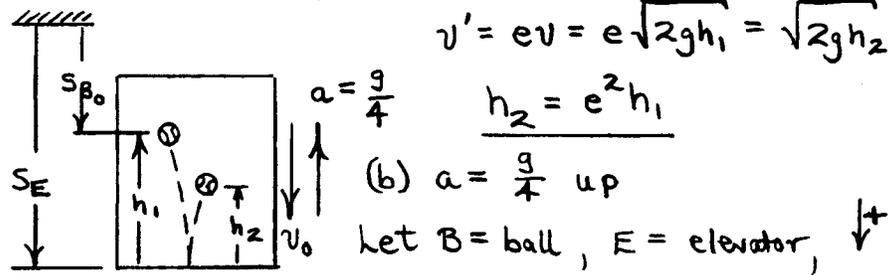
At impact,  $s_B = s_E$ :  $s_{B_0} + v_{B_0}t + \frac{1}{2}gt^2 = s_{E_0} + v_{E_0}t - \frac{1}{2}\frac{g}{4}t^2$
