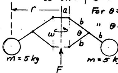
For  $\theta = 90^\circ$ ,  $r_0 = 0.1 + 2(0.3) \cos 45^\circ = 0.524 \text{ m}$
