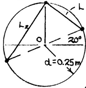
$$\begin{cases} L_1 = 2d \sin(90^\circ - 20^\circ)/2 = 0.287 \text{ m} \\ \delta_1 = 0.25\sqrt{2} - L_1 = 0.0668 \text{ m} \\ L_2 = 2d \sin\left(\frac{90^\circ + 20^\circ}{2}\right) = 0.410 \text{ m} \\ \delta_2 = L_2 - 0.25\sqrt{2} = 0.0560 \text{ m} \end{cases}$$
