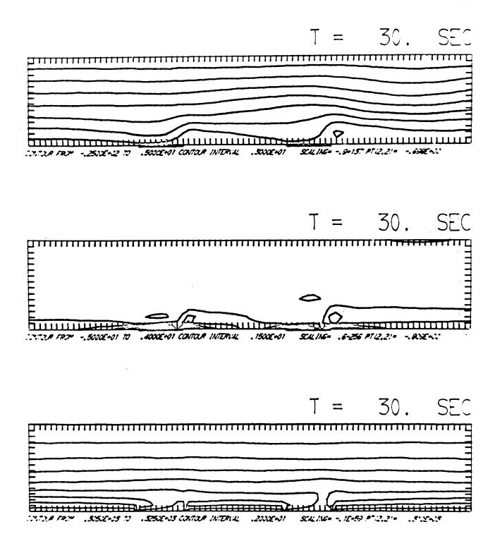
Fig. 3. Numerically obtained contour lines of stream function, vorticity, and temperature at t = 30 sec.
