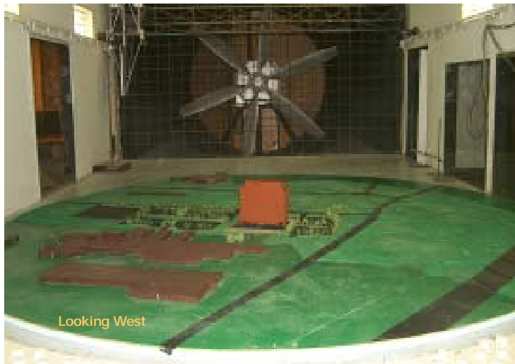
Fig. 2. Model (1:240) scale in Environmental Wind Tunnel, WEFL, Colorado State
