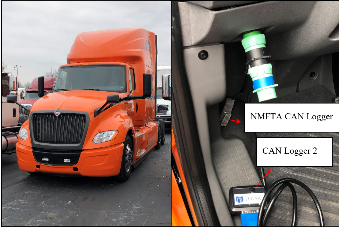
Figure 4-5. Data collection on a 2019 International truck at the Summit Truck Group dealership in Tulsa
