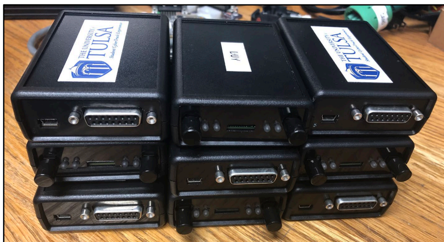
Figure 2-39. CAN monitoring devices in production
