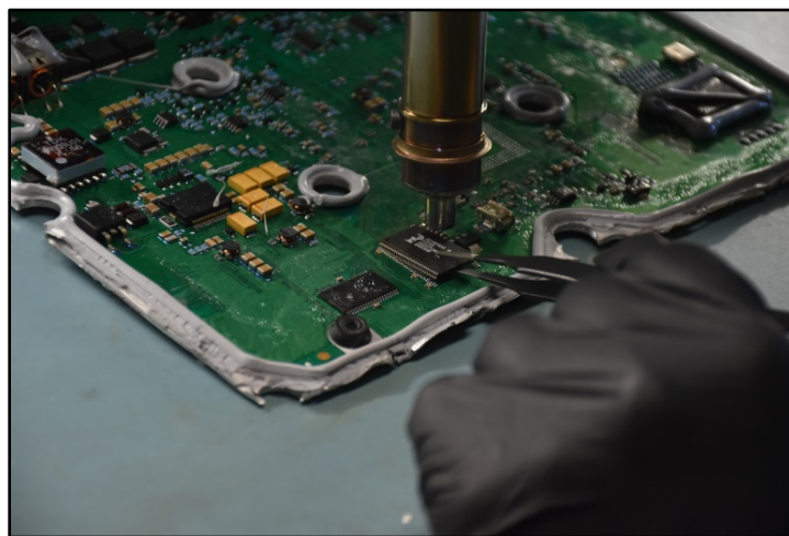
Figure 5-7. Removing flash memory from an engine control module using a hot-air rework station
