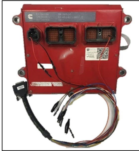
Figure 5-12. : Power cable with key switch shown connected to a Cummins CM870 ECM
