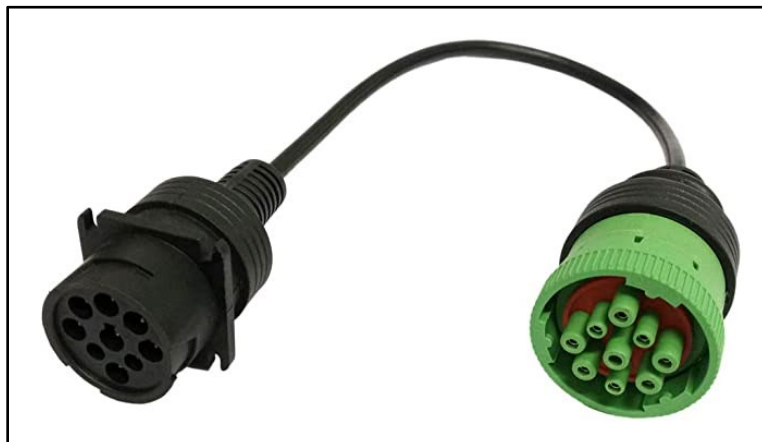
Figure 2-2. SAE J1939 type-1 (black) to type-2 (green) adapter cable [12]
