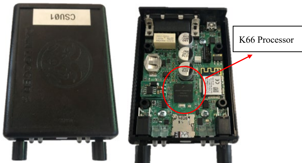
Figure 2-9. This photograph of the CAN Logger 3, Rev 3e shows the single board solution using the K66 processor
