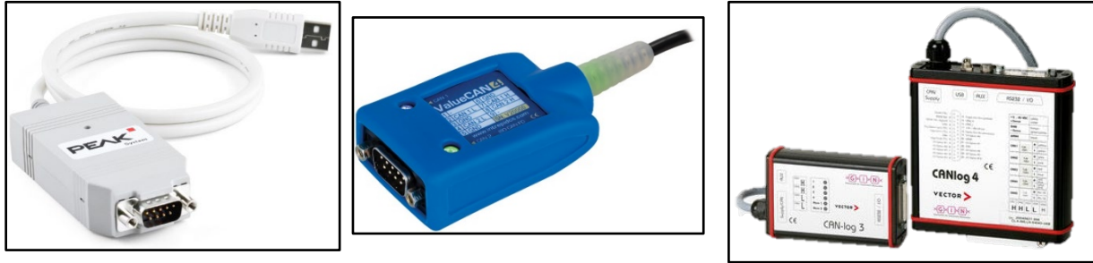
Figure 2-3. CAN analyzing tools: PEAK PCAN-USB [13] (left), Intrepid ValueCAN [14] (middle), and Vector CANlog [15] (right)
