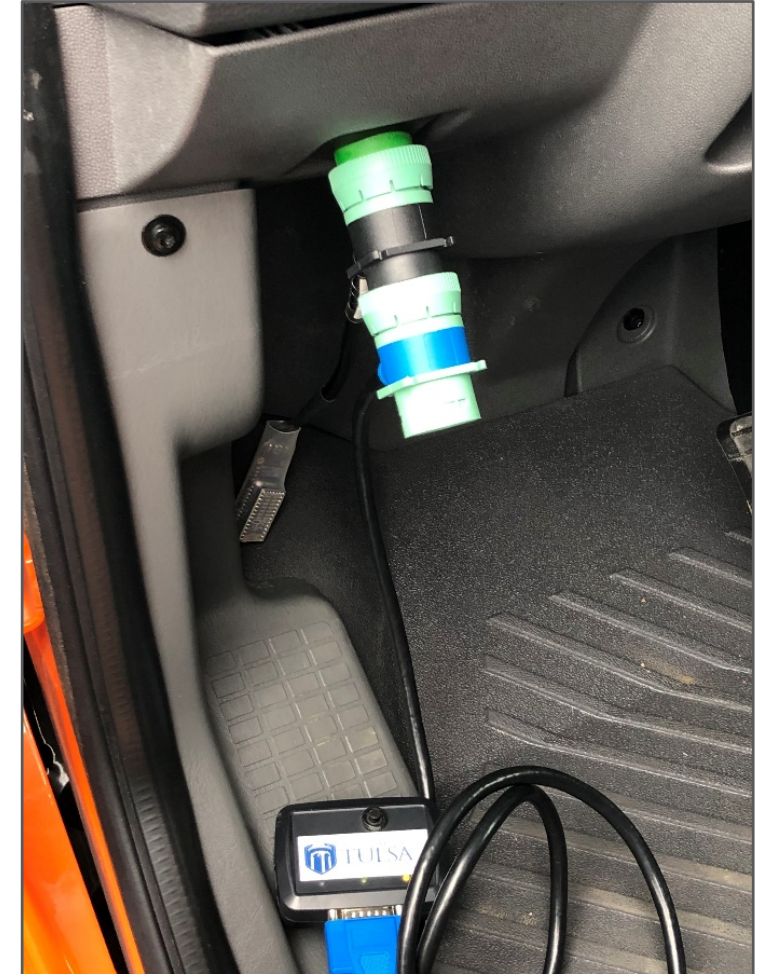
A diagnostic port in a heavy truck
