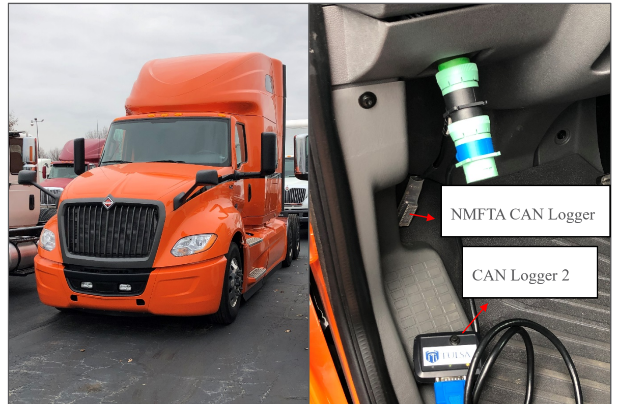
Data collection on a 2019 International truck at the Summit Truck Group dealership in Tulsa
