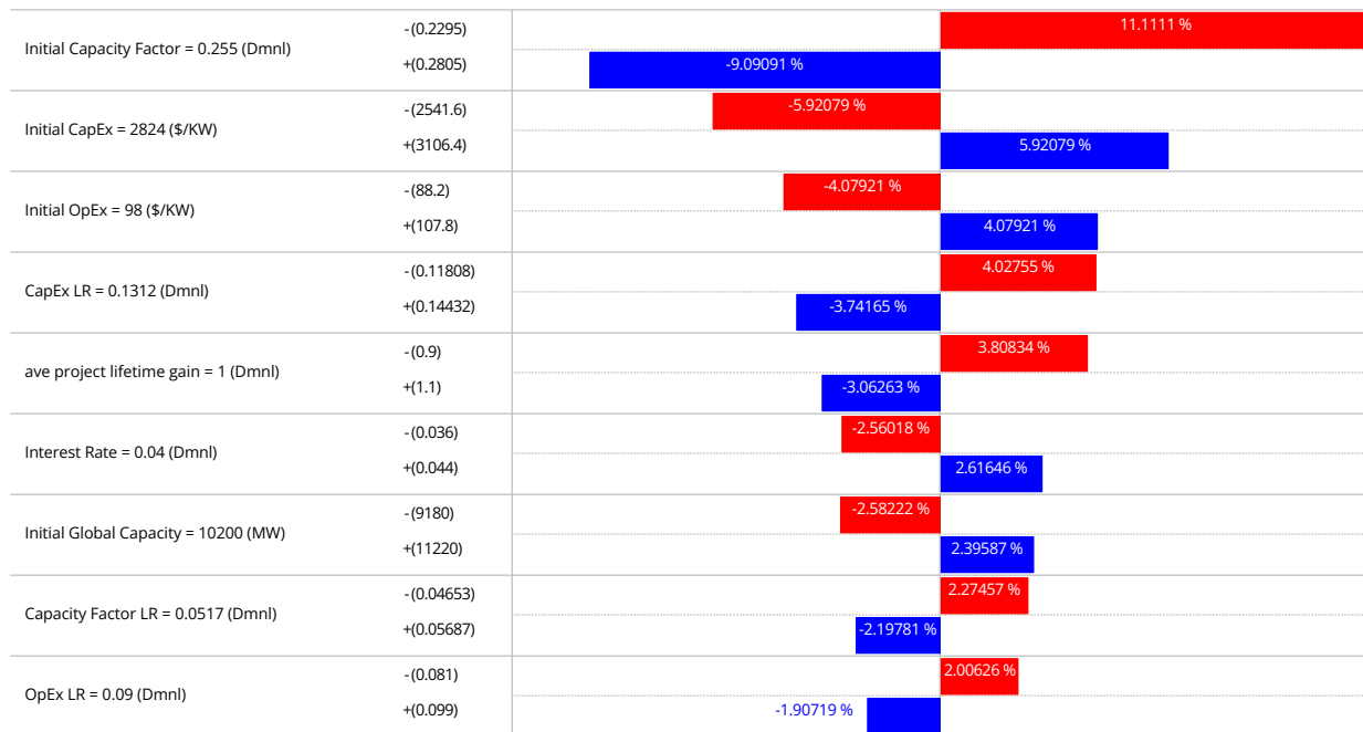
Figure 4.14: Sensitivity of LCOE to modeled variables
