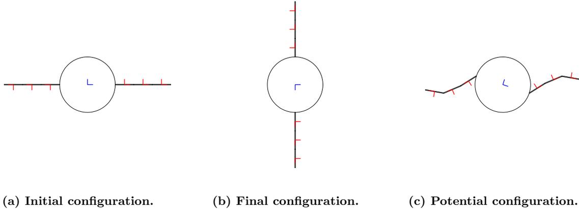
Figure 7: Various configurations of the satellite reorientation problem.
