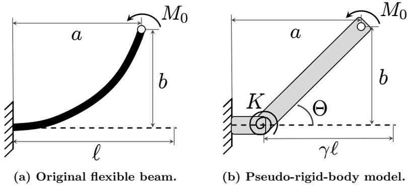
**Figure 3: Pseudo-rigid-body model of a cantilever beam with an applied moment at the free end.**
