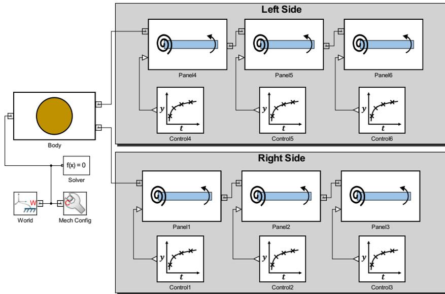
(a) Complete SimMechanics<sup>®</sup> model with 3 divisions per solar array.
