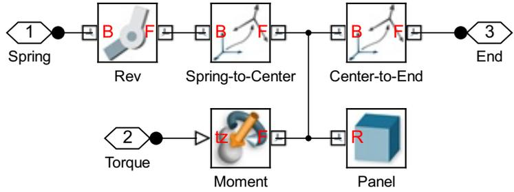
(c) Solar array subsystem.
